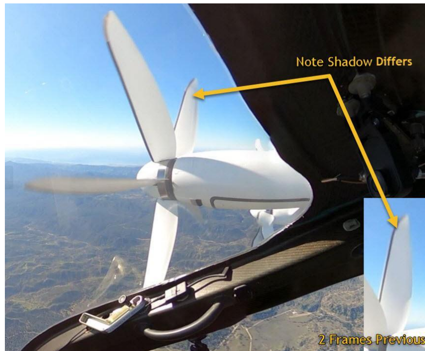
Figure 5. Time 09:58:11.373 PST. Blade shadow differences are illustrated.
