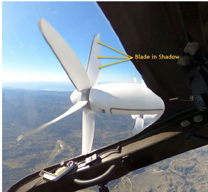
Figure 3. Time 09:58:11.373 PST. Blade shown at a nominal blade angle for the given conditions.
