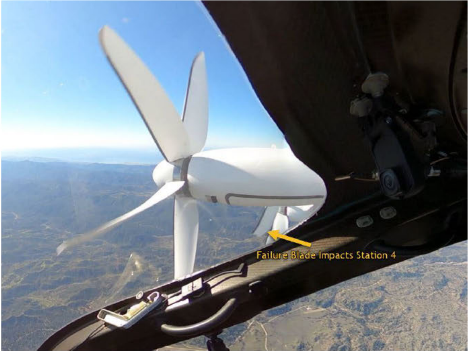
Figure 8. Time 09:58:11.473 PST. The frame shows the failure blade contacting station 4.
