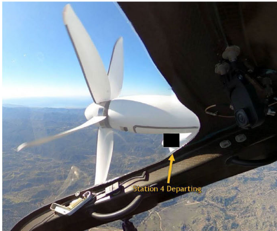
Figure 9. Time 09:58:11.704 PST. The frame shows station 4 departing from its nominal position.
