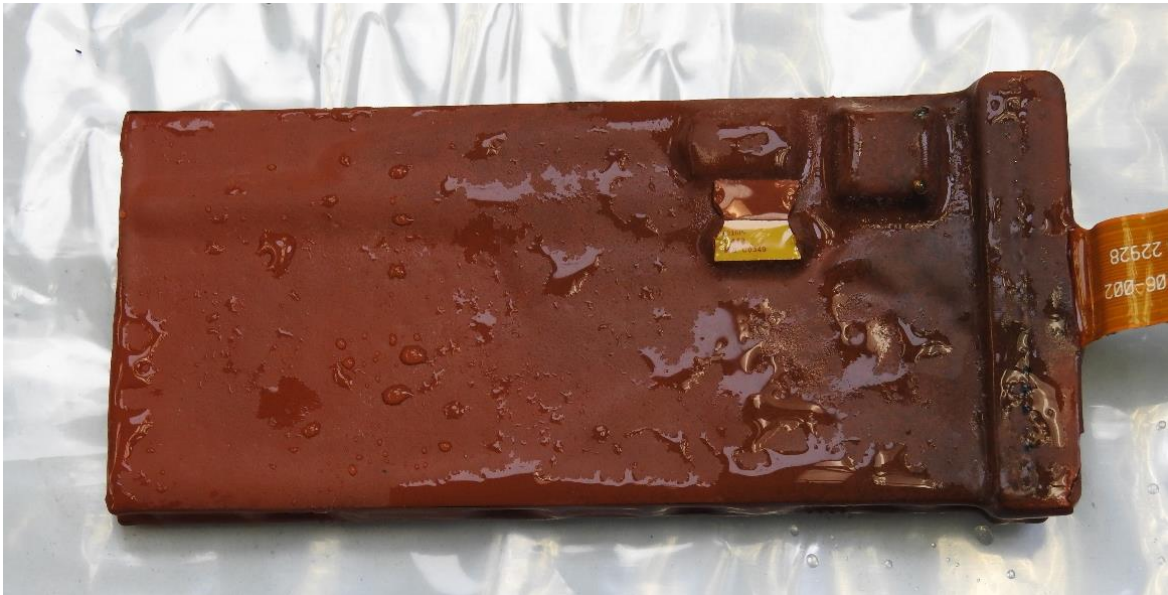
Figure 2. The memory board, recovered from within the Crash Survivable Memory Unit, still encased in RTV coating.
