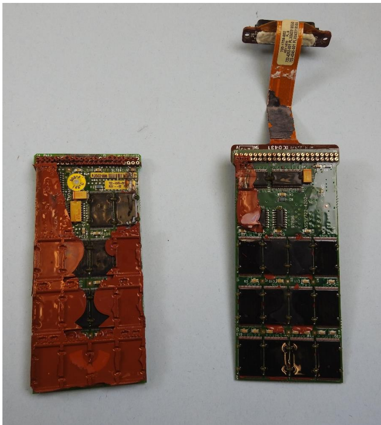
Figure 3. The memory boards with the RTV coating partially removed.
