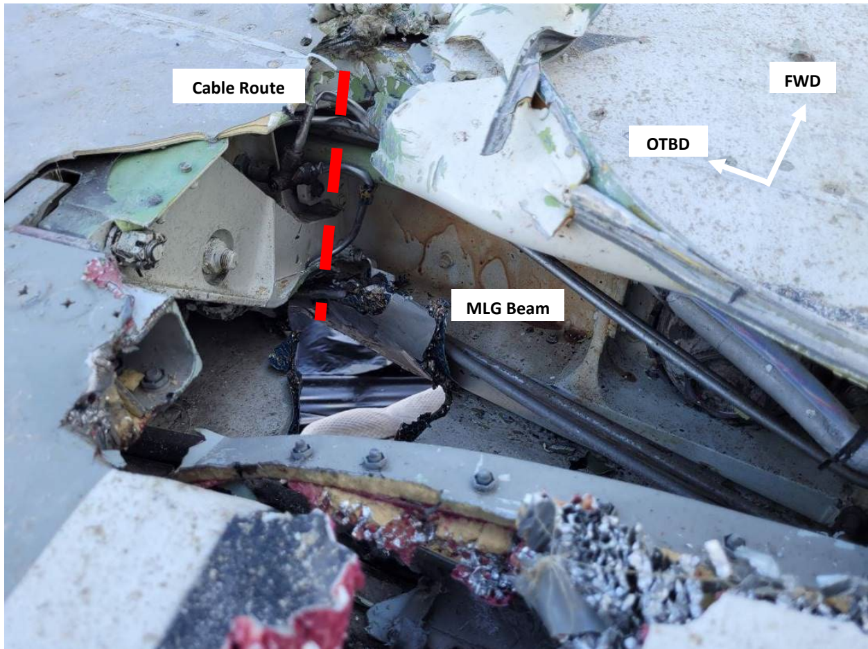
Figure 71. Left wing trailing edge damage close-up of MLG Beam (Boeing photo)
