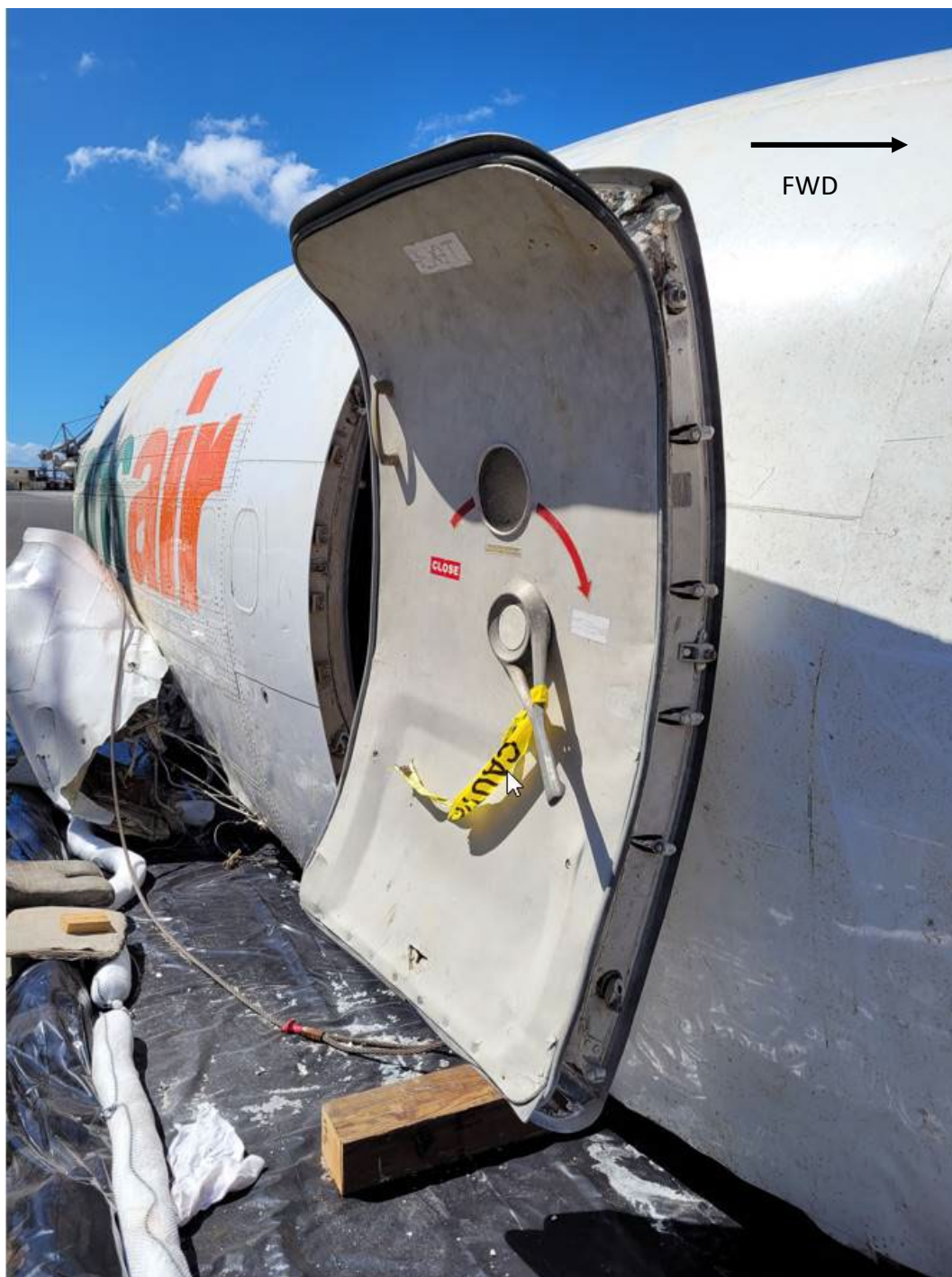
Figure 34. Right Forward Entry door, looking aft (Boeing photo)
