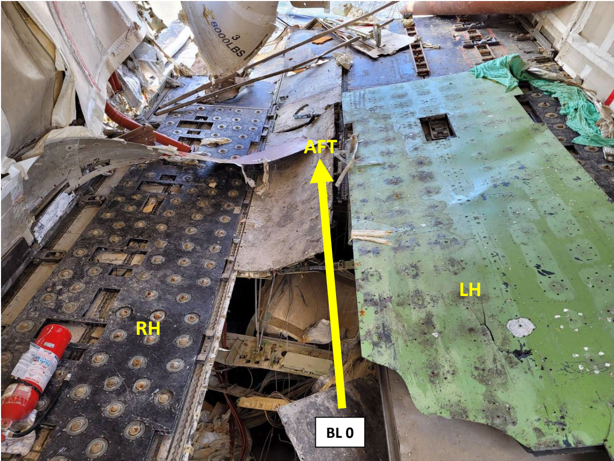
Figure 22. Main Deck Floor structure damage, looking aft (Boeing photo)
