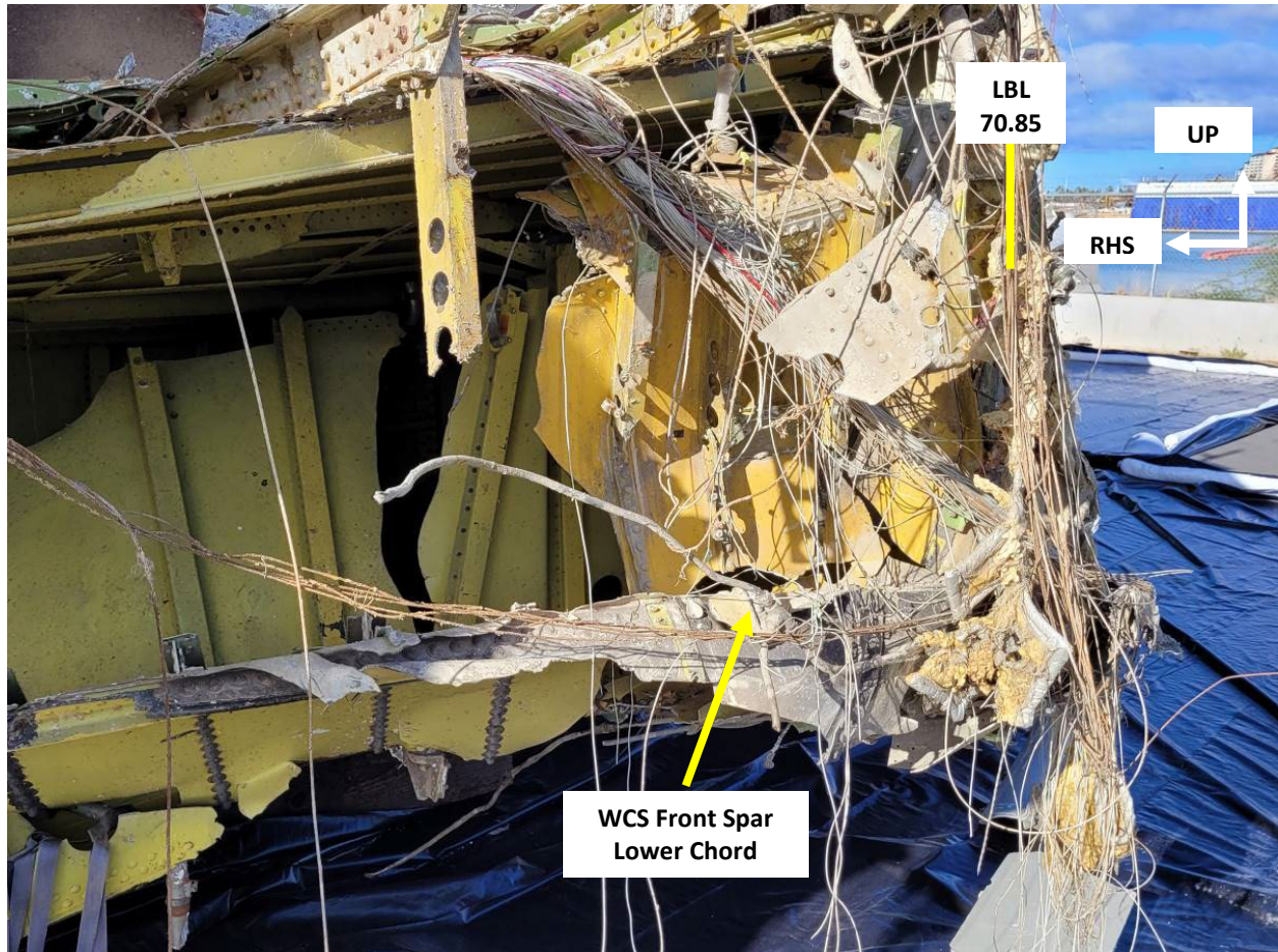
Figure 48. Left WCS Front Spar Lower Chord damage (Boeing photo)
