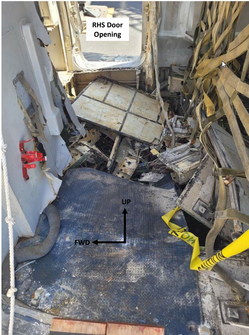
Figure 23. Floor structure damage behind the cockpit (Boeing photo)
