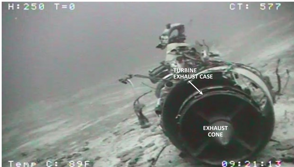
Figure 4 No. 2 engine, rear view
