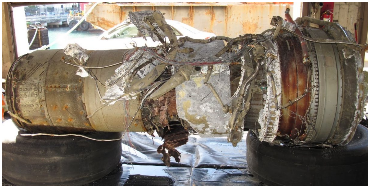
Figure 8 No. 1 engine as recovered, right side view
