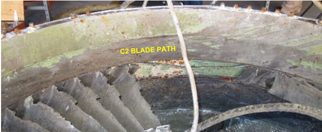
Figure 30 No. 2 engine C1 stator TE clash and C2 blade path scoring
