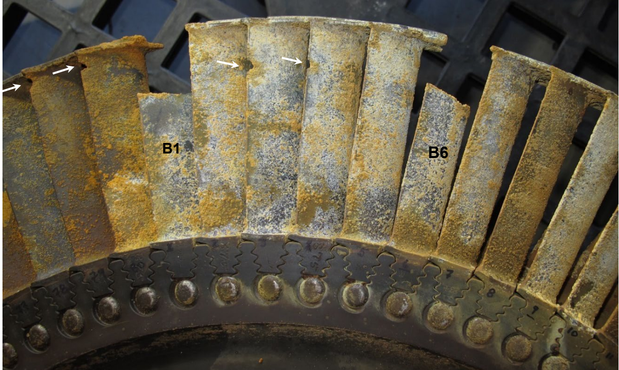
Figure 37 No. 2 engine T1 showing the two fractured blades. TE impact damage is indicated by arrows
