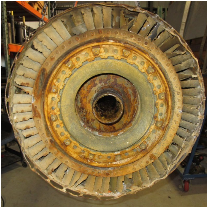
Figure 18 No. 1 engine high compressor front view showing C7 damage
