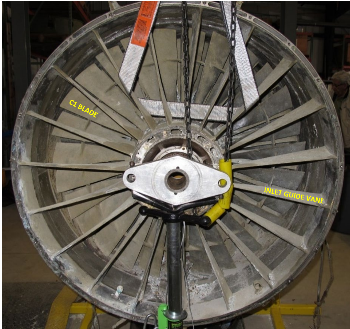
Figure 10 No. 1 engine, inlet view showing IGVs and C1
