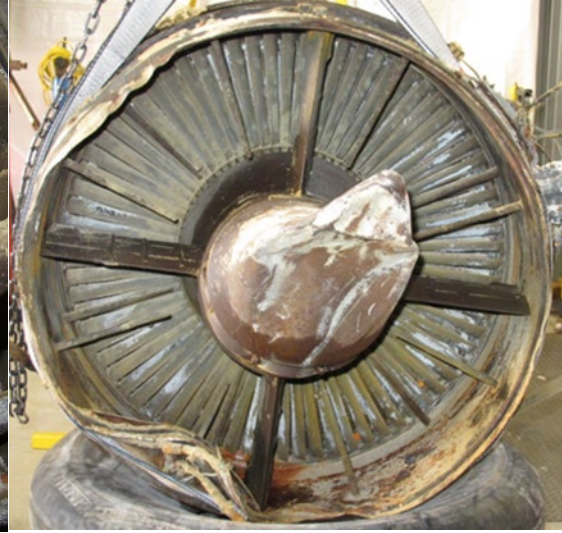
Figure 26 Aft view of No. 1 engine showing T4, and Tt7 and Pt7 probes
