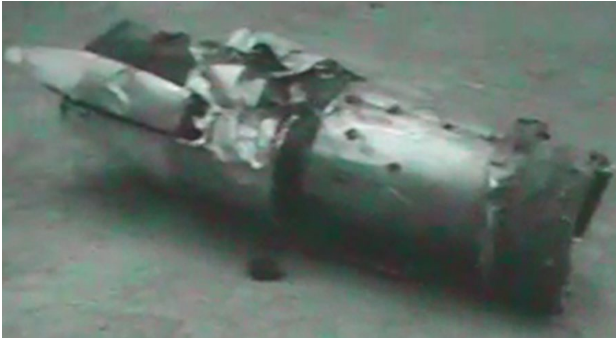
Figure 5. Unactuated No. 2 engine thrust reverser
