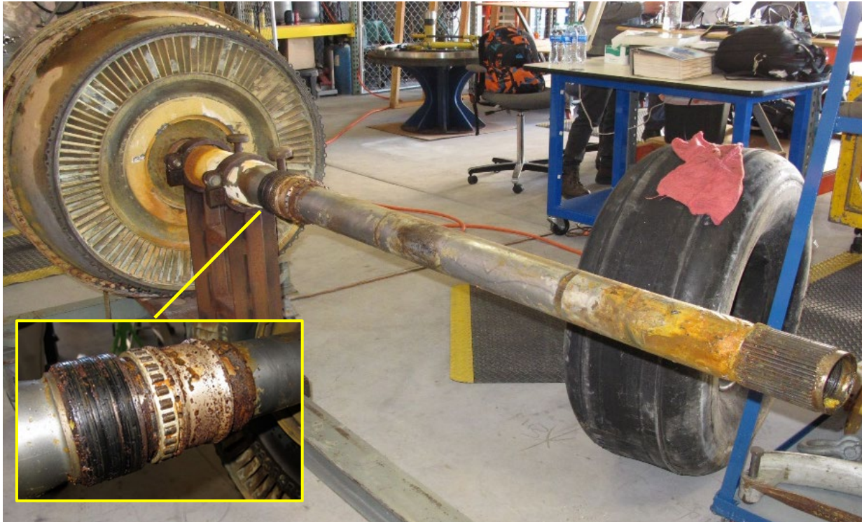
Figure 24 No. 1 engine low turbine and shaft and closeup view of No. 4 ½ interstage bearing roller elements and rotating seal components
