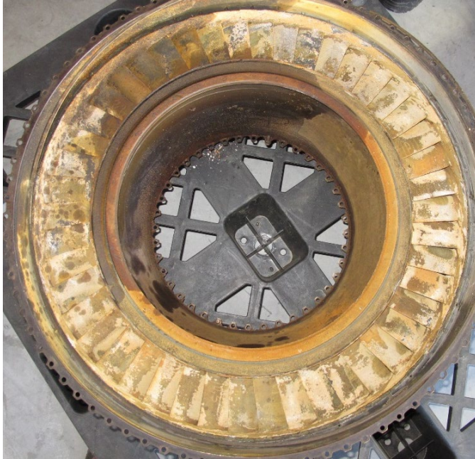
Figure 35 No. 2 engine NGV in good condition
