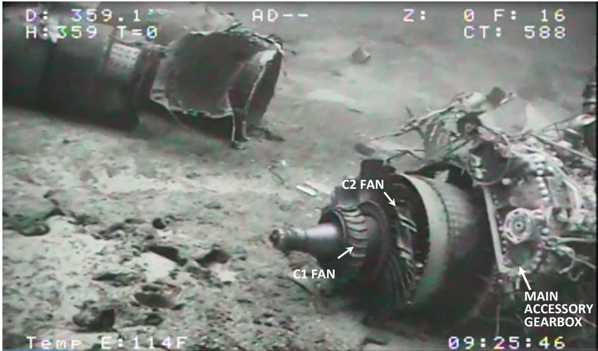
Figure 3 No. 2 engine, inverted, showing exposed fan and MGB
