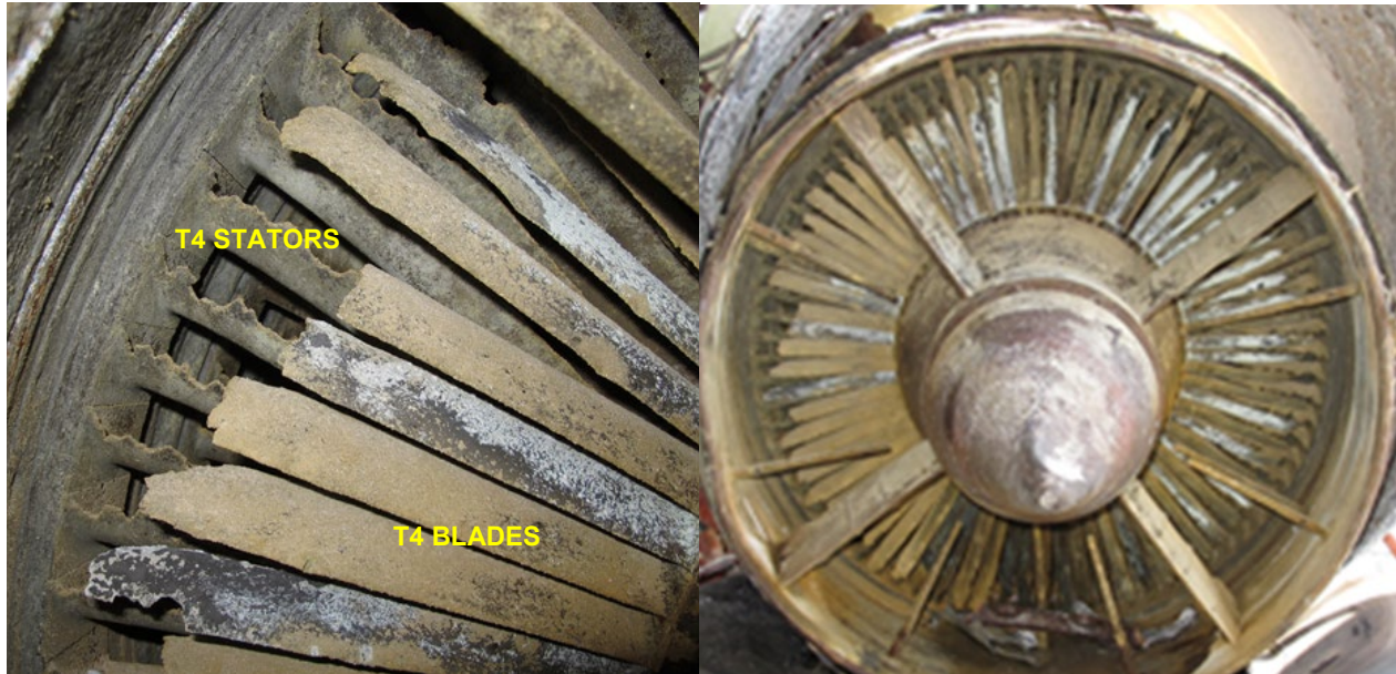
Figure 42 View through the No. 2 engine TEC showing T4 vane TE breakout damage and T4 blade outer span fractures
