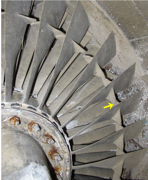
Figure 11 No. 1 engine showing shingled C1 shrouds
