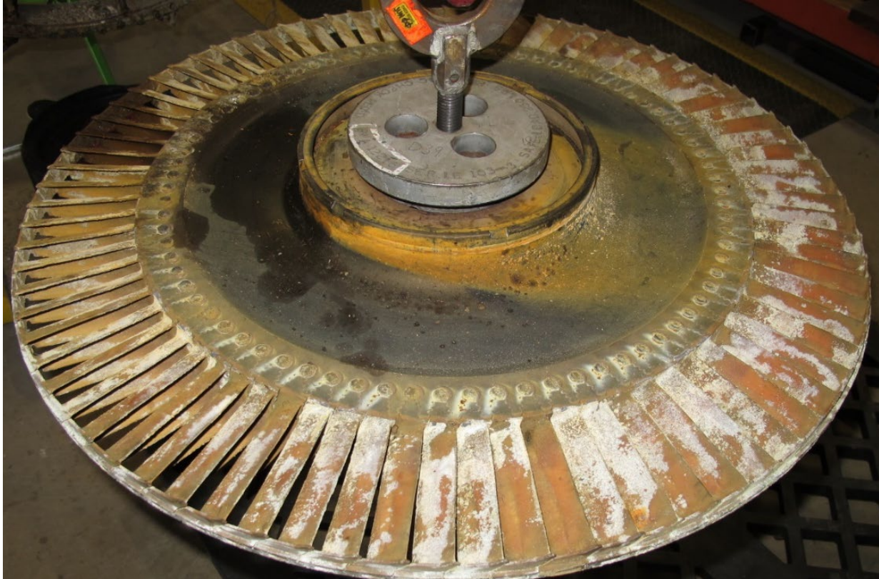
Figure 23 Aft face of the No. 1 engine T1 disk assembly showing intact airfoils and tip shrouds
