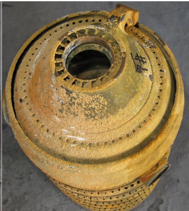
Figure 21 Visible combustor dome surface showing absence of metallization
