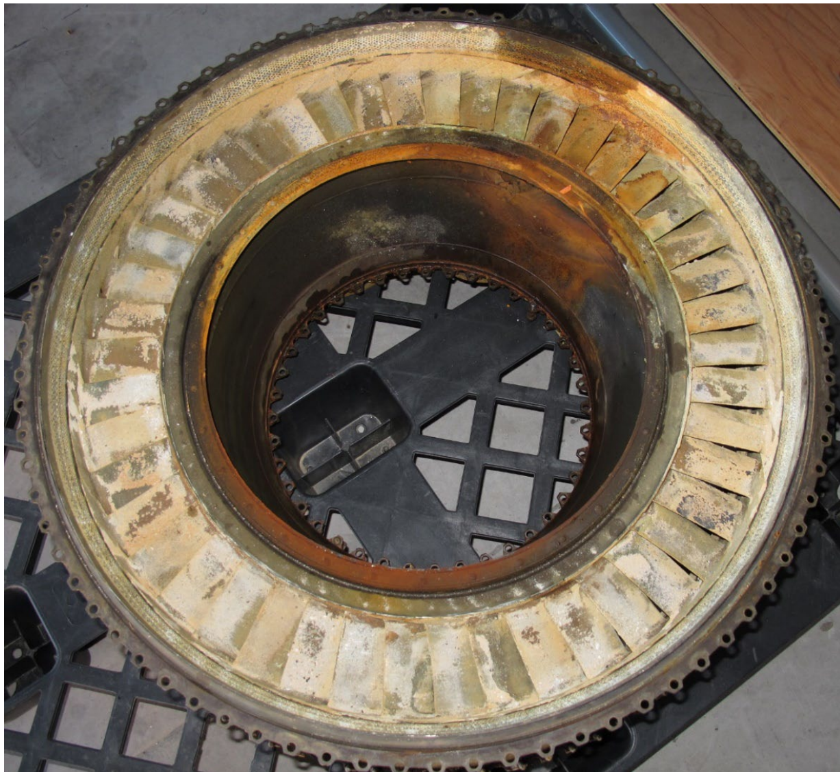
Figure 22 No. 1 engine T1 nozzle aft face, showing typical in-service T1 vane condition
