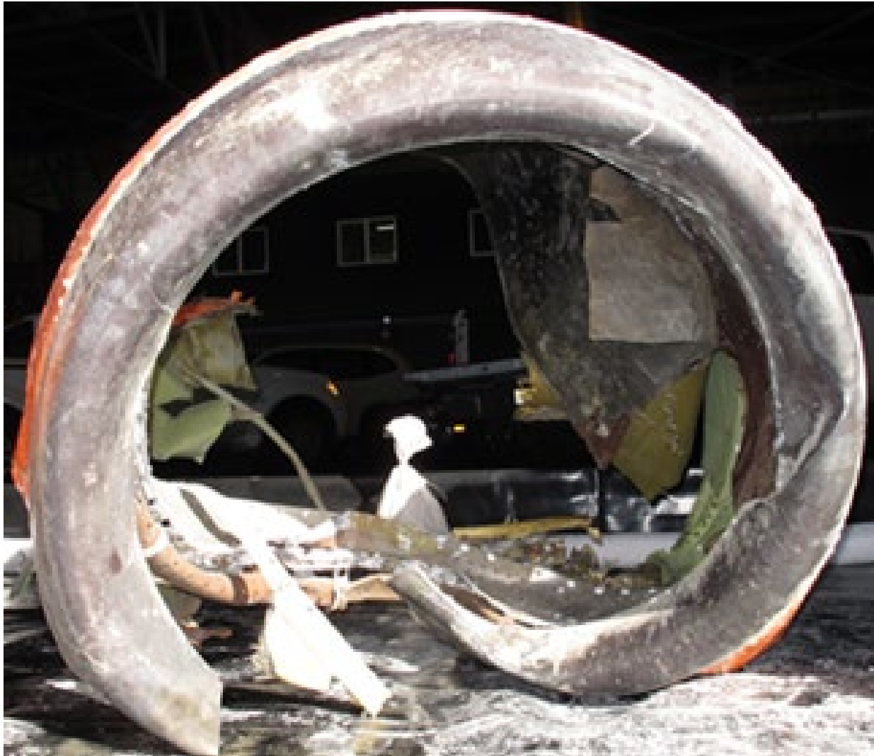
Figure 7 No. 2 nose cowl, front view
