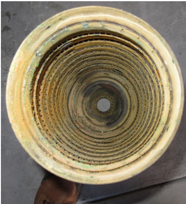
Figure 20 No. 1 engine exemplar combustion chamber showing no thermal distress
