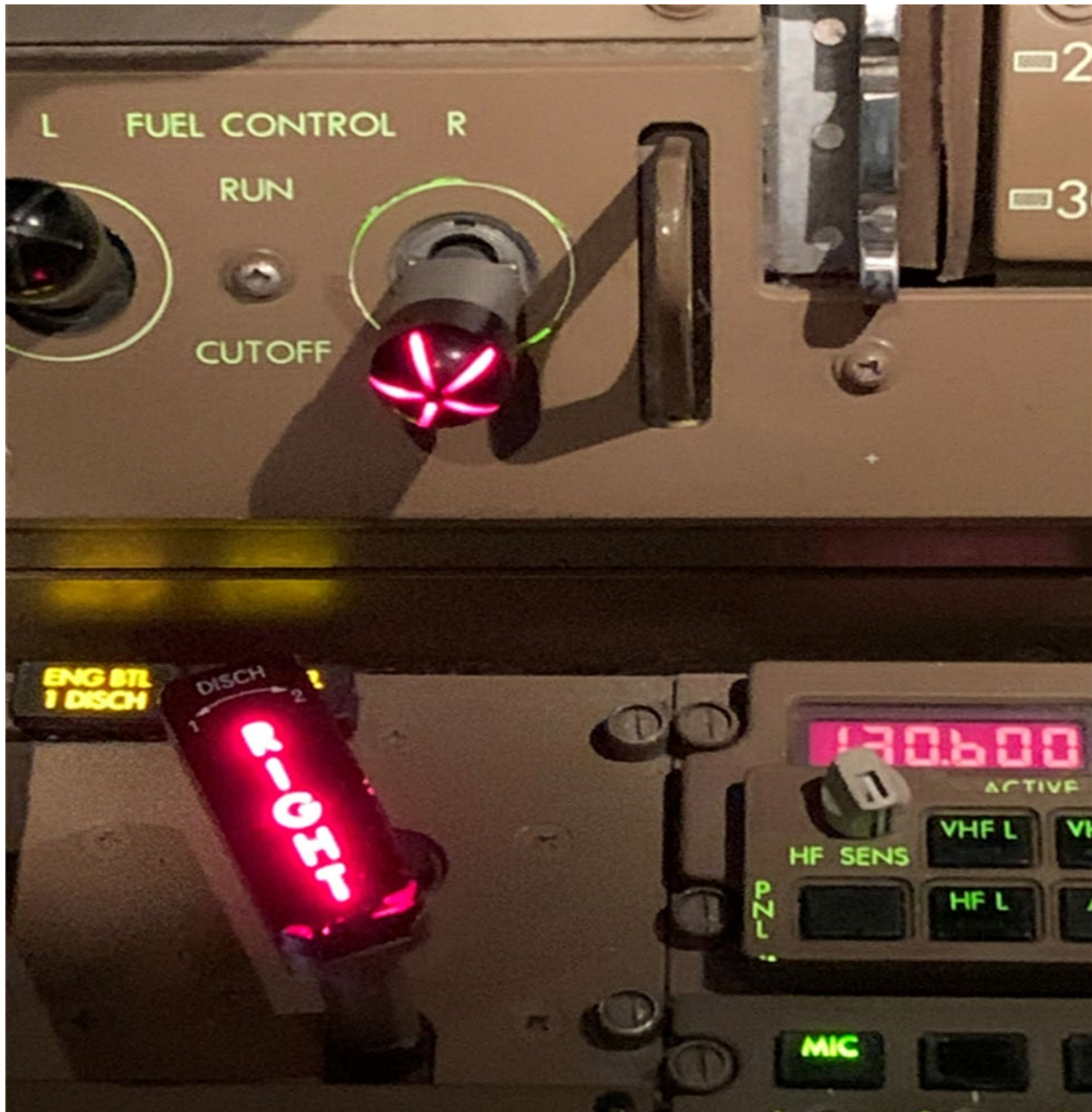
Photo 2: United Airlines B-777A, model simulator showing Right Engine Fire (Source: Attachment 2: 777 Simulator and Cockpit Observations)
