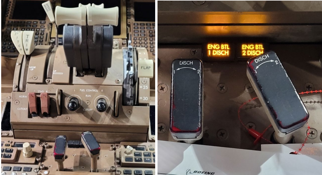
Figure 18 - Engine Fire Switches on incident airplane
