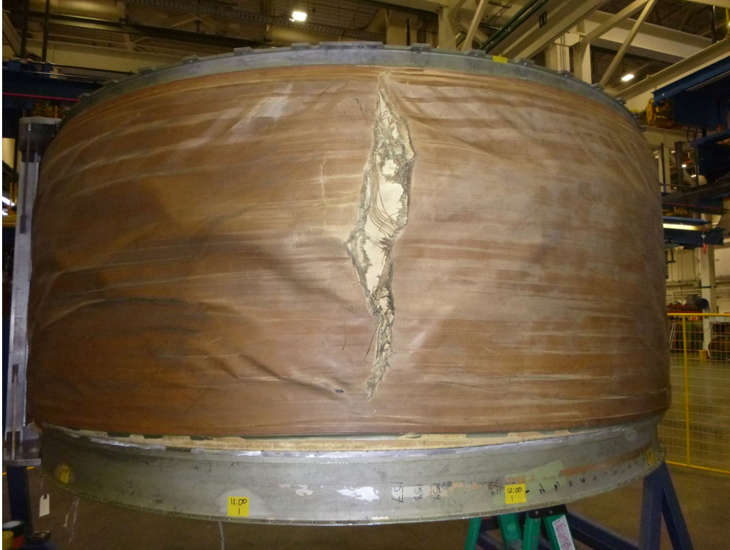
Figure 8 - Tear in outer layers of containment belt near 11:30 position
