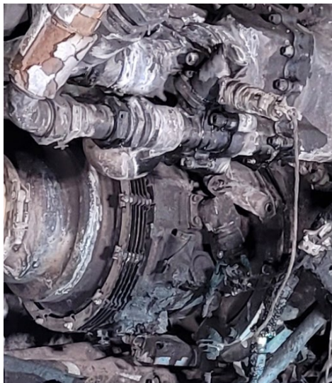
Figure 25 - Solenoid valve on engine driven pump on incident airplane
