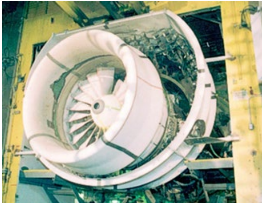
Figure 29 - Certification FBO test engine and inlet damage
