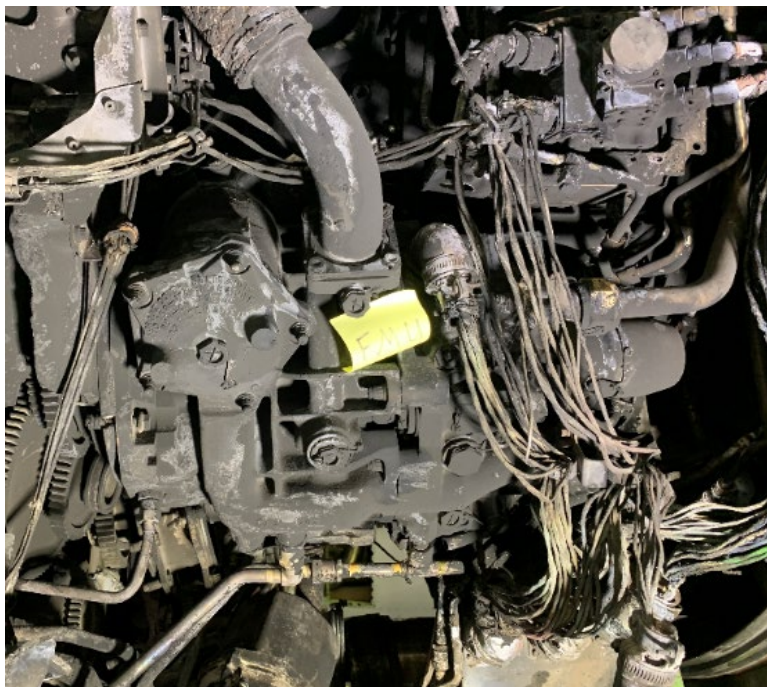
Figure 27 - Right engine fuel metering unit on incident airplane
