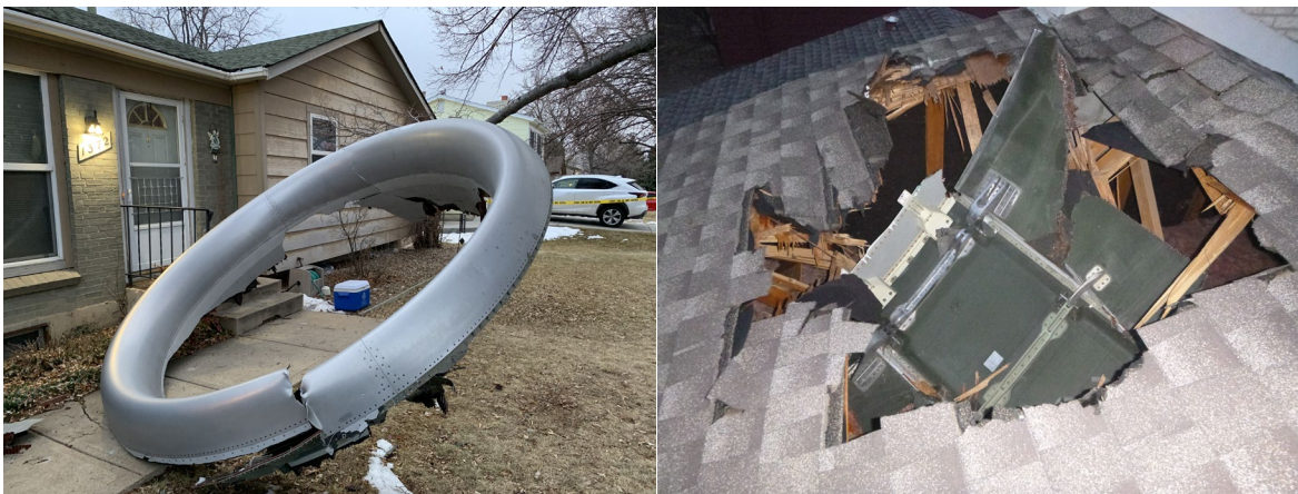
Figure 6 - Inlet lip skin(left) and fan cowl support beam (right) as found
