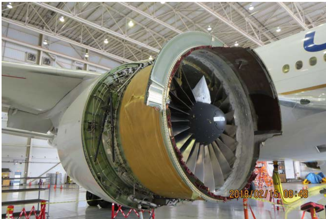
Figure 31 - UAL 1175 left engine, fan cowl, and inlet damage
