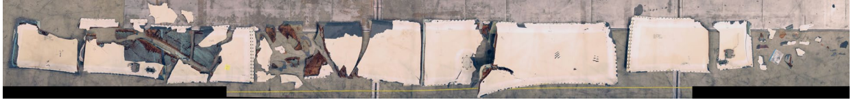
Figure 13 - Inlet outer barrel reconstruction, inner surface
