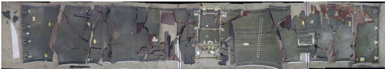
Figure 14 - Fan Cowl reconstruction, inner surface
