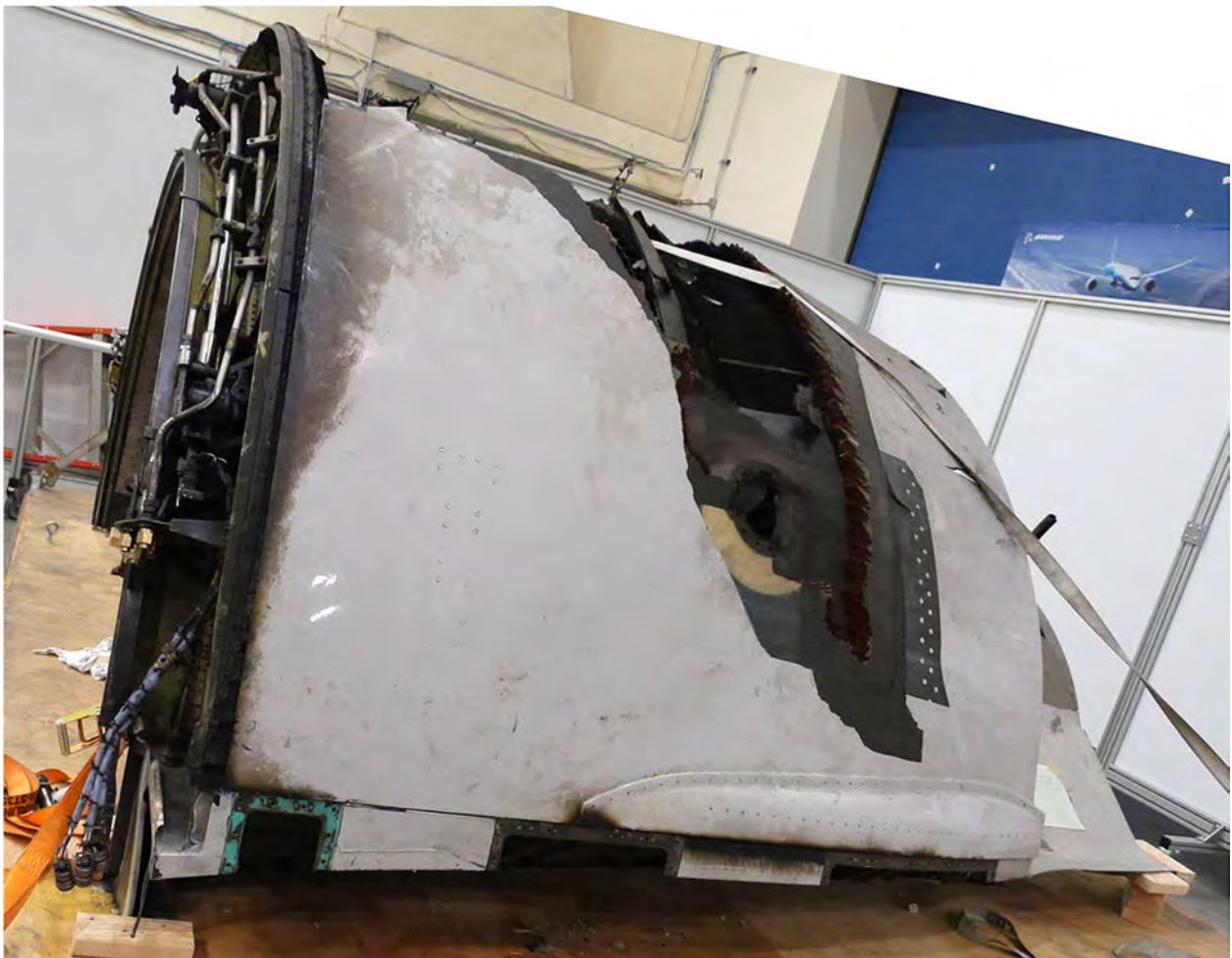
Figure 39: Outboard thrust reverser hinge beam and translating sleeve (view looking down).
