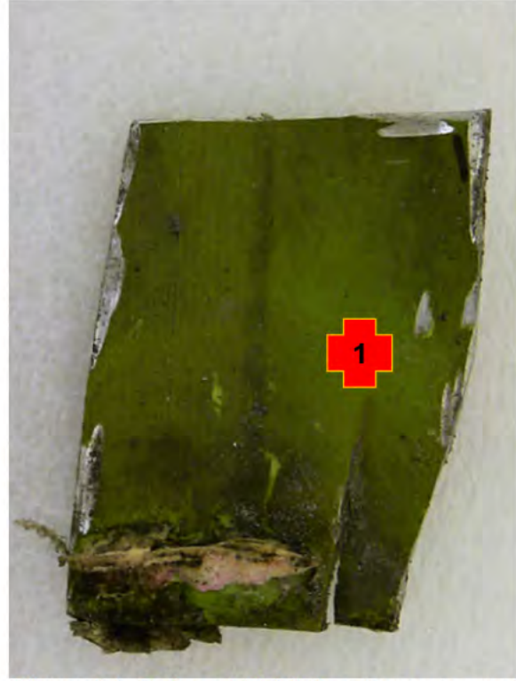
Figure 84: Outboard (right) thrust reverser crack at 12:00 removed.
