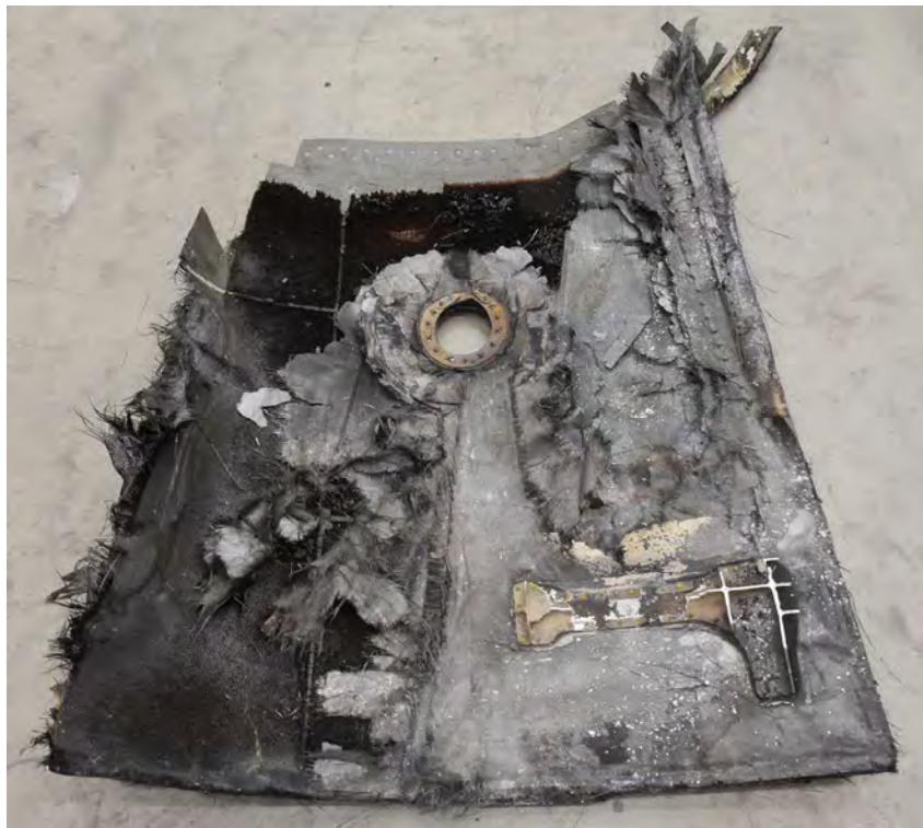
Figure 47: Translating sleeve separated from outboard thrust reverser, inner surface.
