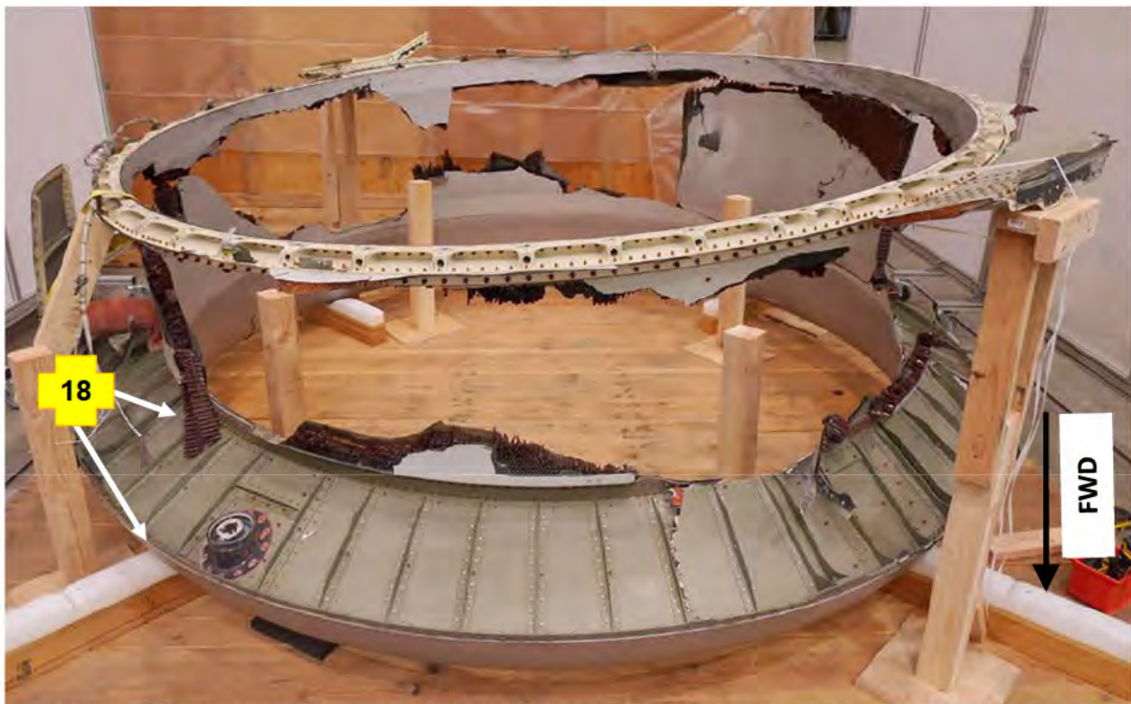
Figure 13: Inlet cowl lipskin, forward bulkhead and inlet attach ring supported by lumber to allow reconstruction of fragments recovered from the incident location.
