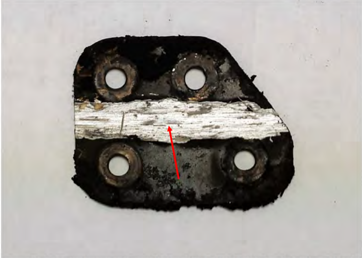
Figure 32. As received gooseneck assembly base (P/N 315W3422-13) from Door Access Panel Assembly. The fracture is indicated by the red arrow.
