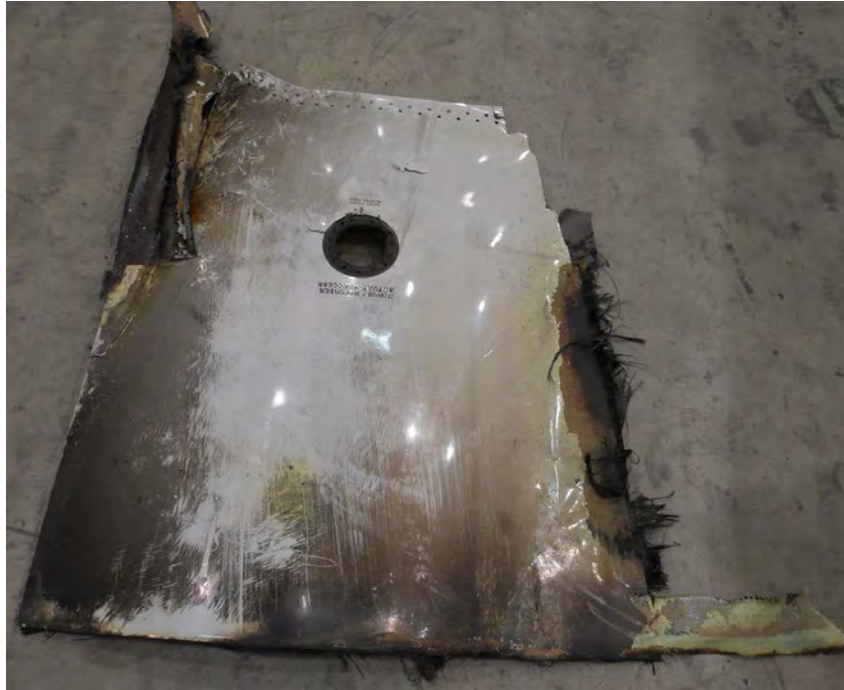
Figure 46: Translating sleeve separated from outboard thrust reverser, outer surface.
