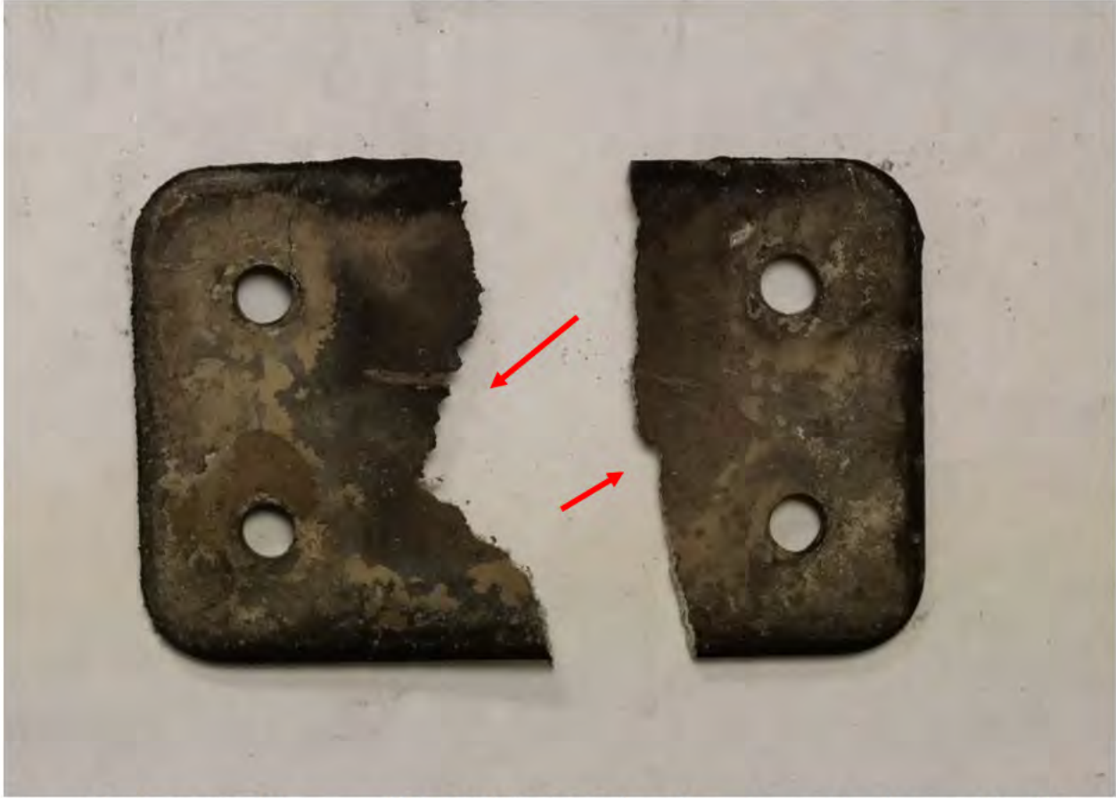
Figure 34. As received depressor (P/N 315W3419-3) from Door Access Panel Assembly. The fractures are indicated by the red arrows.
