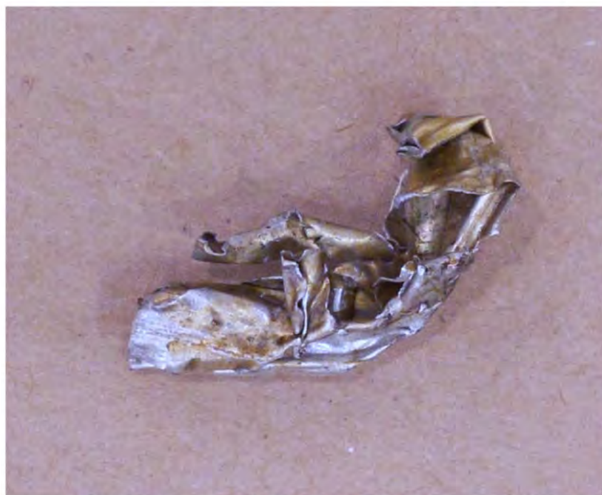
Figure 62: Fragment removed from inner wall of translating sleeve at 2:45.
