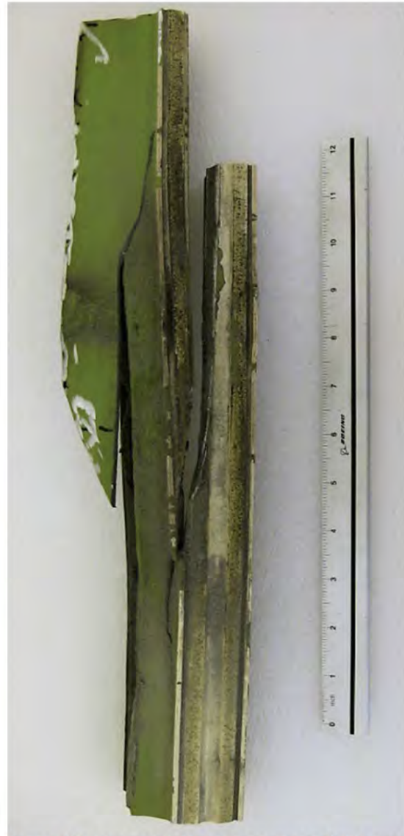
Figure 88: Inboard (left) thrust reverser 9:00 crack removed.
