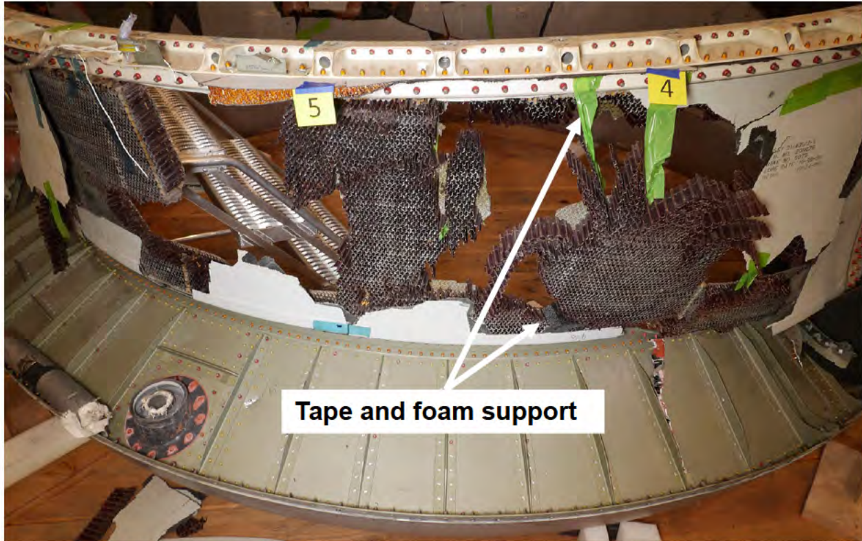
Figure 14: Inlet cowl with fragments reassembled to assist in incident investigation.
