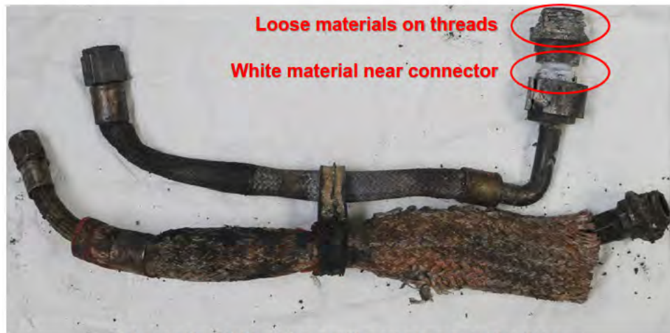
Figure 6 – BUG oil lines with sample areas identified
