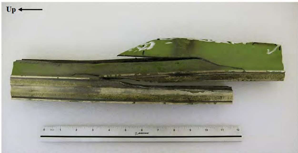
Figure 16. Left Thrust Reverser fracture at the 9:00 clock position after removal.
