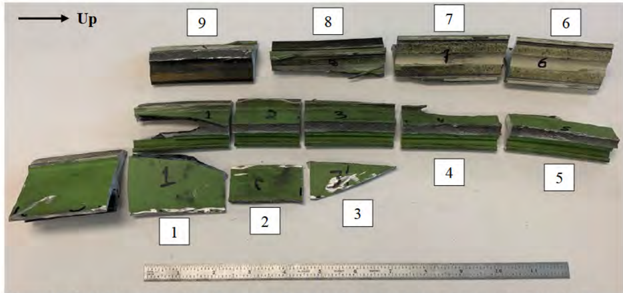
Figure 17. Left Thrust Reverser fracture at the 9:00 clock position cut into sections for SEM examination with the sections labeled.
