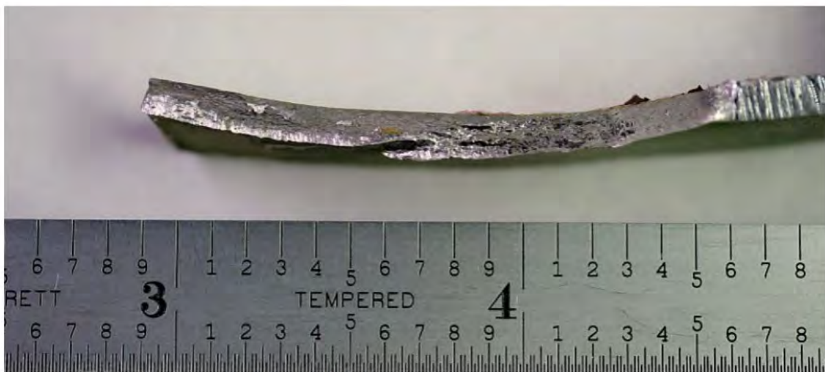
Figure 4. Macro photograph of the Right Thrust Reverser fracture initiation.
