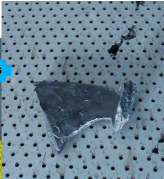
Figure 60: Outboard thrust reverser, fragment removed from near 3:00, detail.
