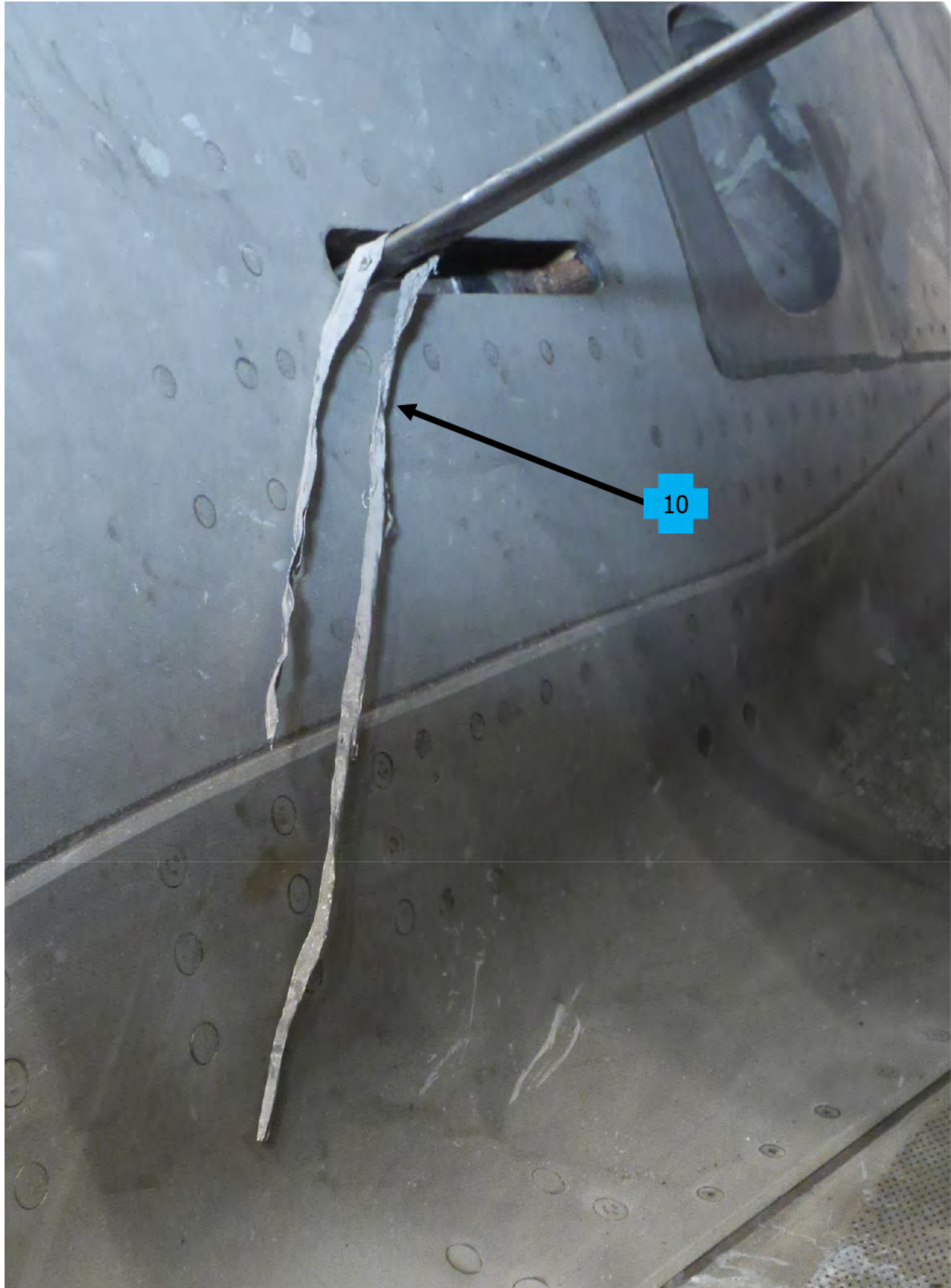
Figure 65: Material removed from blocker door drag link at 12:30.
