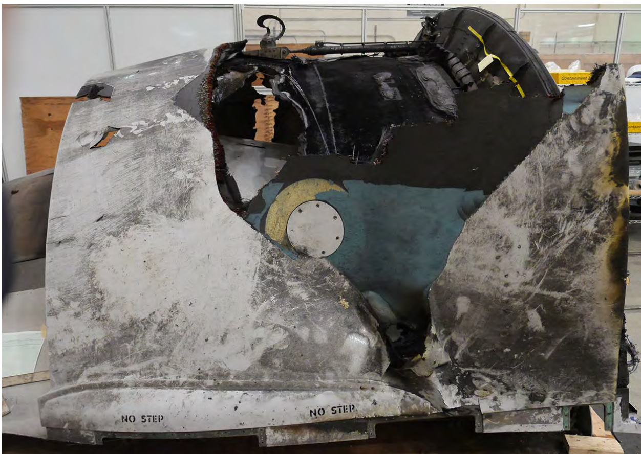
Figure 67: Inboard thrust reverser hinge beam, showing damage to translating sleeve and cascades (view looking down).
