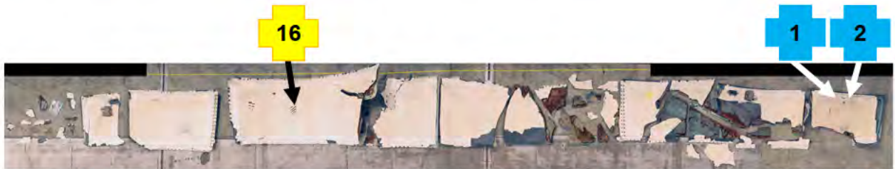
Figure 17: Inlet cowl outer barrel inner surface. Image created using merged photos. Zoom to view at full resolution.
