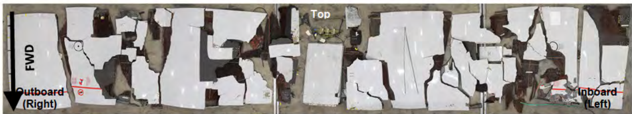
Figure 26: Fan cowl and fan cowl support beam outer surface reconstruction. Image created using merged photos. Zoom to view at full resolution.
