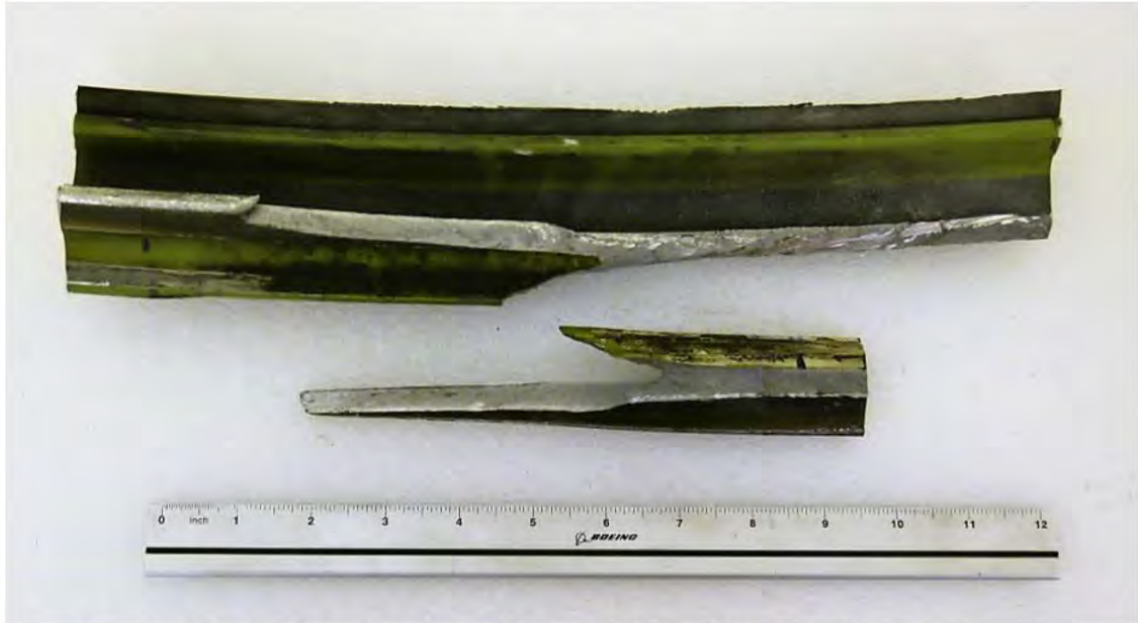
Figure 8. Left Thrust Reverser fracture at the 7:00 clock position after removal.
