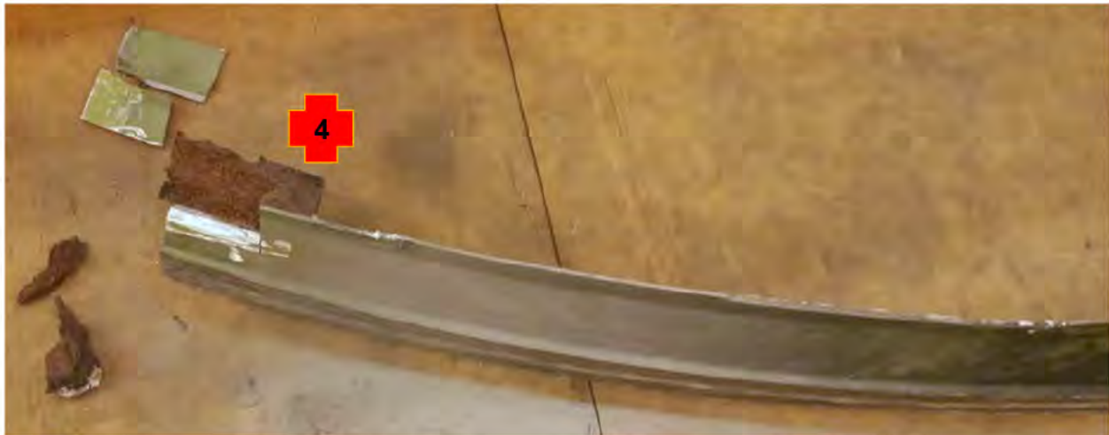
Figure 89: Inboard (left) thrust reverser crack at 12:00 removed.
