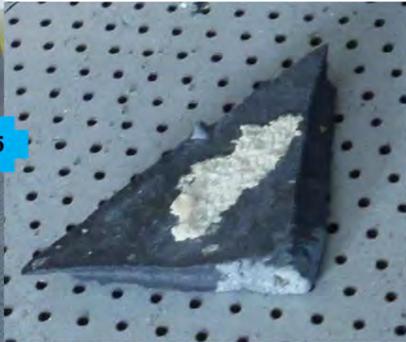
Figure 58: Outboard thrust reverser, fragment removed from near 3:30, detail.
