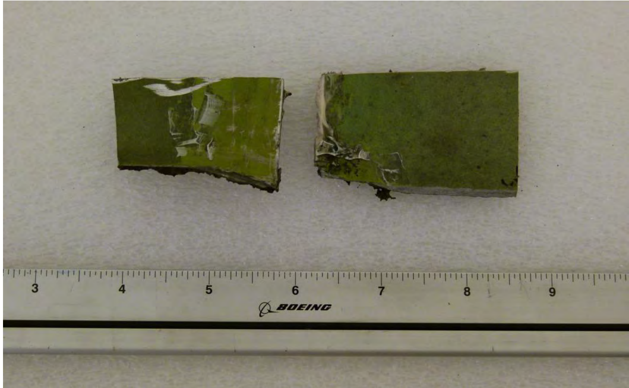
Figure 28. Left Thrust Reverser fracture at the 12:00 clock position after removal.
