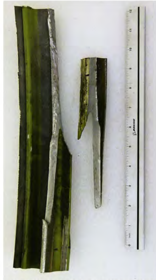
Figure 86: Inboard (left) thrust reverser crack at 7:00 removed.
