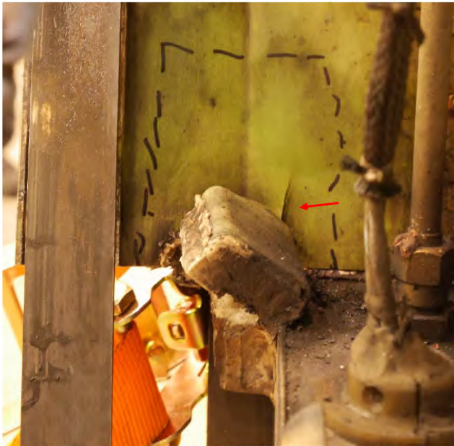
Figure 2. Right Thrust Reverser fracture at the 12:00 clock position before removal.
