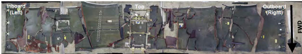
Figure 25: Fan cowl and fan cowl support beam inner surface reconstruction. Image created using merged photos. Zoom to view at full resolution.
