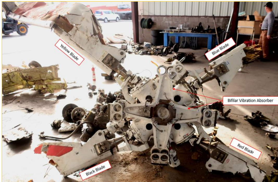
Photo 3-Rotor head with blade sections annotated.
