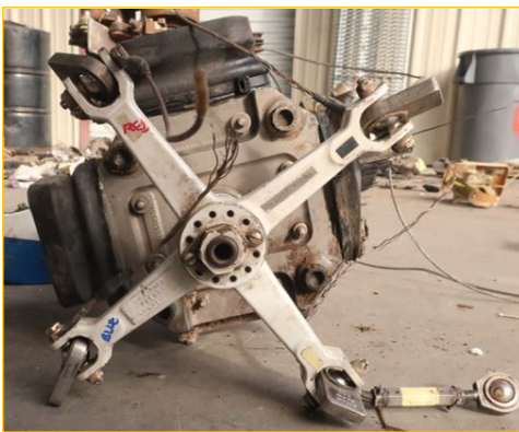
Photo 5-Tail rotor hub pitch beam.
