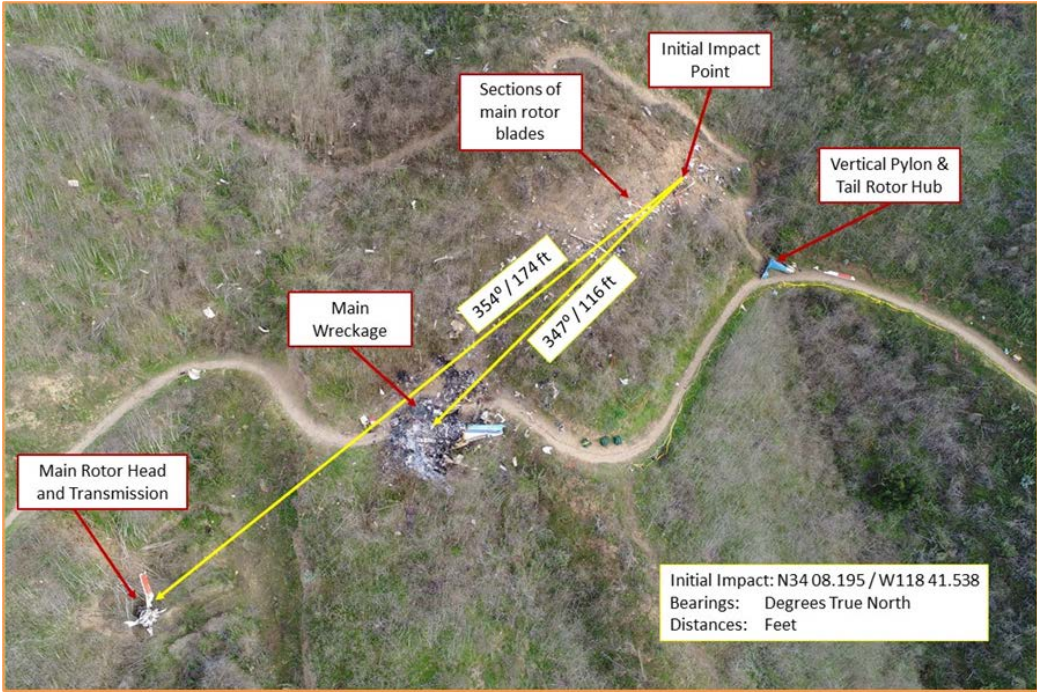
Figure 3 - Wreckage diagram. Overall view of initial impact area and wreckage path with select measurements and significant items.
