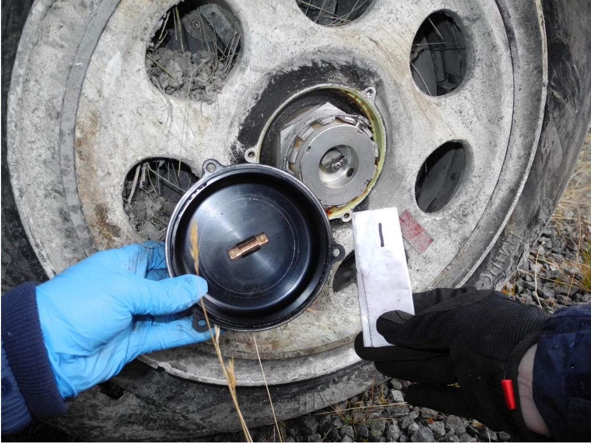
Figure 28 #1 wheel hubcap with transducer clip
