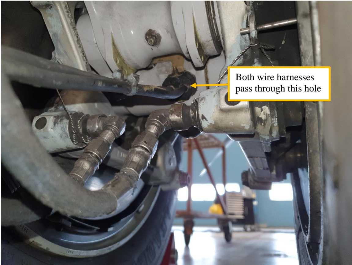
Figure 27 Exemplar airplane wheel speed transducer wire harness routing at base of strut
