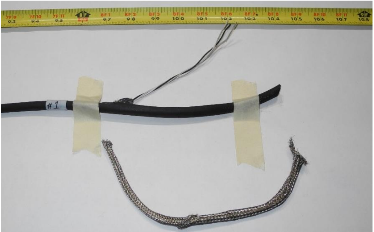
Figure A3 #1 wire harness fractured end showing 3 total wires
