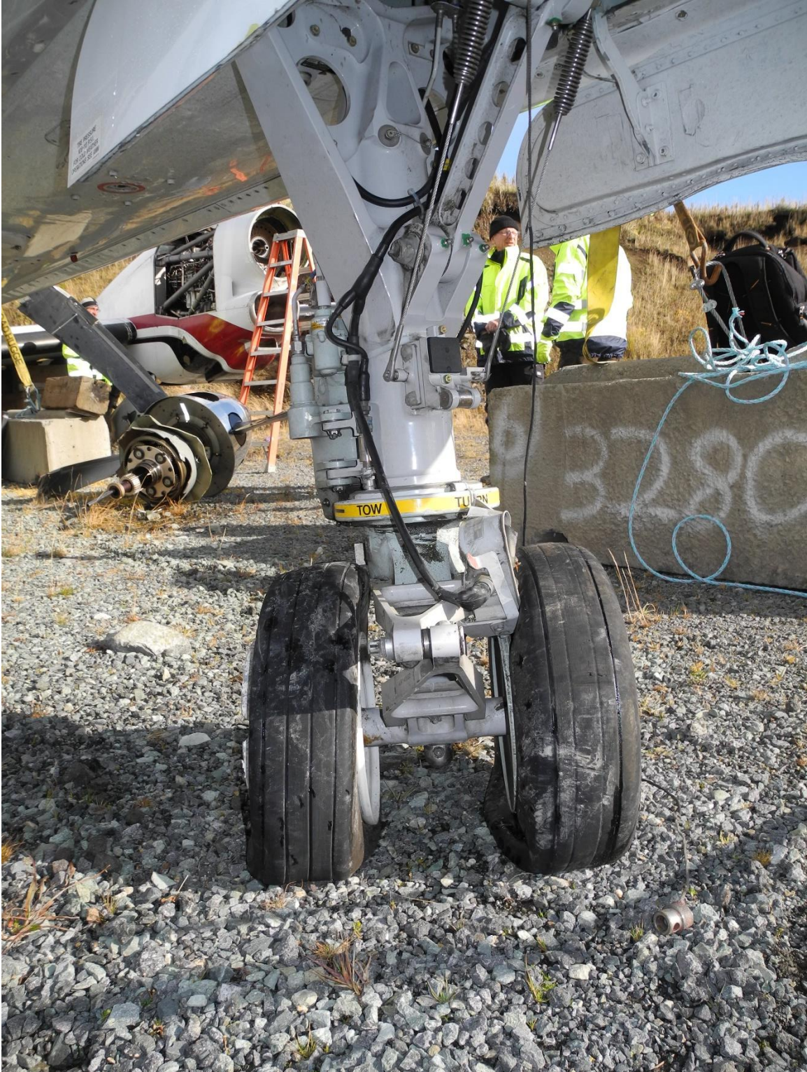
Figure 62 Nose gear and tires, right tire in contact with the light
