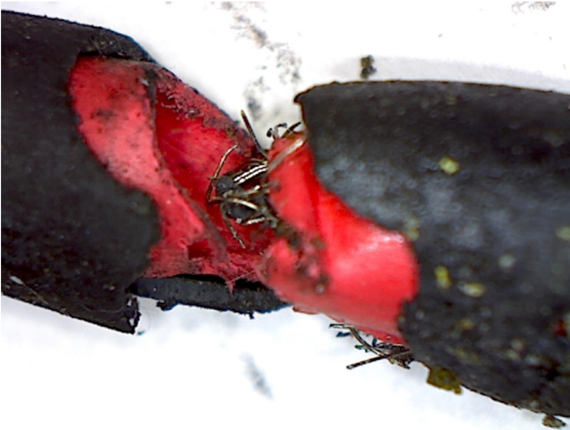
Figure A21 #1 wire harness fracture end (left) and short segment fracture end (right)
