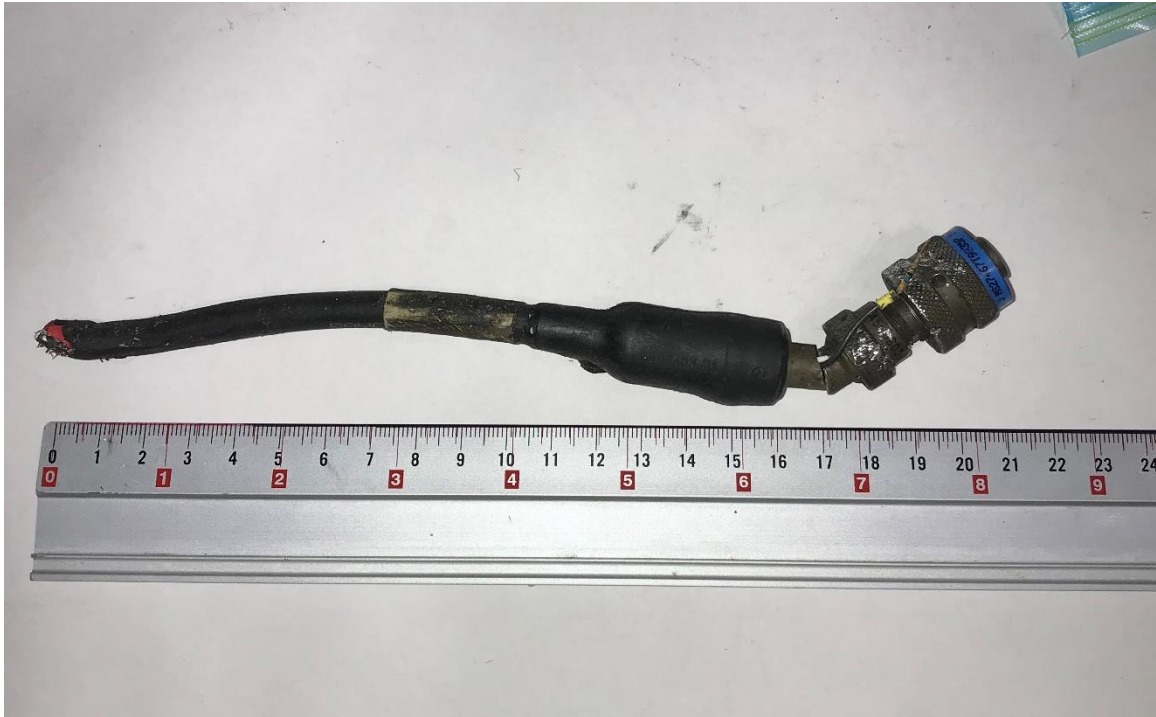
Figure A25 Short segment with upper connector dimension
