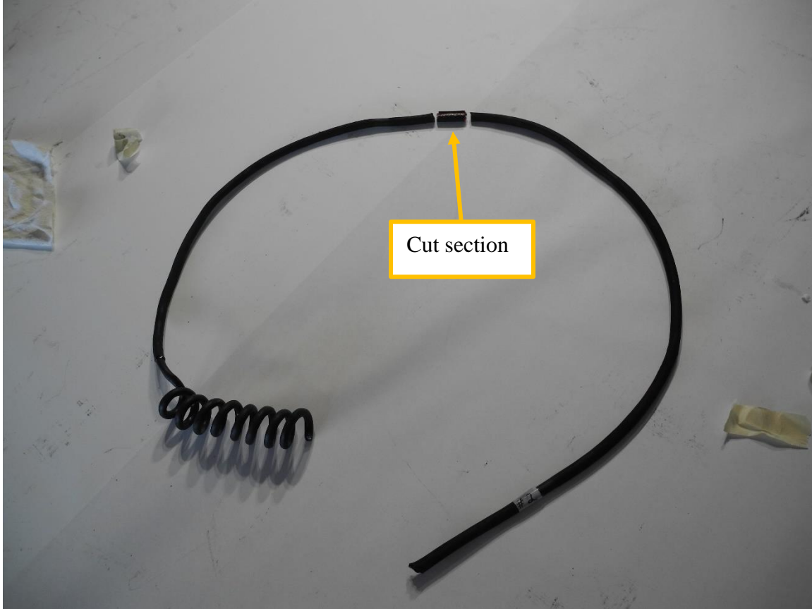
Figure A26 #2 harness with small segment cut out of middle
