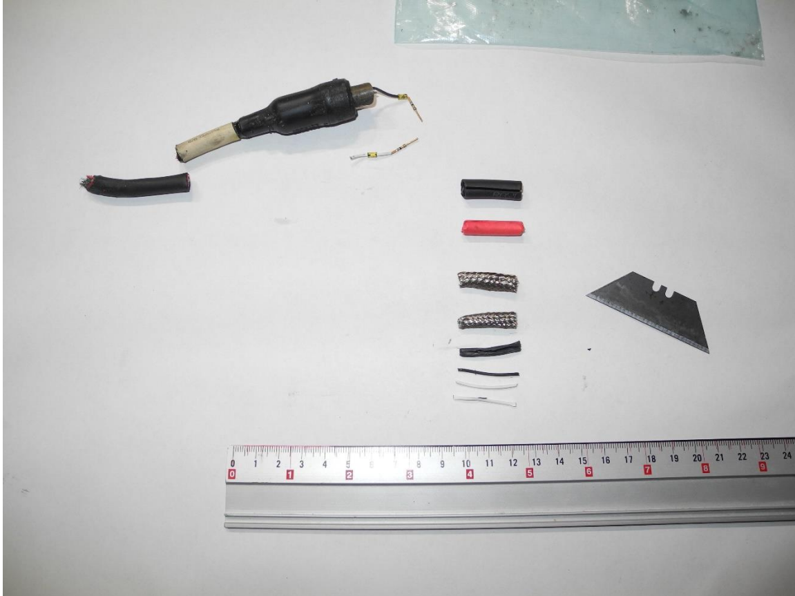
Figure A29 Short segment with 1 inch segment cut from middle, shows 3 total wires
