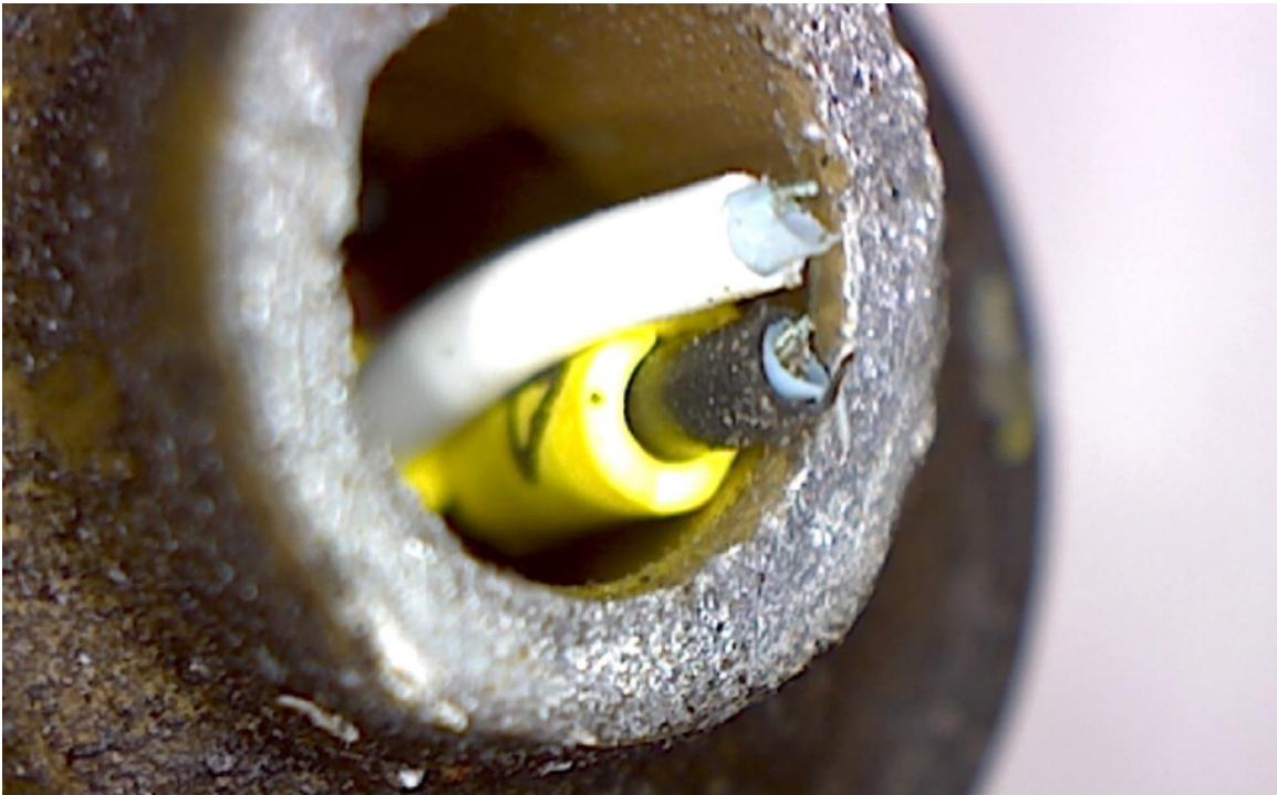
Figure A20 Lower connector wires still attached
