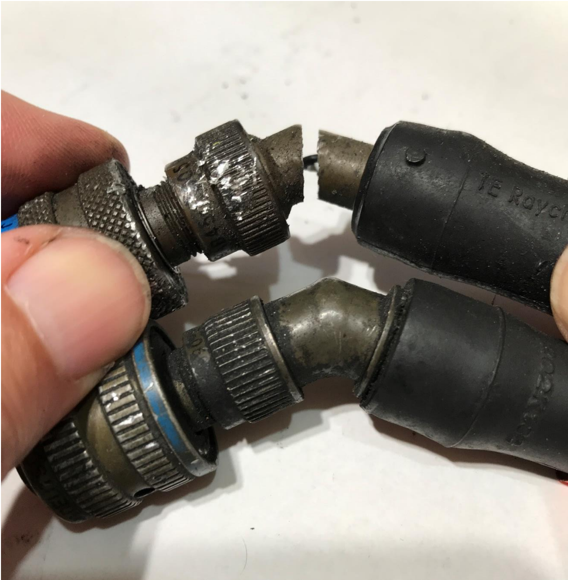
Figure A22 Fracture surfaces of connectors formed 45 degree elbow
