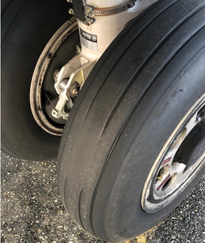
Figure 15 Flat spot on #1 tire prior to accident flight
