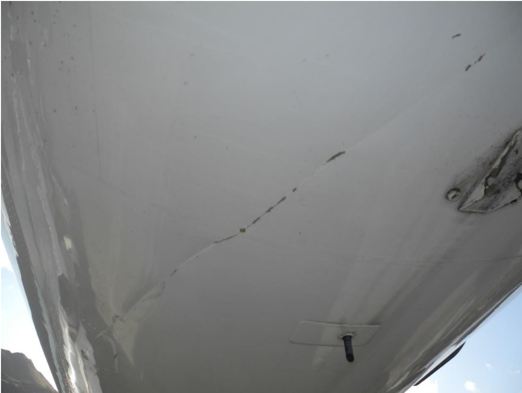
Figure 50 Scrape aft lower left fuselage
