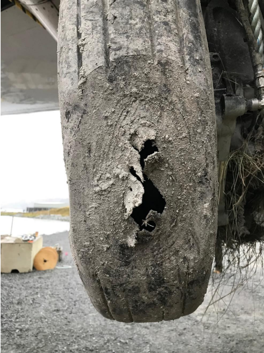
Figure 13 Hole in left outboard tire
