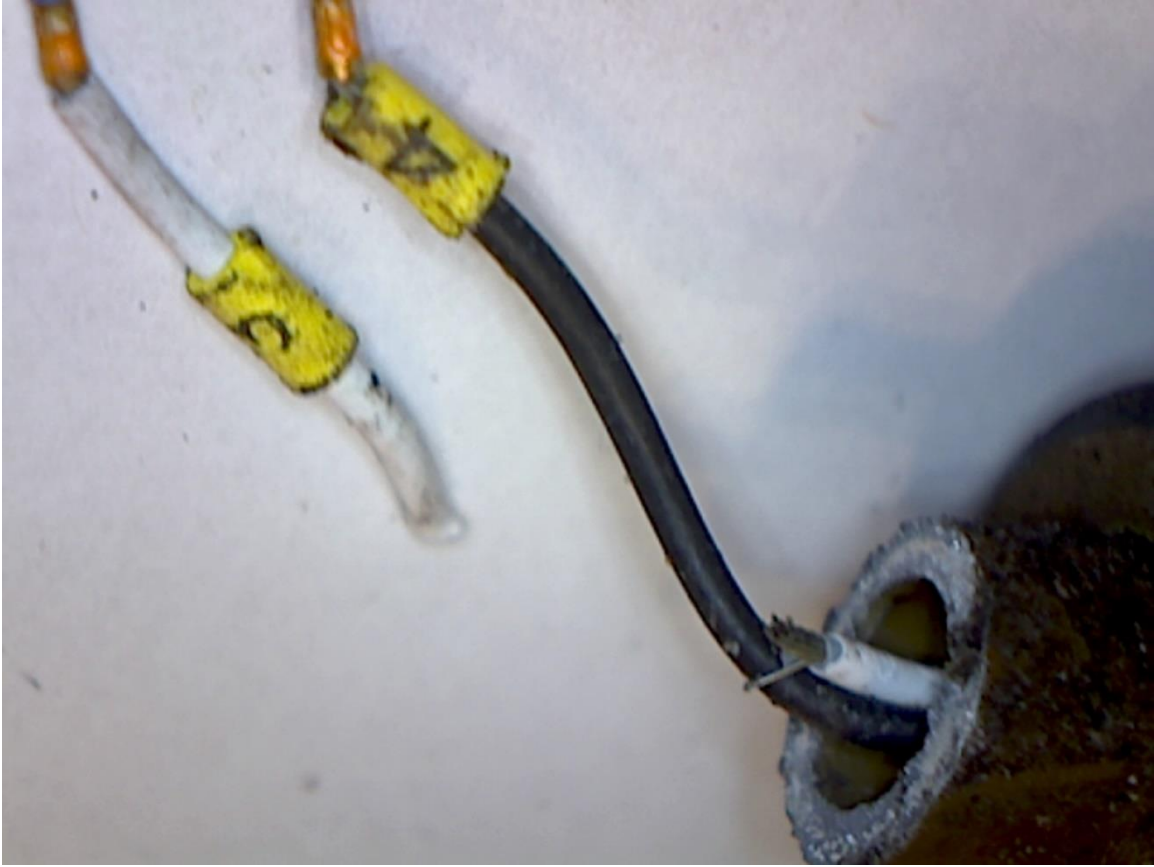
Figure A14 Short segment wire numbers
