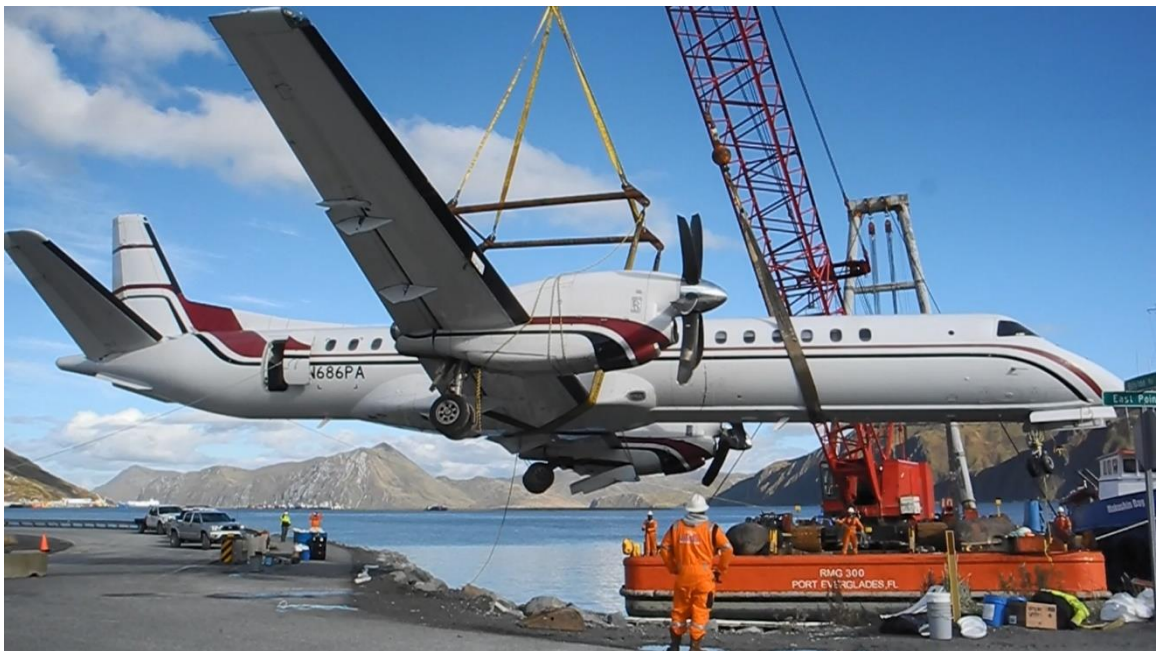
Figure 3 Airplane being lifted by crane onto barge
