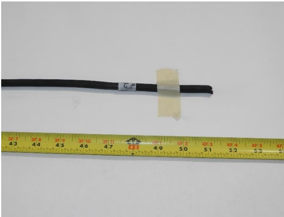
Figure A4 #2 wire harness fractured end
