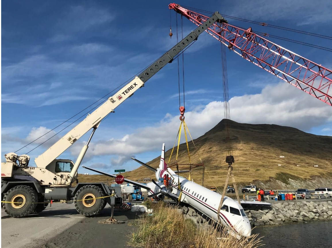
Figure 2 Airplane rigged for recovery
