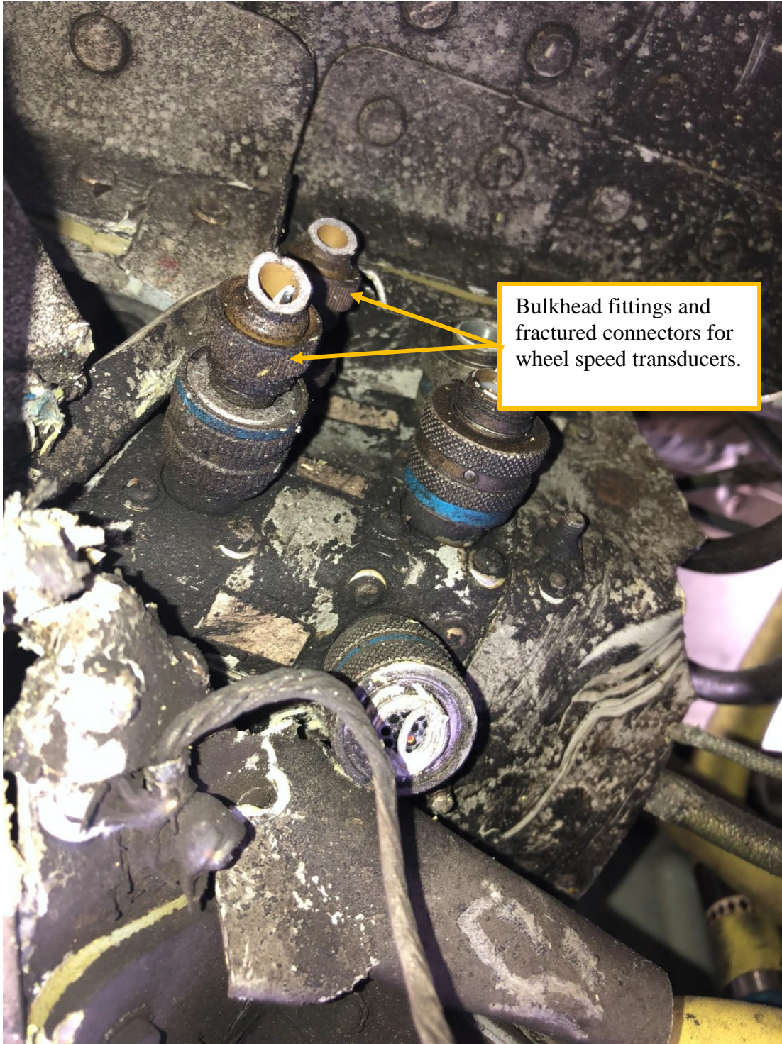
Figure 35 Left wheel well wheel speed transducer bulkhead fittings
