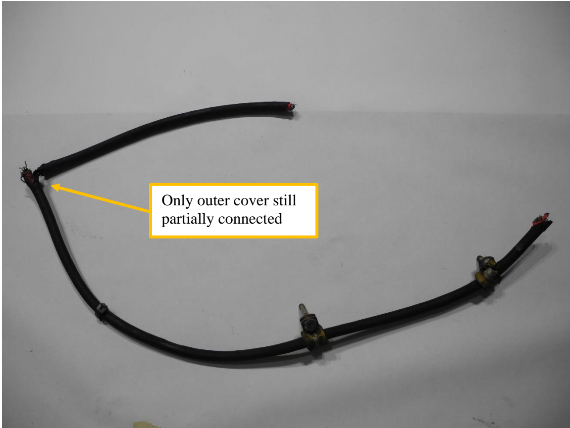
Figure A9 Long segment of wire harness
