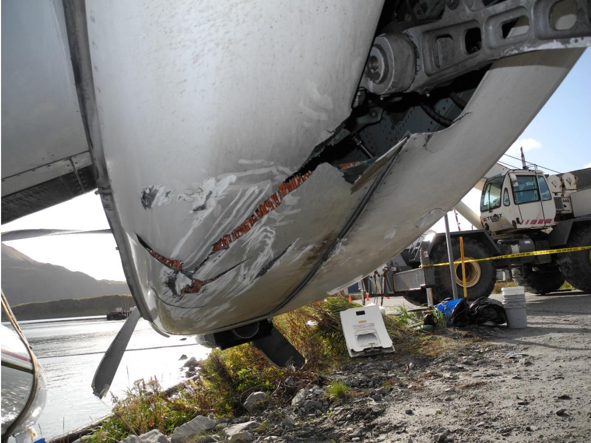
Figure 46 Right main gear door damage
