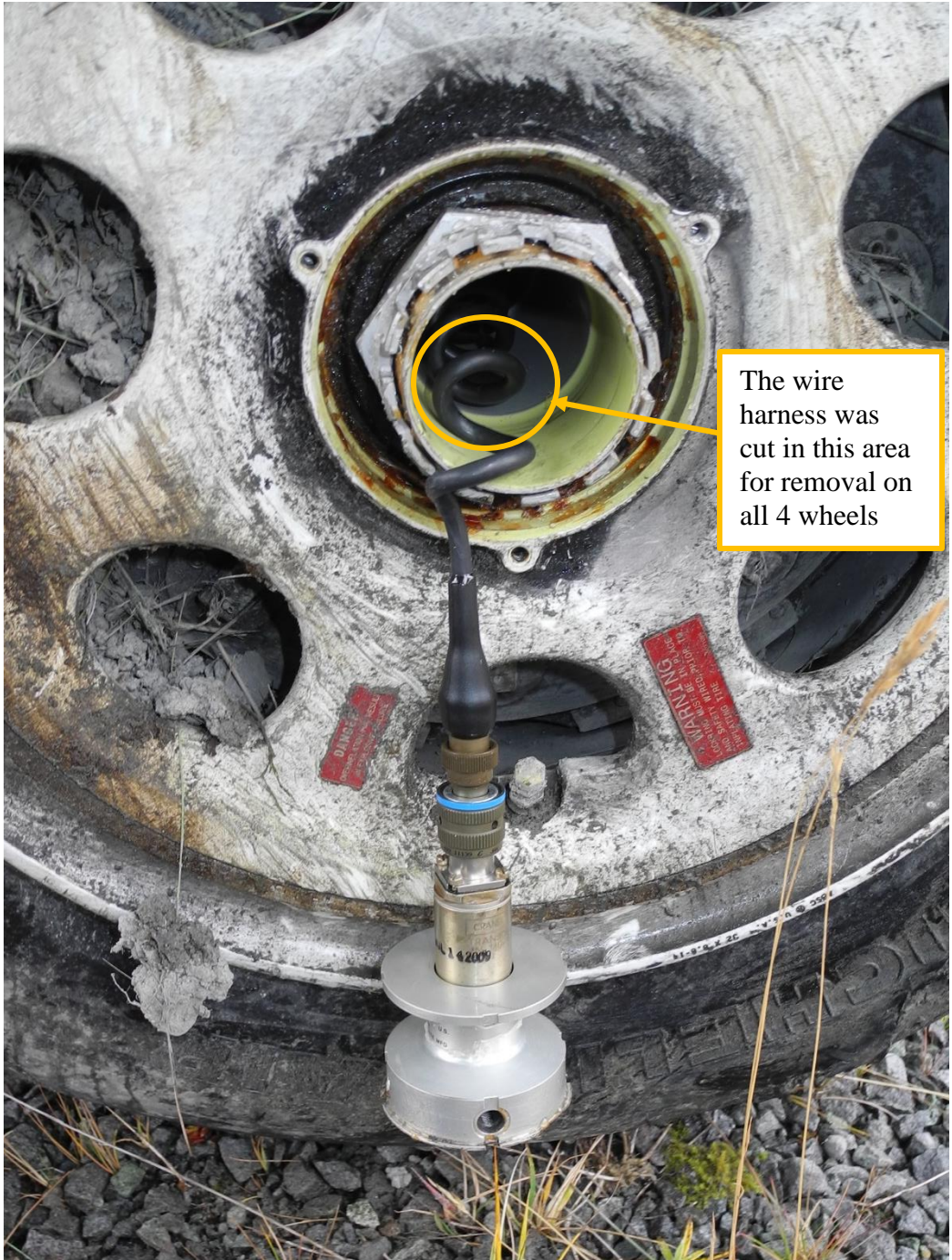
Figure 29 #1 wheel speed transducer removed from axle
