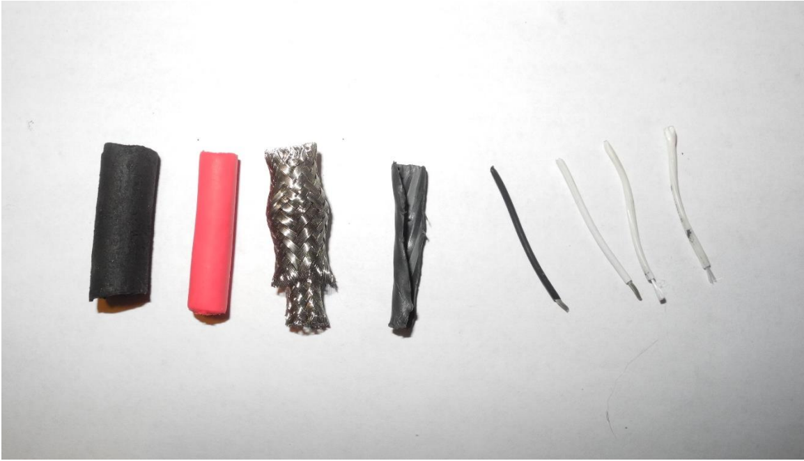
Figure A27 Disassembled #2 harness cut section
