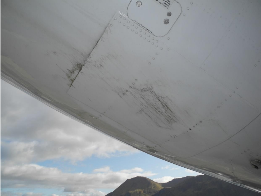
Figure 49 Scrapes on lower aft fuselage
