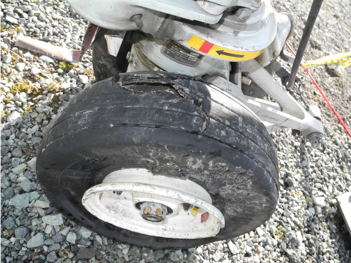
Figure 61 Punctured left tire
