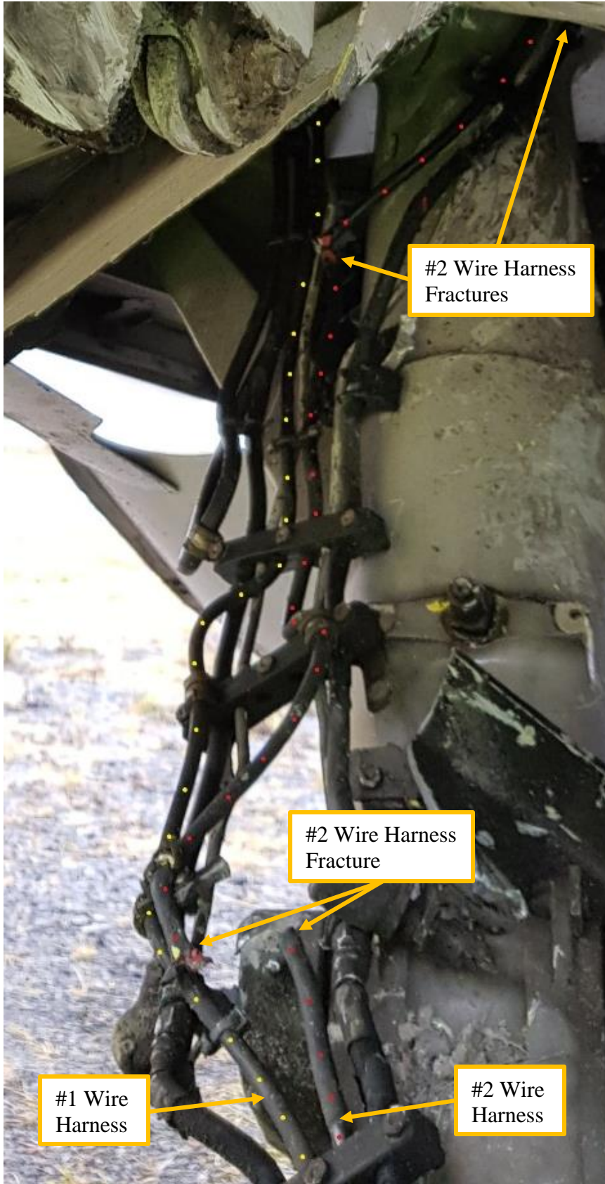
Figure 34 Left gear wheel speed transducer routing
