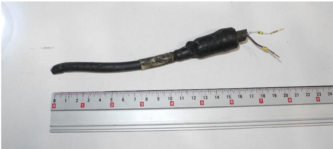
Figure A12 Short segment with connector portion and pins
