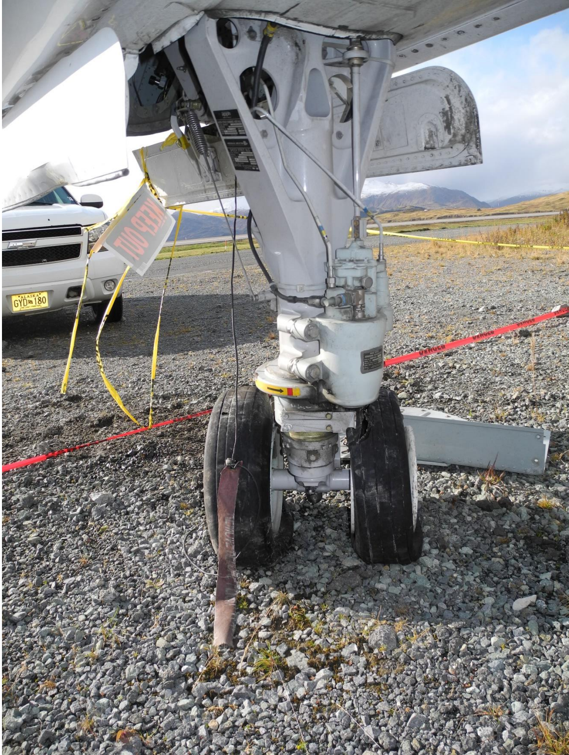
Figure 60 Nose gear and tires after recovery
