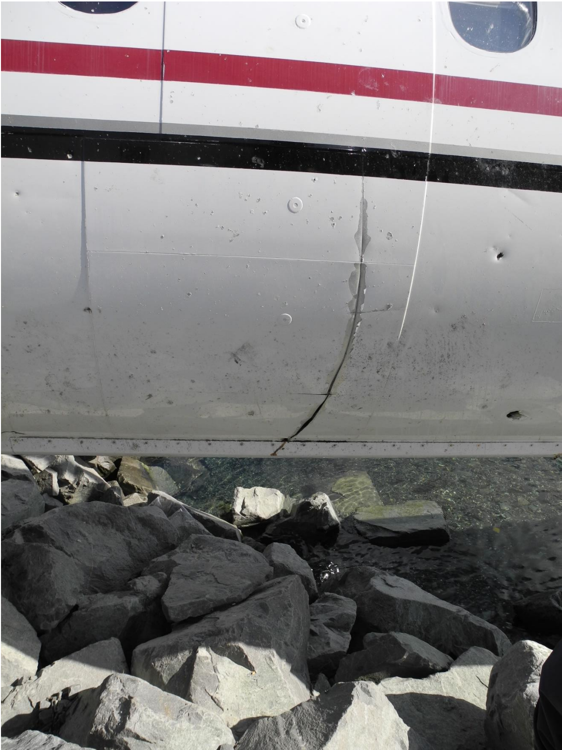
Figure 51 impact, punctures and dents, right side forward of wing.
