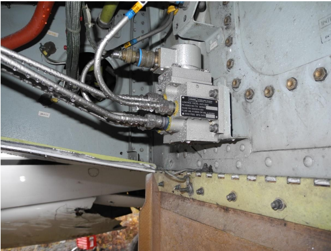
Figure 38 Inboard antiskid valve
