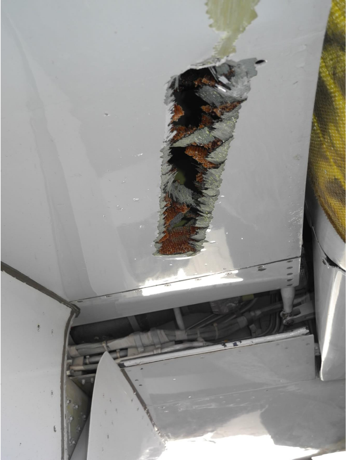
Figure 43 Damage to bottom inboard portion of flap
