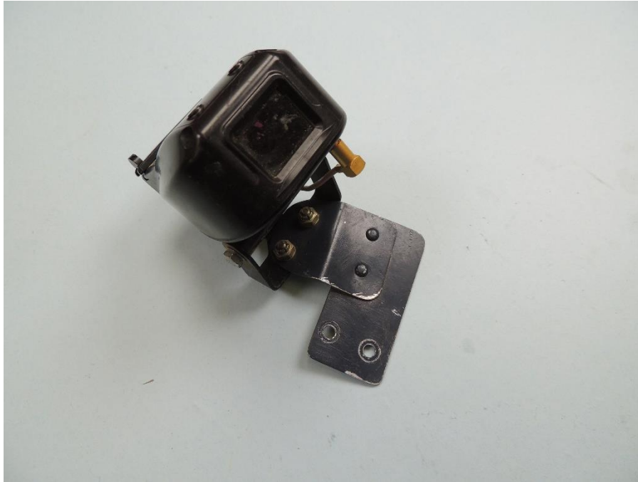
Figure 1. The Appareo Vision 1000 device as received. The associated SD card is not pictured.
