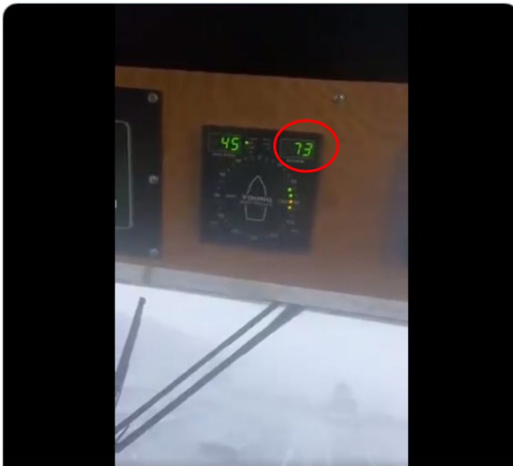
Figure 24 – Wind gust information from vessel located south-southwest of the accident vessel at the accident time
