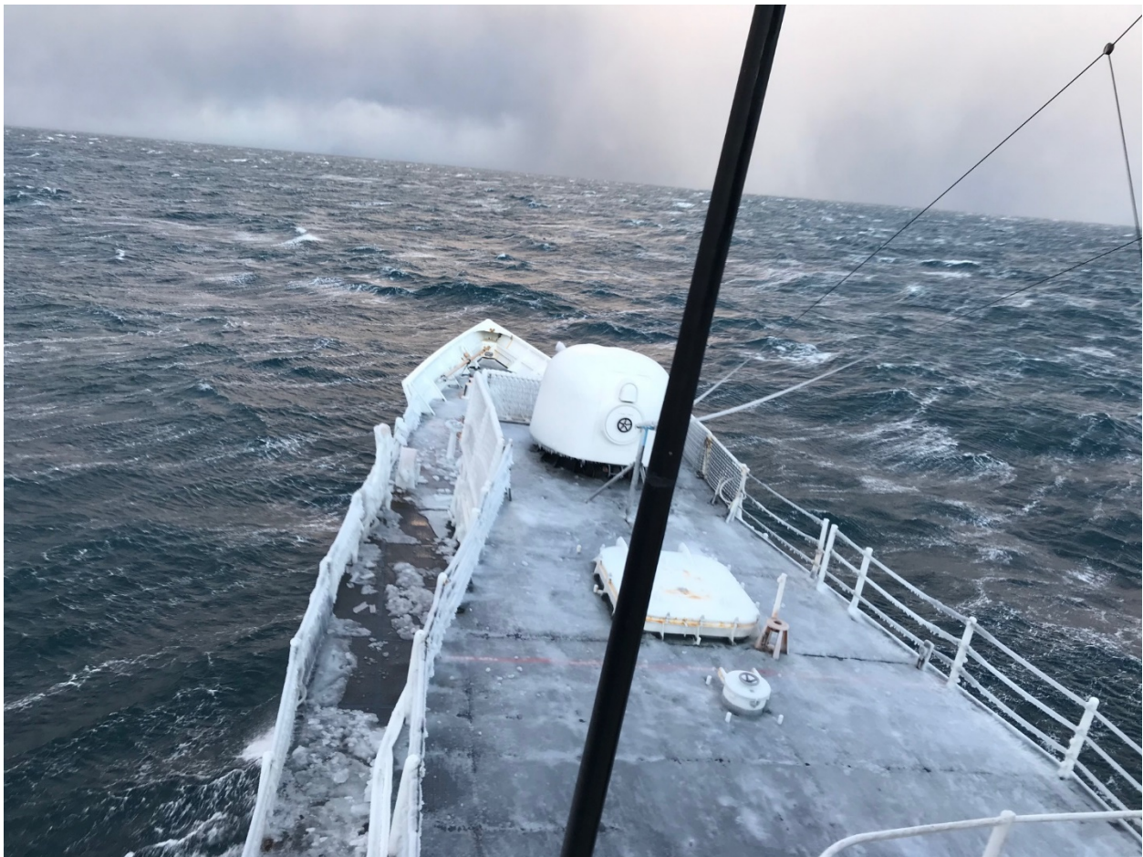
Figure 26 – USCG Mellon with icing on the vessel during the afternoon of January 1, 2020.
