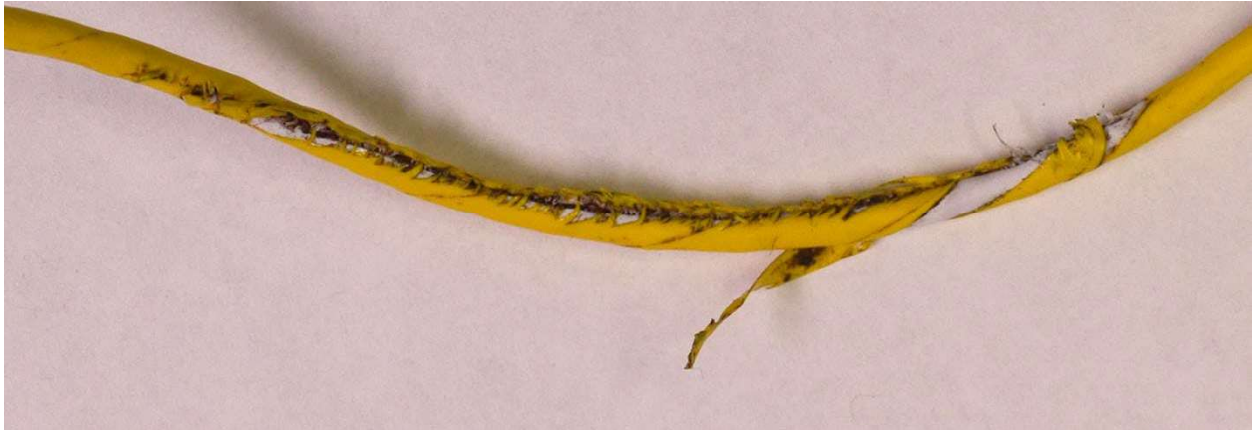
Figure 13 – RMLG yellow wire example of jacket damage
