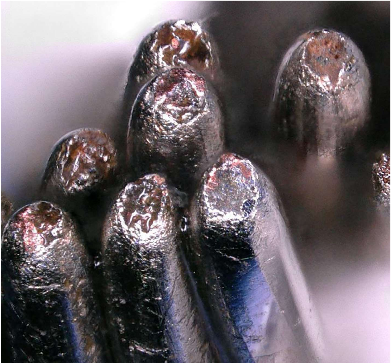
Figure 18 - RMLG blue wire fractured end showing necking and ductile overload
