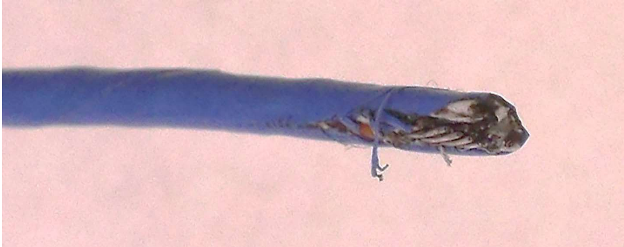
Figure 14 – RMLG blue wire fractured end
