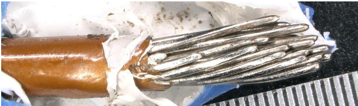
Figure 20 - RMLG blue wire fractured end with jacket peeled back
