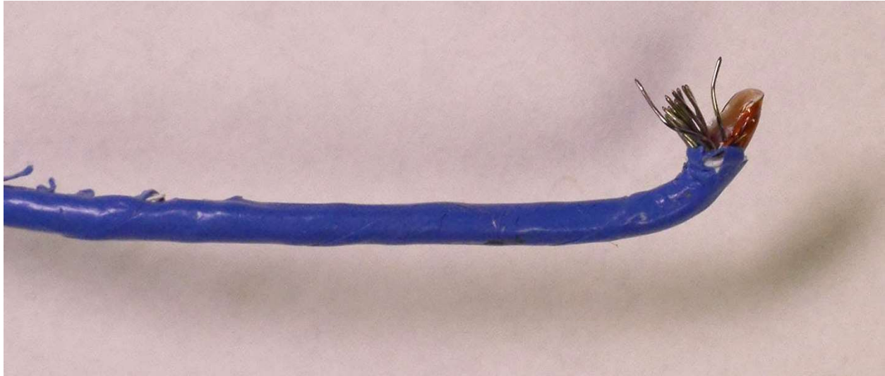
Figure 23 – Wire section 44 fractured end
