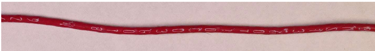
Figure 10 – RMLG red wire showing wire label
