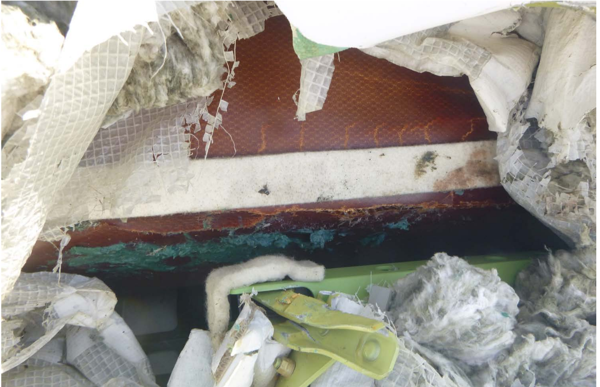
Figure 8 – Blue grease splatter inside fuselage hole
