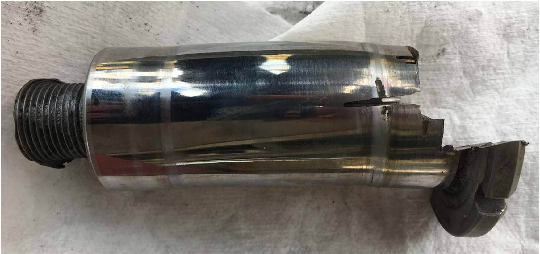
Figure 9 – Left pylon inboard aft upper spar fitting (R4) fuse pin
