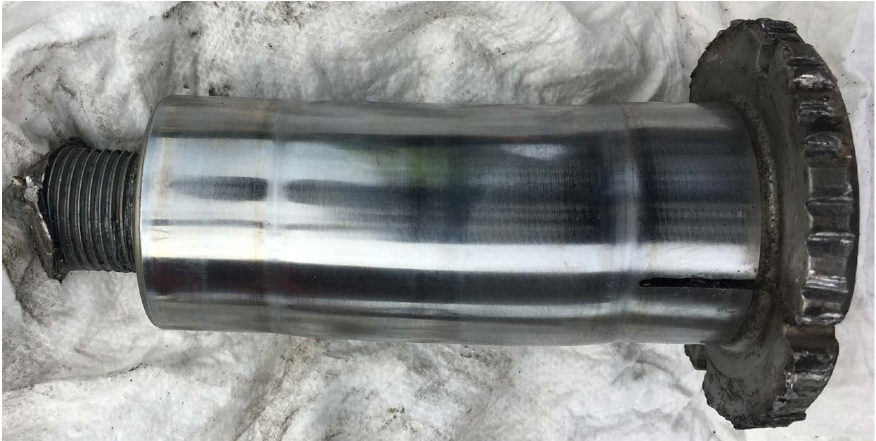
Figure 10 – Right pylon outboard aft upper spar fitting (R3) fuse pin
