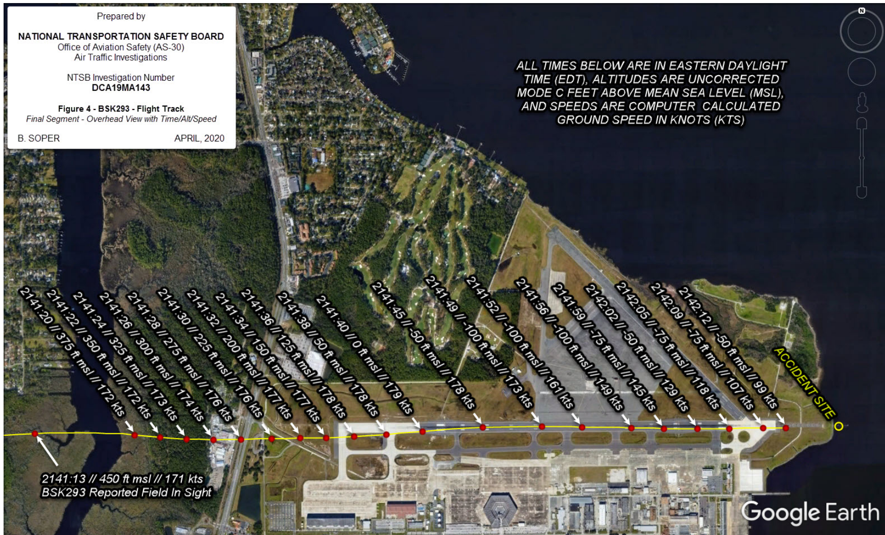
Figure 4 - Overhead view of final segment of accident flight track with time, altitude, and ground speed data depicted for reference.
