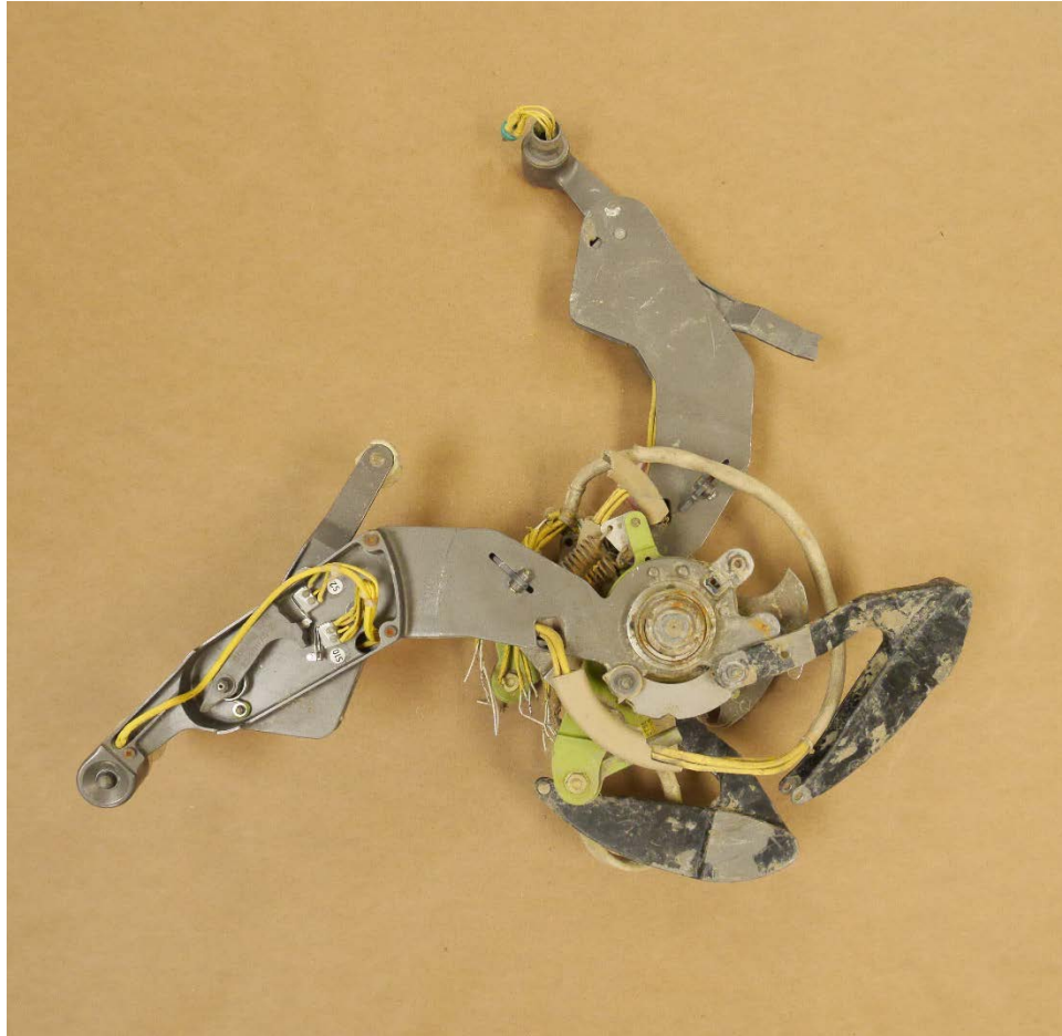
Figure 14 - Control Stand Thrust Lever Assembly and associated structure, as received at the Boeing EQA Laboratory.
