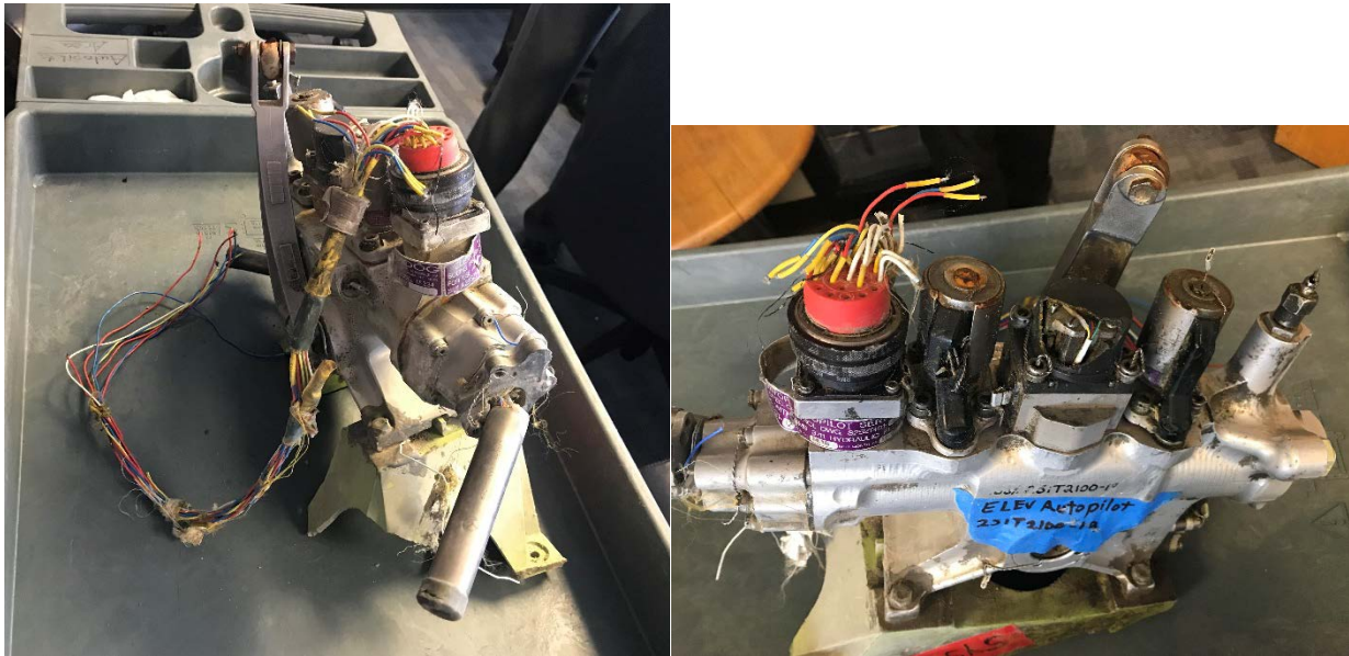
Figure 10a and 10b - The Center Autopilot Elevator Servo.
