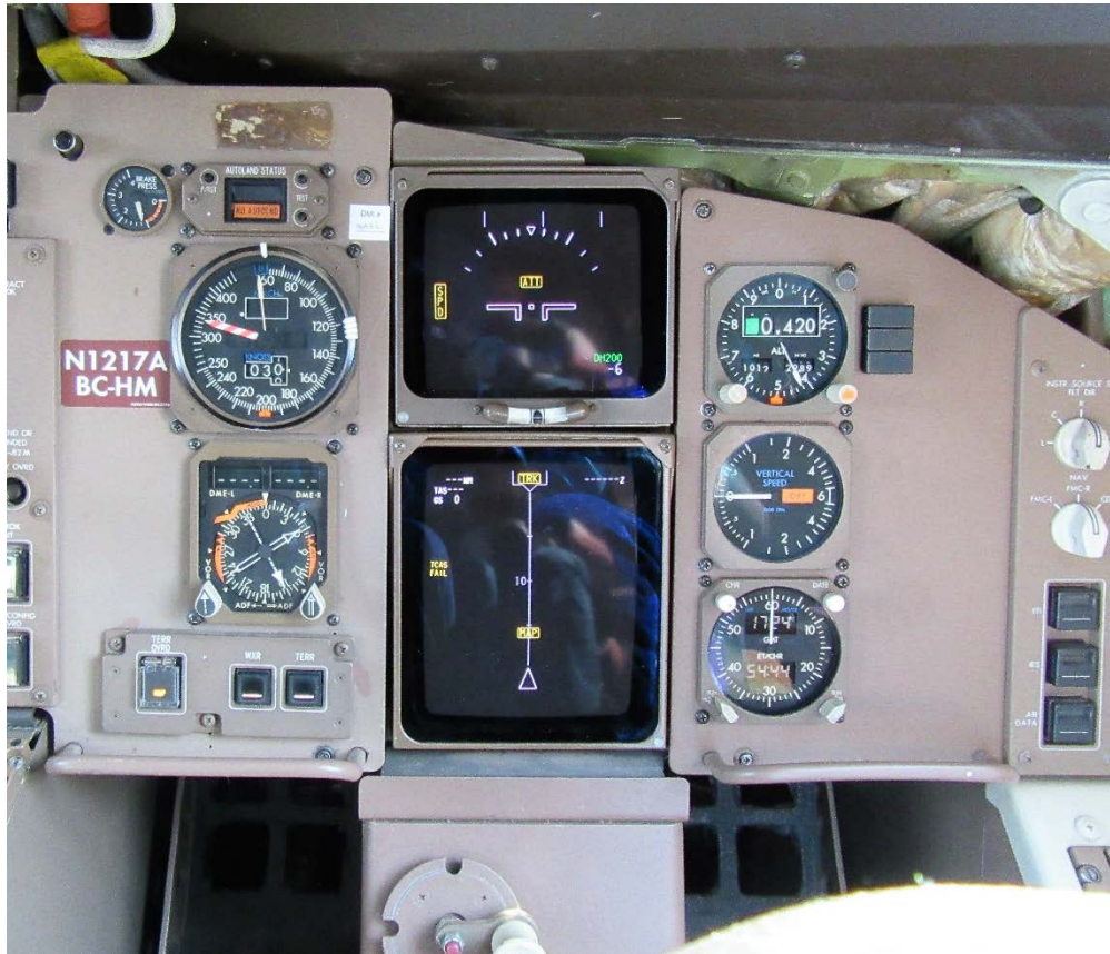
Figure 16 - The First Officer's Flight Instrument Panels. Note: this photograph was taken during the airplane's freighter conversion in 2017.
