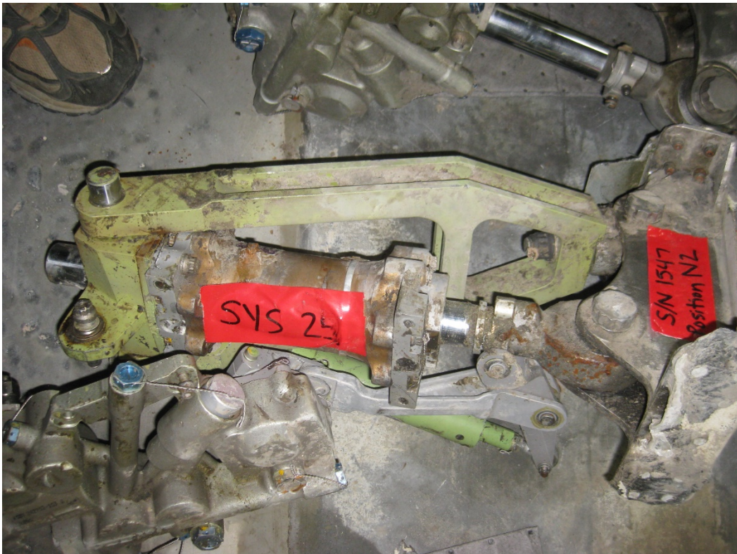
Figure 6 - Elevator PCA Serial Number 1547, as recovered in warehouse.
