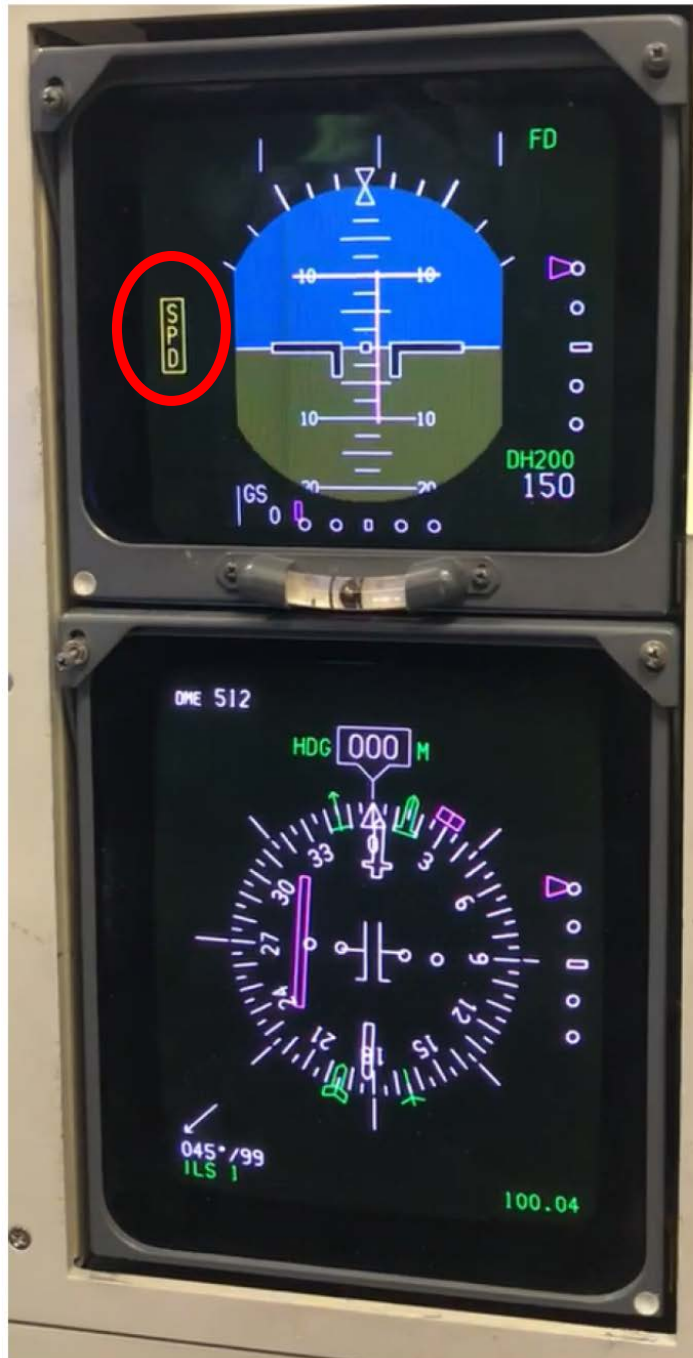
Figure 19 - EFIS Displays with Airspeed Flagged. The Airspeed Flag is circled in red.
