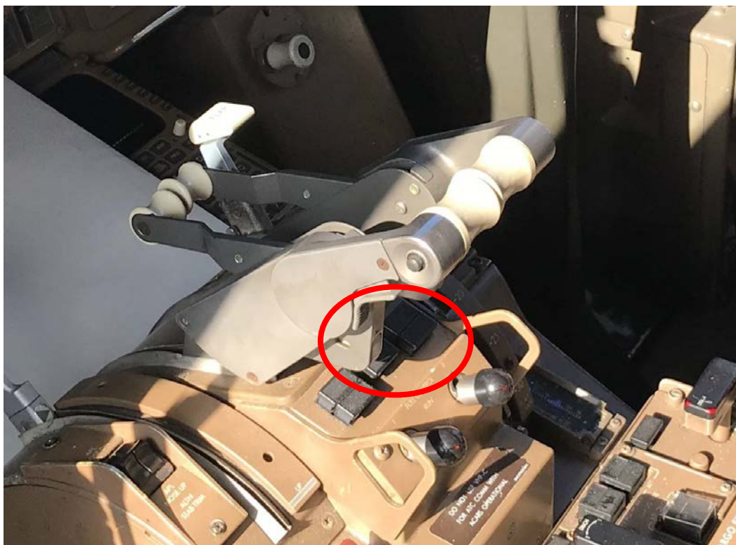
Figure 12 - 767 throttle stand, throttle levers, and Go Around switches (circled in red). Photograph is not of the accident airplane.
