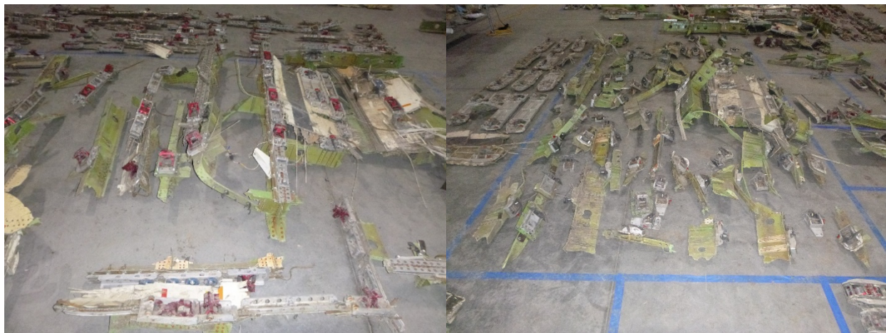
Figure 20a and b: Examples of the Cargo Loading and Securing System Components, as recovered in the Baytown warehouse.
