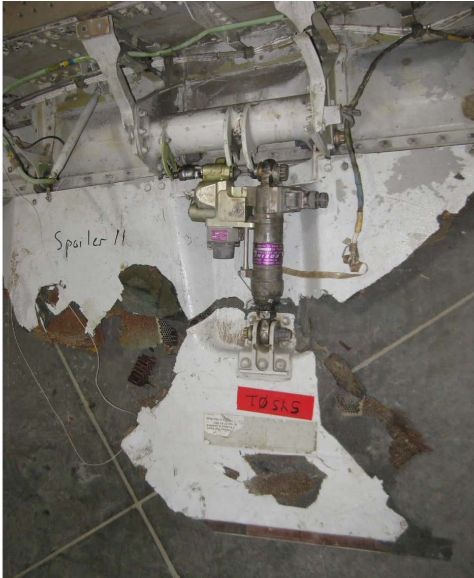
Figure 8 - Spoiler Number 11, as recovered and identified in the warehouse. Note that a portion of the spoiler flight control surface is still attached to the actuator, and the actuator is still attached to right wing structure.
