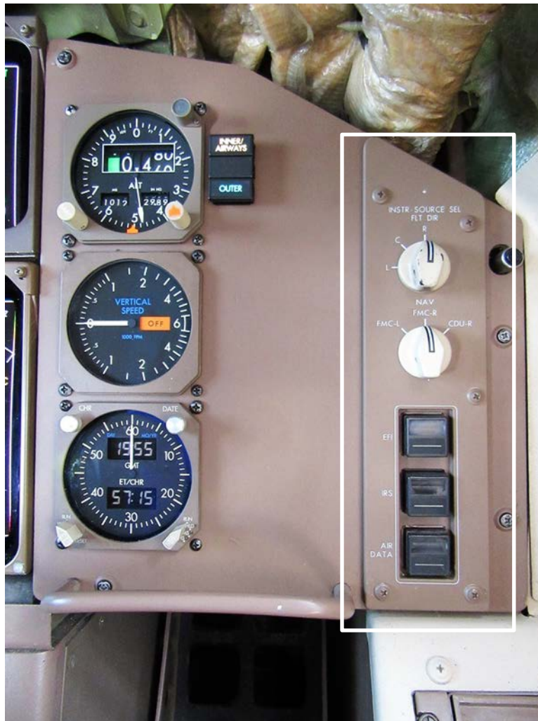
Figure 17 - The First Officer's Instrument Source Select Switch Panel, inside white box. Note: this photograph was taken during the airplane's freighter conversion in 2017.
