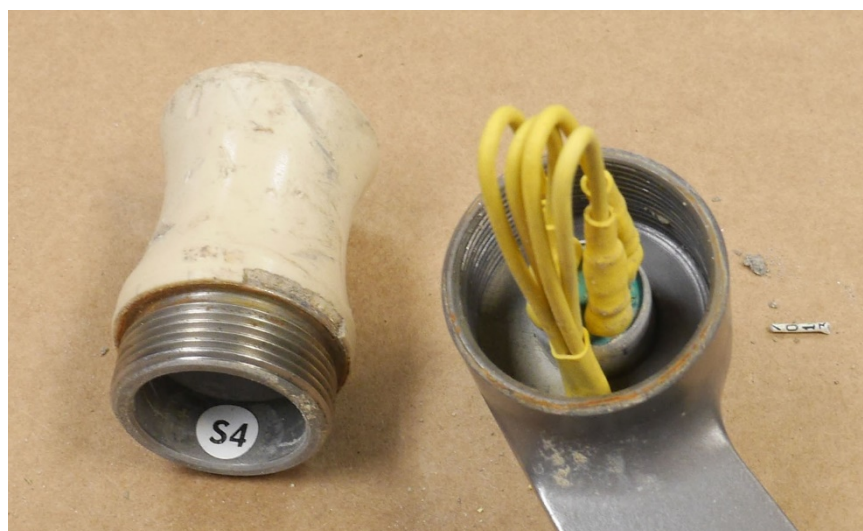
Figure 28 – Right throttle lever with knob removed for switch access
