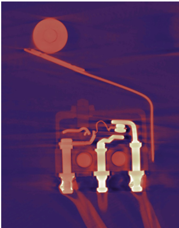
Figure 17 – CT cross section of left go-around stacked switch
