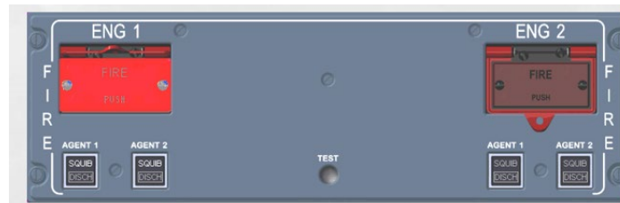
Figure 1: Engine Fire Pushbutton Located on Center Overhead Panel. (Note: ENG 1 FIRE light is illuminated)
