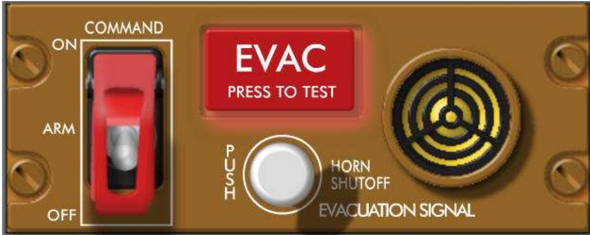
Copyright © Boeing. Reprinted with permission of The Boeing Company. Figure 2: Emergency Evacuation Command Panel 33
