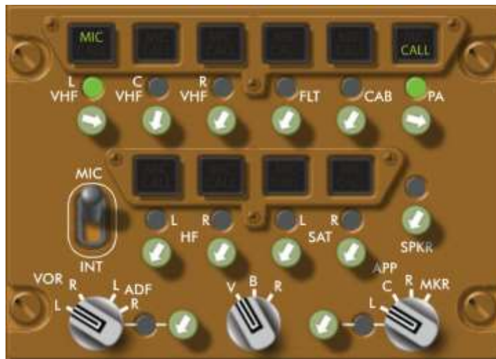
Copyright © Boeing. Reprinted with permission of The Boeing Company. Figure 1: B767 Audio Control Panel. 31
