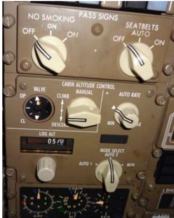
Photo 3: B-767 Pressurization Panel. 32
