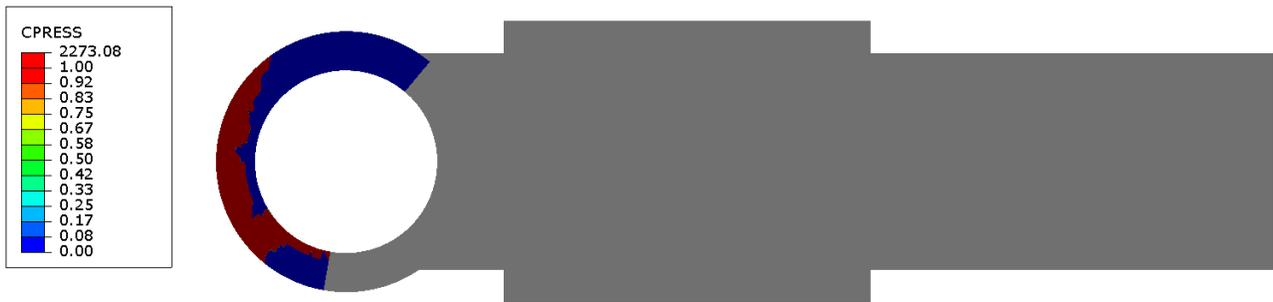
Figure 14. Contact pressure at the assumed preexisting separation at the saddle fusion interface (unit: psi).
