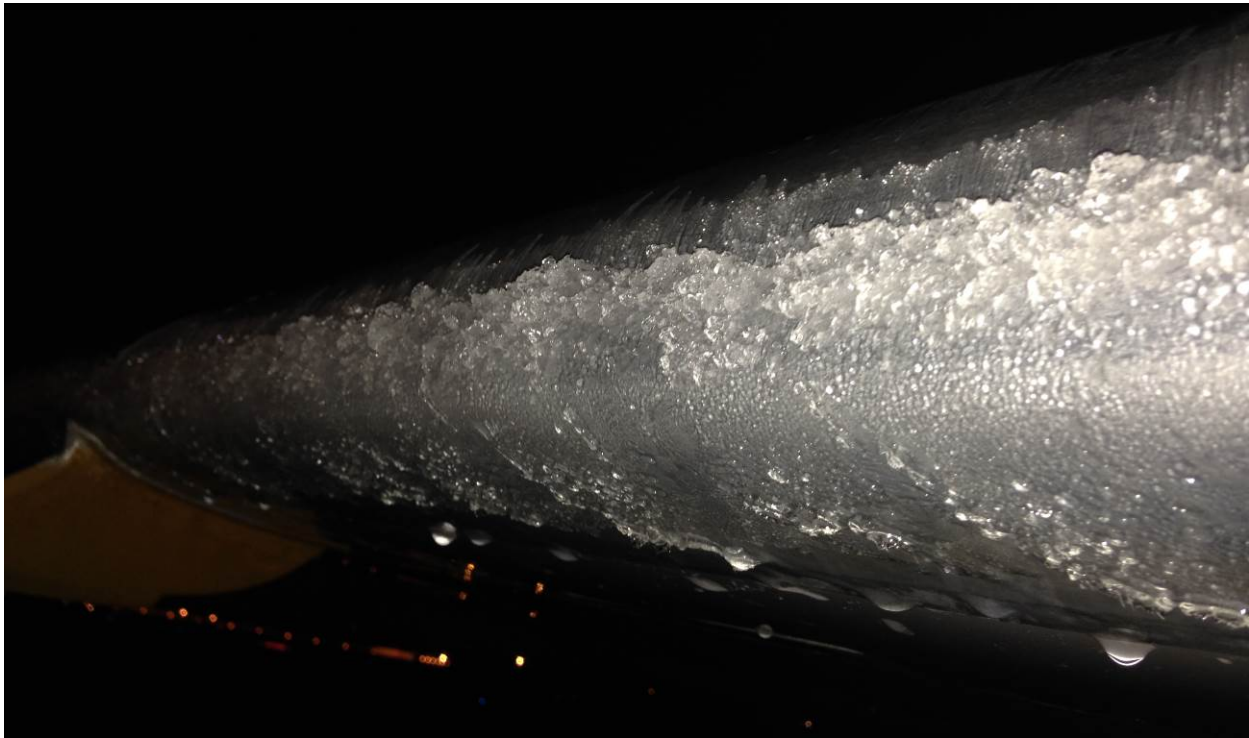
Figure 10. Ice on the leading edge of the aircraft wing shortly after landing.
