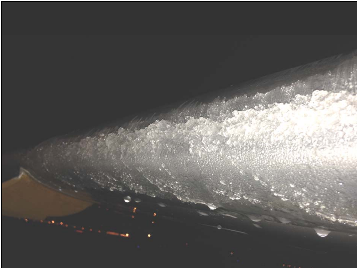
Figure 19 - Structural icing left on the wing after the airplane arrived at the gate
