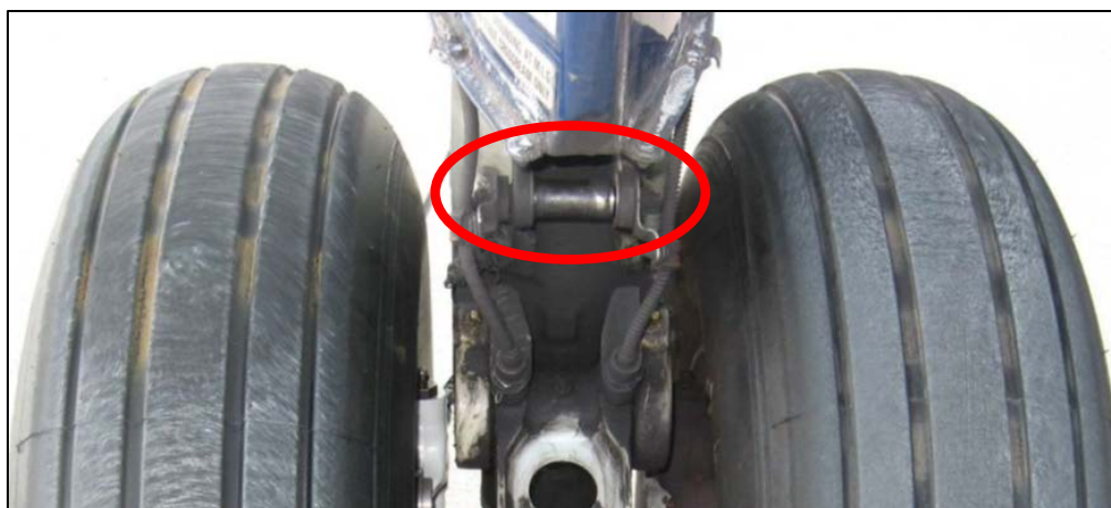
Figure 6 - Main Gear with Uplock Roller Circled in Red. Note: Airplane in figure is not the accident airplane. (Photograph Courtesy of Piedmont)
