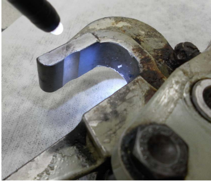
Figure 12 - Left Main Gear Uplock Latch and Groove.
