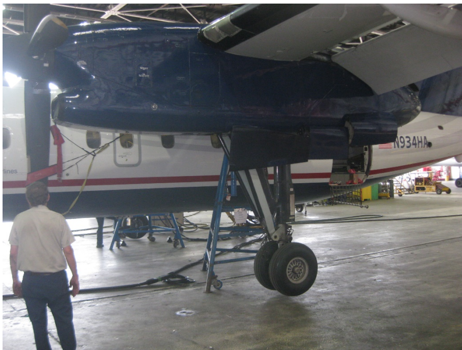
Figure 3 - The Left Main Landing Gear of the accident airplane, on jacks, after removal from the runway. The gear moves aft and up during the gear retraction sequence.
