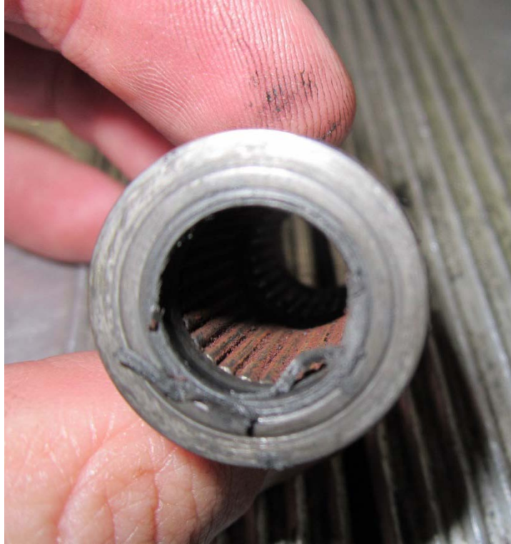
Figure 11 - The left gear uplock roller, after removal.
