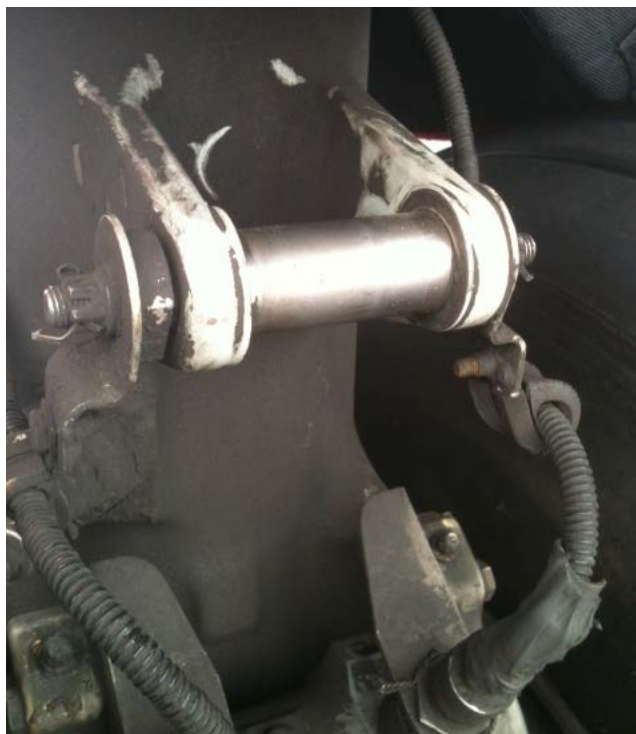
Figure 8 - Left Main Gear Uplock Roller, as installed.
