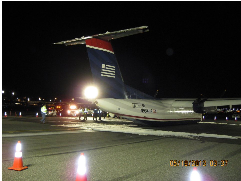
Figure 2 – Aft view of the airplane after landing without the nose or main landing gear extended. (Photograph courtesy of the FAA)
