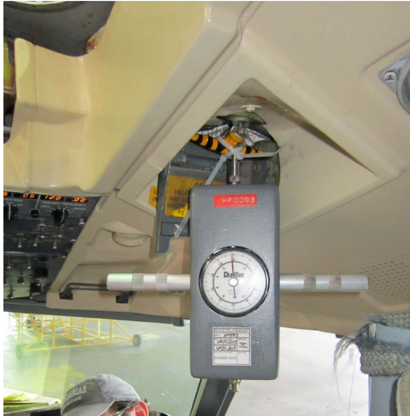
Figure 10 - The "fish scale" force gauge, as installed, connected to the Alternate Gear Release T-Handle.
