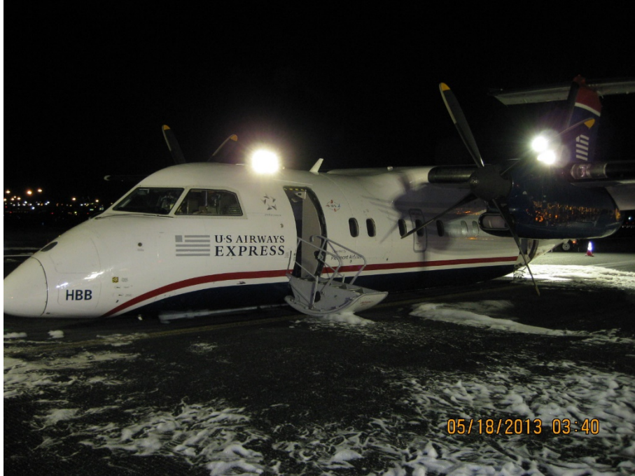
Figure 1 -The airplane after landing without the nose or main landing gears extended. (Photograph courtesy of the FAA)
