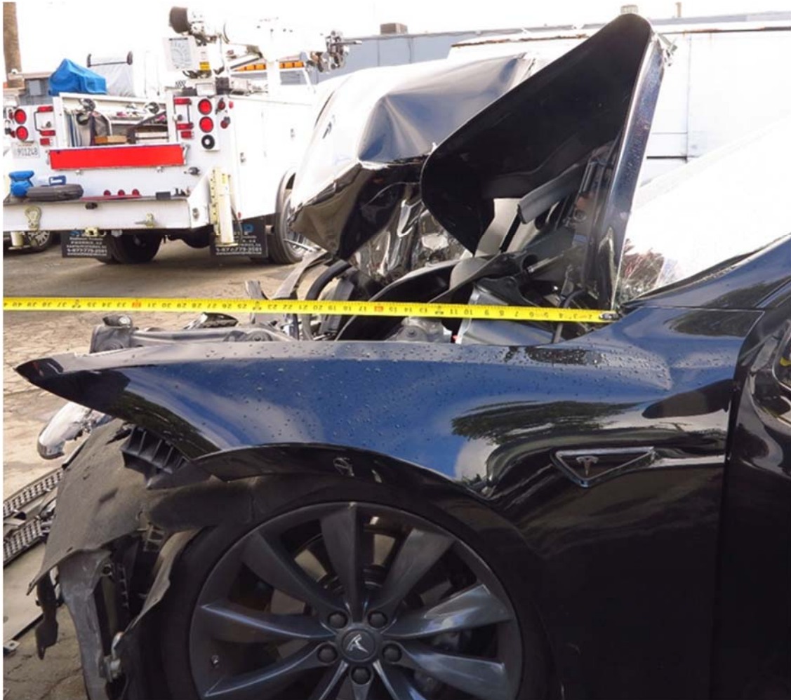
Vehicle Photo 2: This is a view of the damage sustained to the hood of the passenger vehicle.
