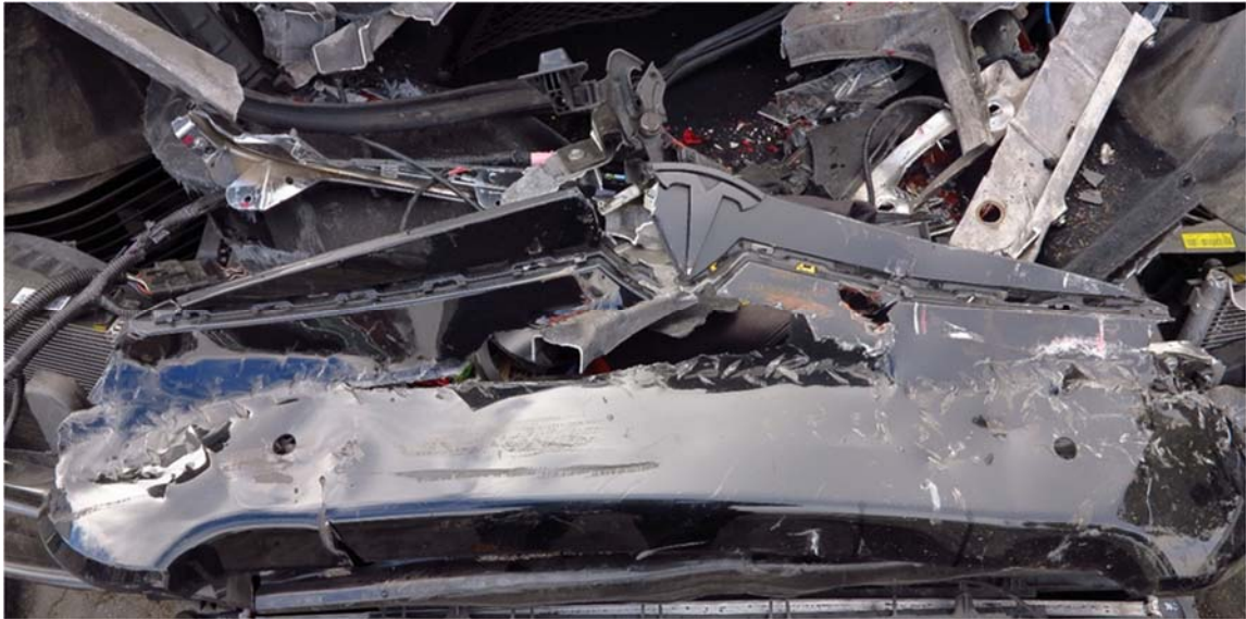
Vehicle Photo 1: This is a view of the design imprint on the upper cowling of the passenger vehicle, that was transferred from the rear of the Fire Truck.
