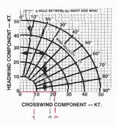
The reported wind at the time of the accident was from 080 degrees at 9 knots, gusting to 22 knots. The pilot was landing on runway 17R. The maximum demonstrated crosswind component was 19 knots.
