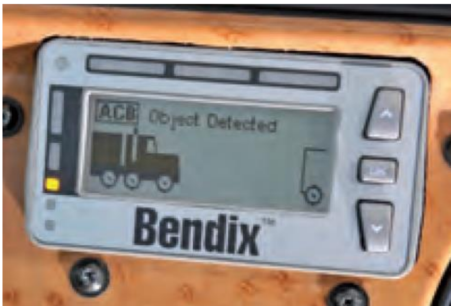
Figure 1. Bendix Wingman Advanced System Showing Object Detected (Source: Bendix Wingman Manual)
