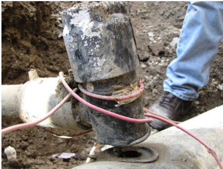
Figure 25: Separated 2-inch saddle tee from the HDPE main.
