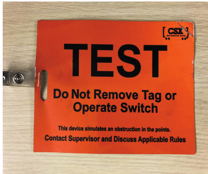
Example of simulated obstruction in the switch points.
