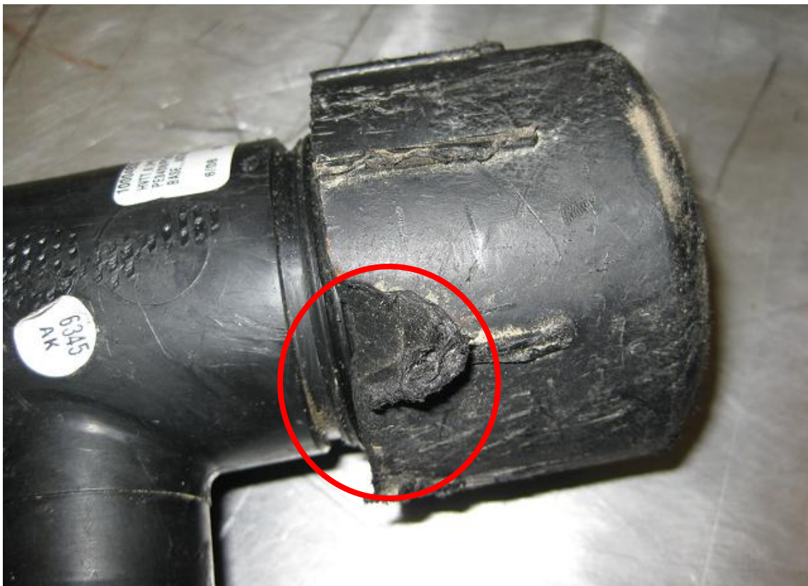
Figure 9 –Picture of damaged cap on Tee
