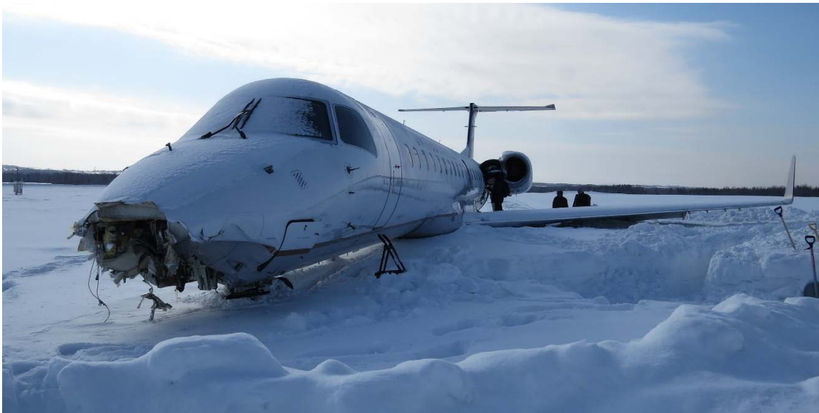
Figure 2 Aircraft nose area damage
