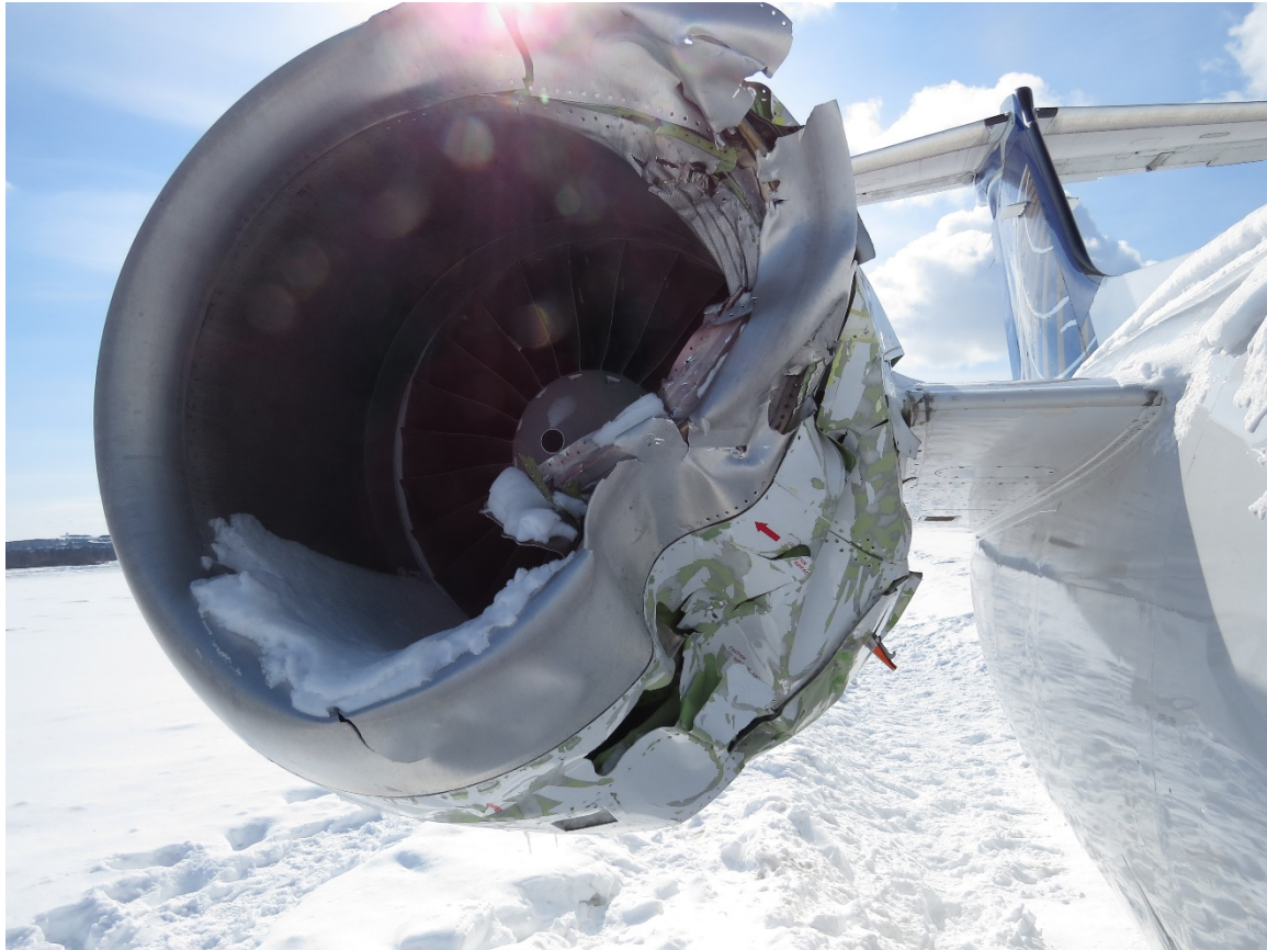
Figure 8 Right engine nacelle damage
