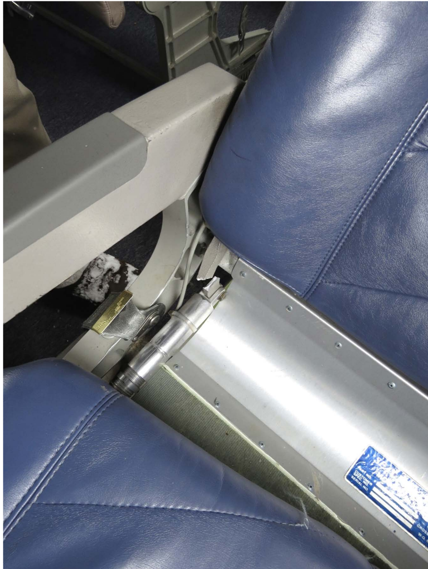
Figure 12 Broken recline actuator hinge on seat 9A
