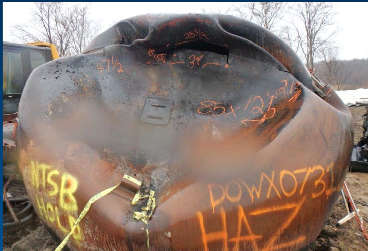
DOWX73168 cracked tank head
