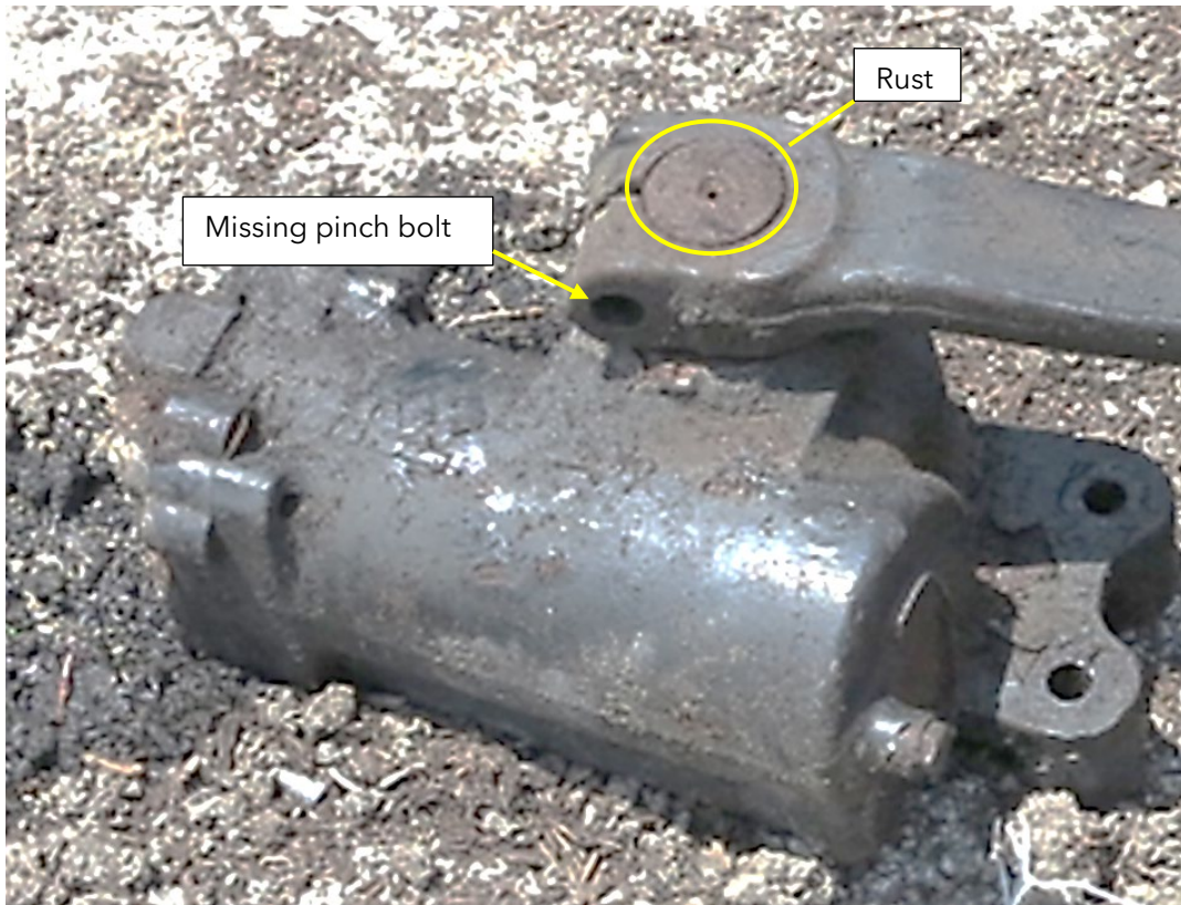
Figure 3: Photograph of the steering gear box, sector shaft, and pitman arm
