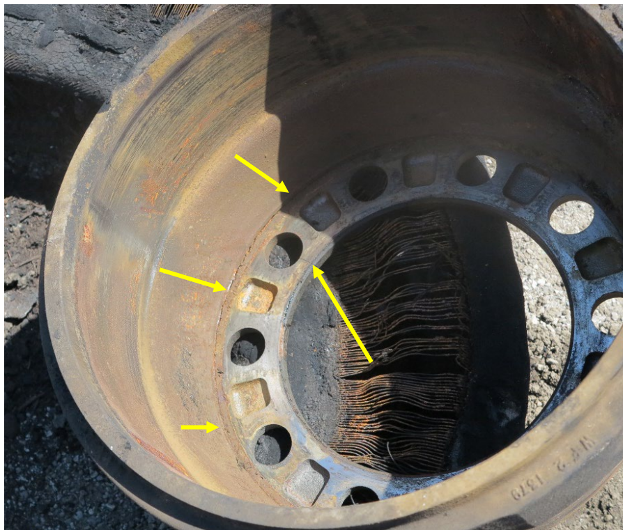
Figure 6: Photograph of the cracked left-side brake drum
