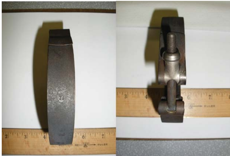
Figure 24 Spot-welded, 3-segment, Coupling
