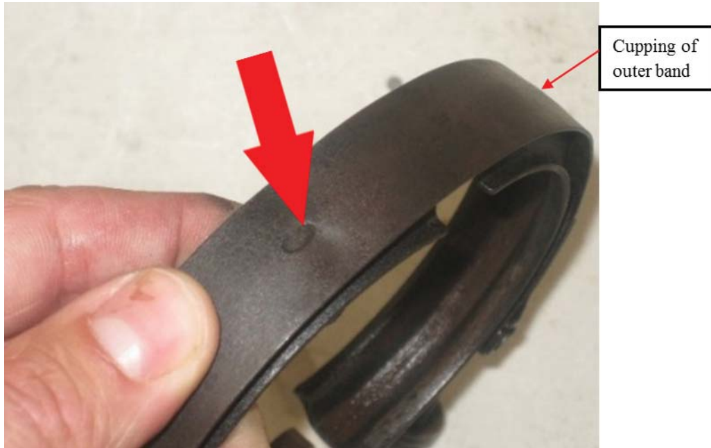
Figure 22 Spot-welded, 3-segment Coupling
