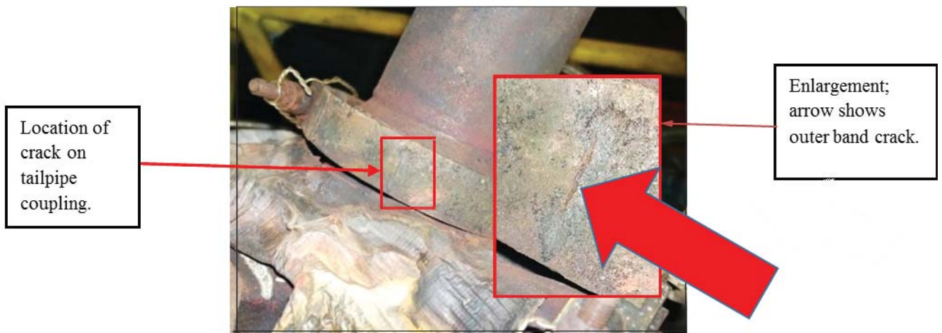
Figure 21 Spot-welded, Multi-segment Coupling
