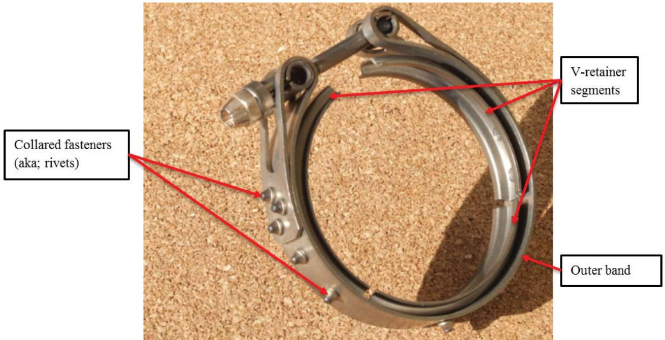
Figure 6 Riveted (aka, Collared Fastener), Multi-Segment, V-band Coupling, 3-Segment, Unknown size
