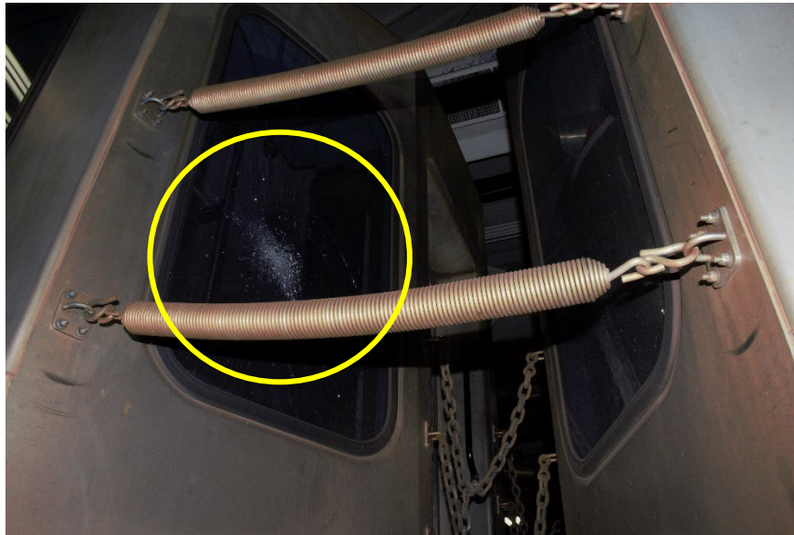
Figure 9 Photograph taken from the exterior of Train Car 5600 showing the smashed right front window, highlighted in yellow, caused by the impact with an occupant inside of the train car. (Source: NTSB)
