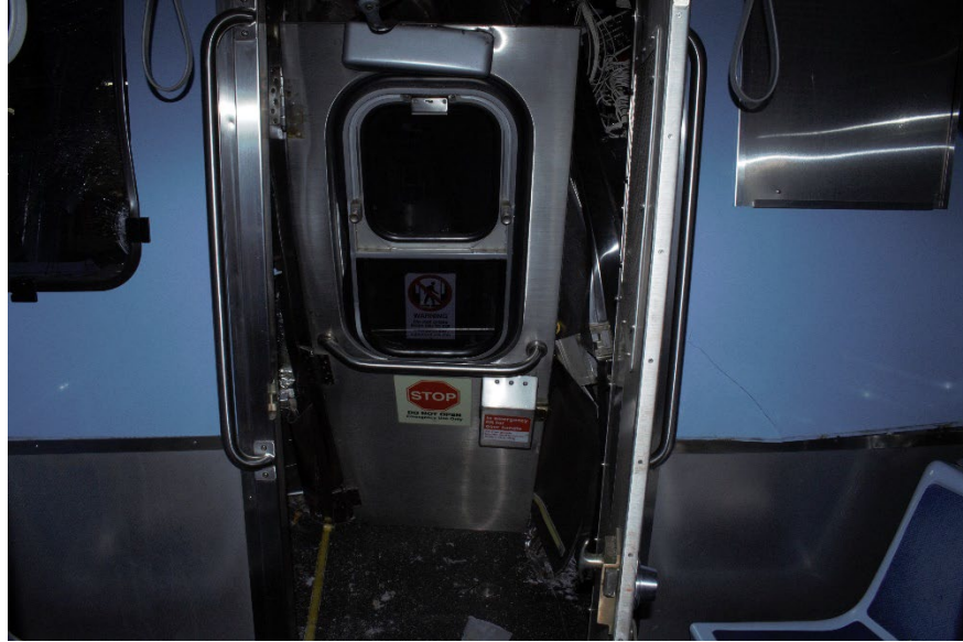
Figure 8 Photograph of the end car door of Train Car 5599 that was shoved inward into the operator's compartment space during the collision. The operator's compartment door that swung open and into the passenger compartment following the impact with the snowplow is visible in the foreground. (Source: NTSB)
