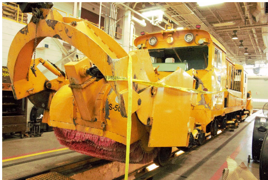
Figure 11 Photograph taken at the Skokie maintenance shop of the Snow Removal Vehicle S-500 with the area of impact with the train, the brush assembly, in the foreground and the windshield of the cab where the employee was ejected, in the background. (Source: NTSB)
