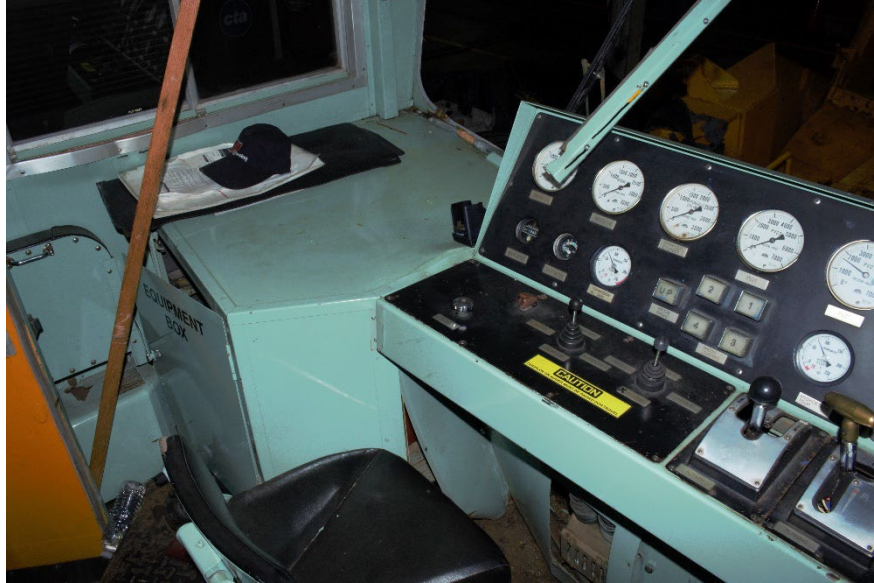
Figure 10 Photograph of the interior cab of the snow removal vehicle at End No. 2 showing the equipment box that the employee was thrown across before being ejected out of the windshield. (Source: NTSB)
