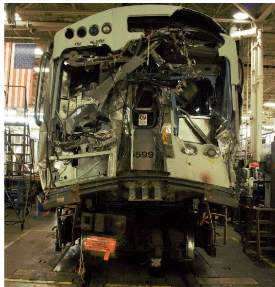
Figure 7 Photograph taken looking at the lead train car, 5599, that struck the snow removal vehicle and shows the resulting collision damage. (Source: NTSB)
