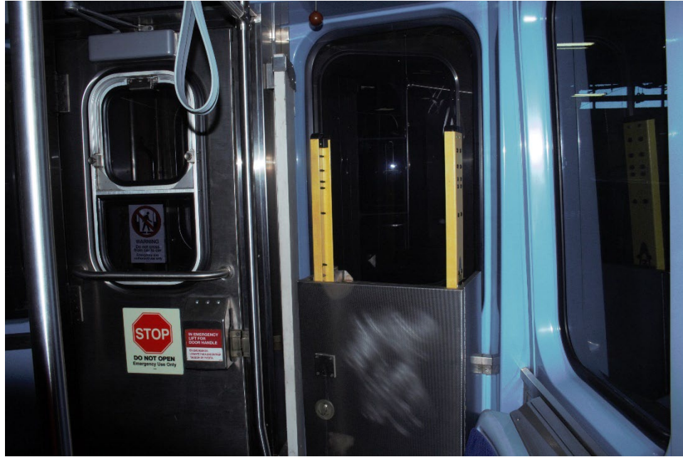
Figure 18 Photograph showing the emergency evacuation ladder in the stowed position on an exemplar "A" car. (Source: NTSB)
