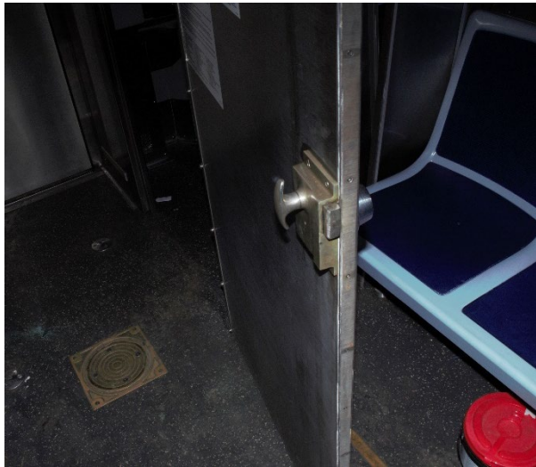
Figure 14 and 15 Photographs of Train Car 5600 operator's compartment door latching mechanism and the frame catch that sprung open during the accident. (Source: NTSB)
