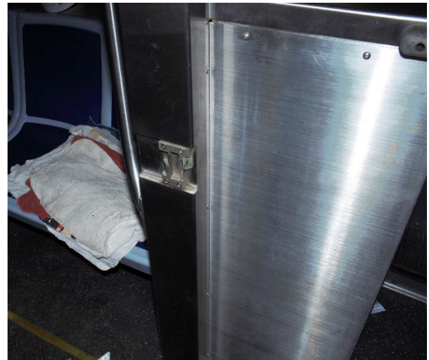
Figure 14 and 15 Photographs of Train Car 5600 operator's compartment door latching mechanism and the frame catch that sprung open during the accident. (Source: NTSB)
