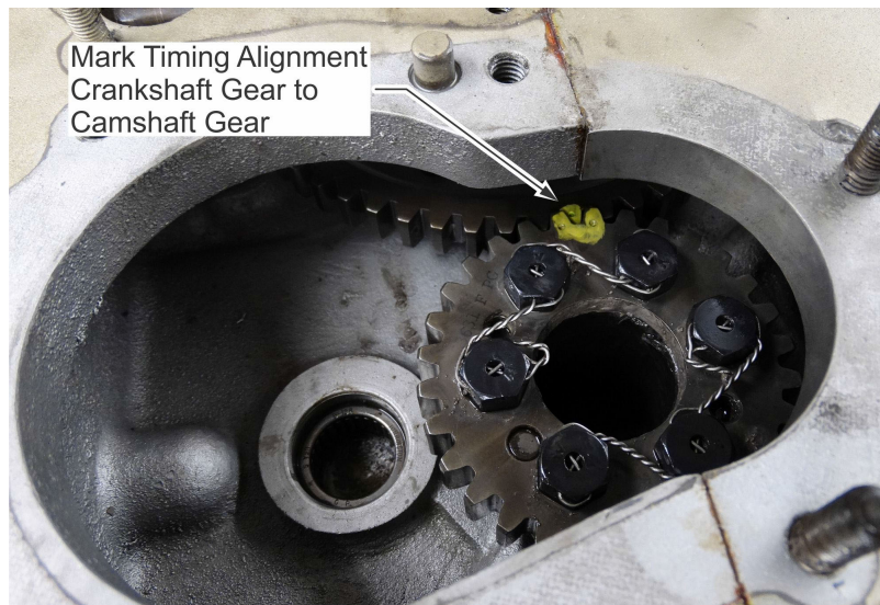
Figure 15. Camshaft Gear Timing Alignment Marked, Sandcast Crankcase
