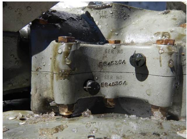
B- Hartzell three blade full feathering propeller model: PHC-C3YF-2UF, hub serial number EB4536A
