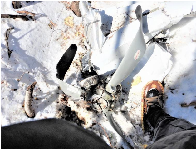
A-Hartzell three blade full feathering propeller model: PHC-C3YF-2UF, hub serial number EB4535A
