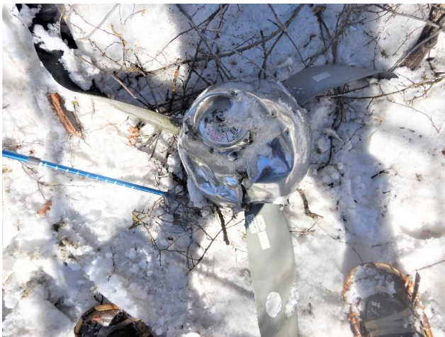
B- Hartzell three blade full feathering propeller model: PHC-C3YF-2UF, hub serial number EB4536A
