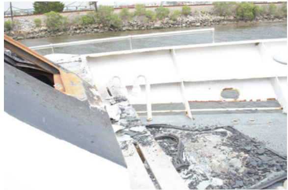
Bow and Damage from Failing Window
