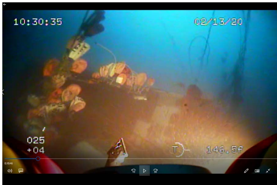
Figure 8: Crab pots, a tethered life ring and random lines extend upward from SCANDIES ROSE to within 40' of the surface
