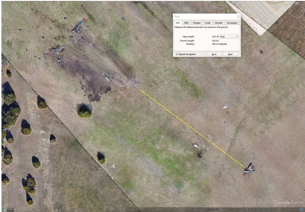
Figure 9. The B-17G initial impact point was located about 410 ft northwest of the tail (Google Earth Overlay).
