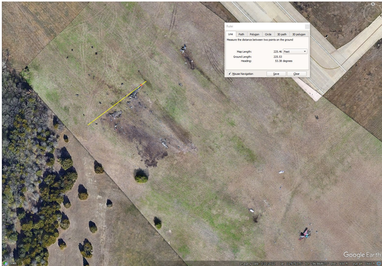
Figure 12. The main B-17G debris field measured about 525 ft long by about 225 ft wide (Google Earth Overlay).
