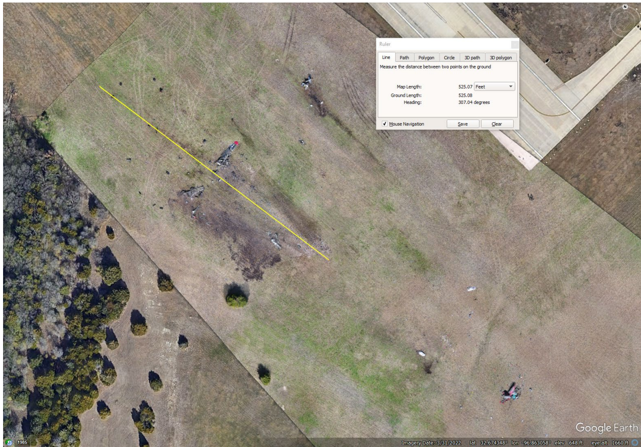
Figure 11. The main B-17G debris field measured about 525 ft long by about 225 ft wide (Google Earth Overlay).
