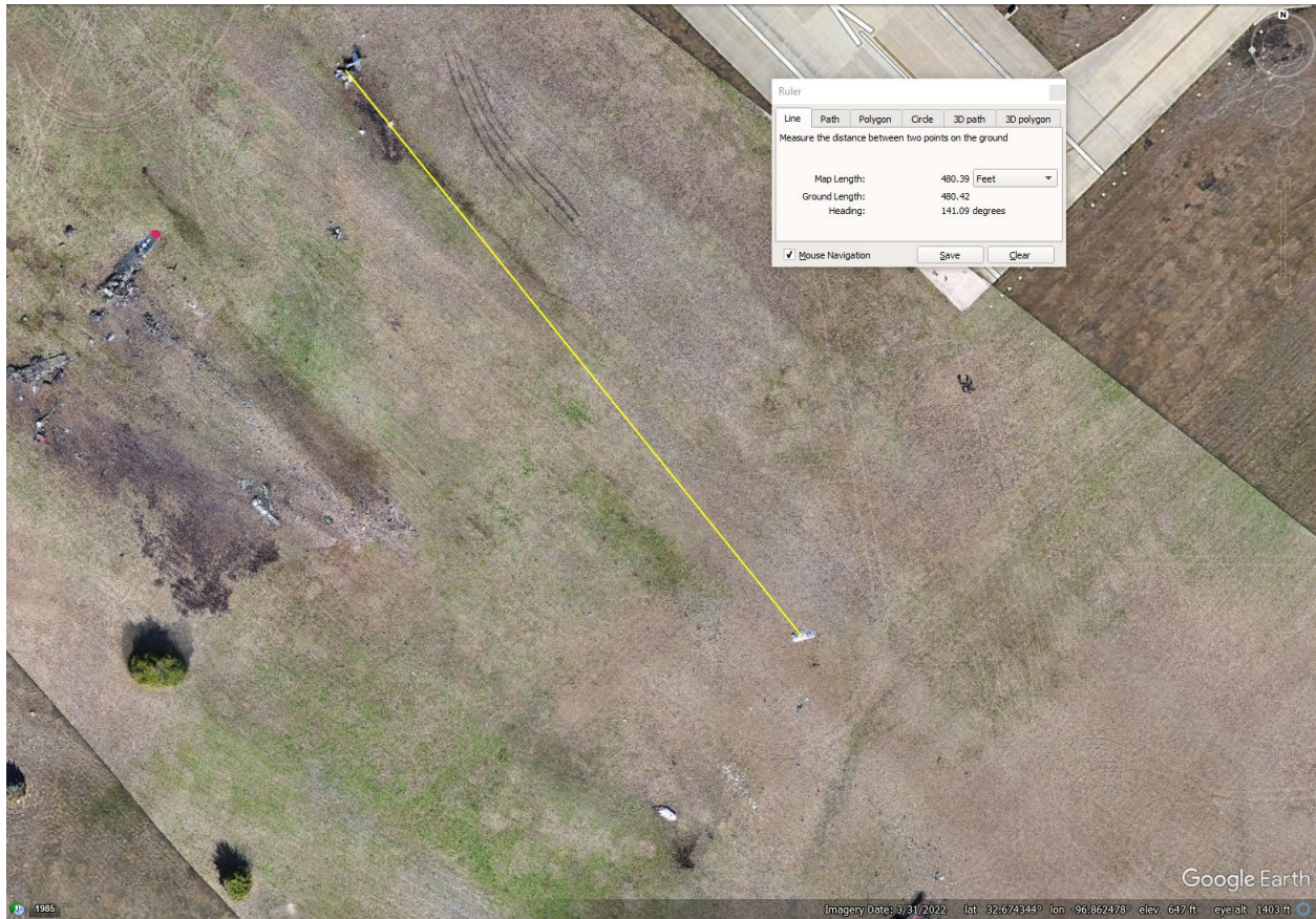
Figure 14. The P-63F left and right wings separated from the fuselage during the collision and were located in the debris field. The right wing was lying on its upper surface and was located about 480 ft southeast of the P-63F fuselage (Google Earth Overlay).
