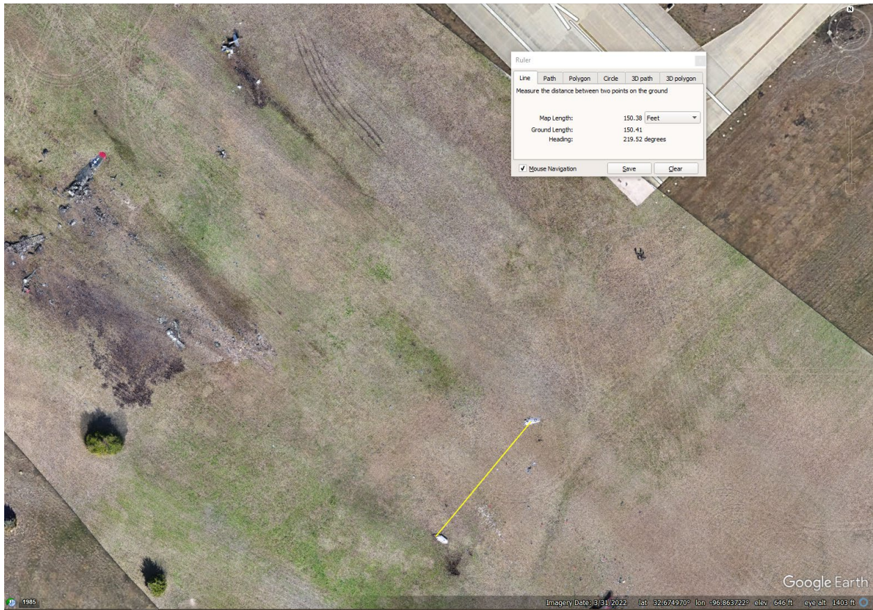
Figure 16. The P-63F left and right wings were separated by about 150 ft (Google Earth Overlay).
