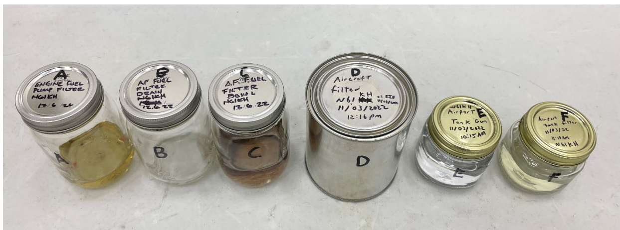
Figure 6. Photo of the fuel samples that were retained with the engine. (Source: Rolls-Royce)
