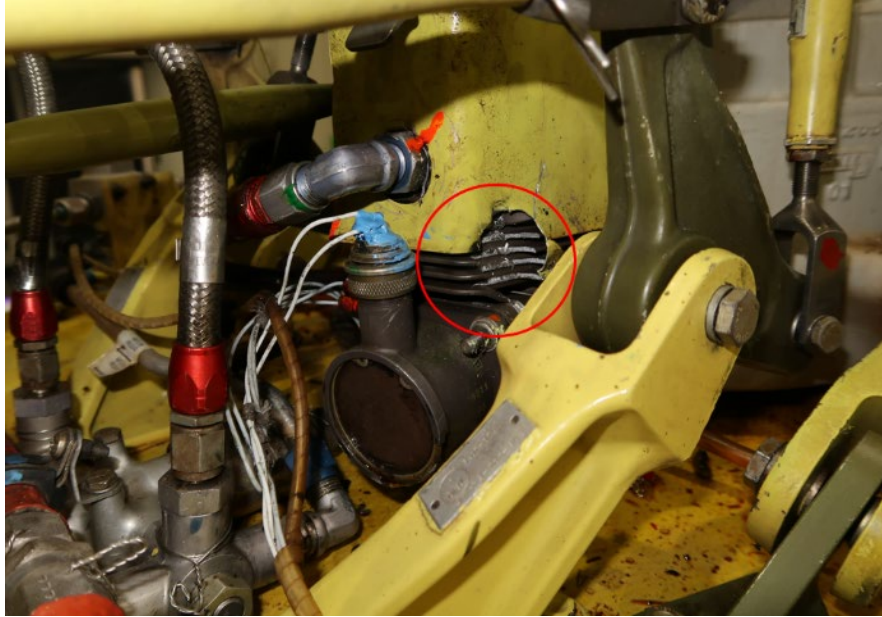
Figure 4. Hydraulic reservoir damage shown in the red circle.
