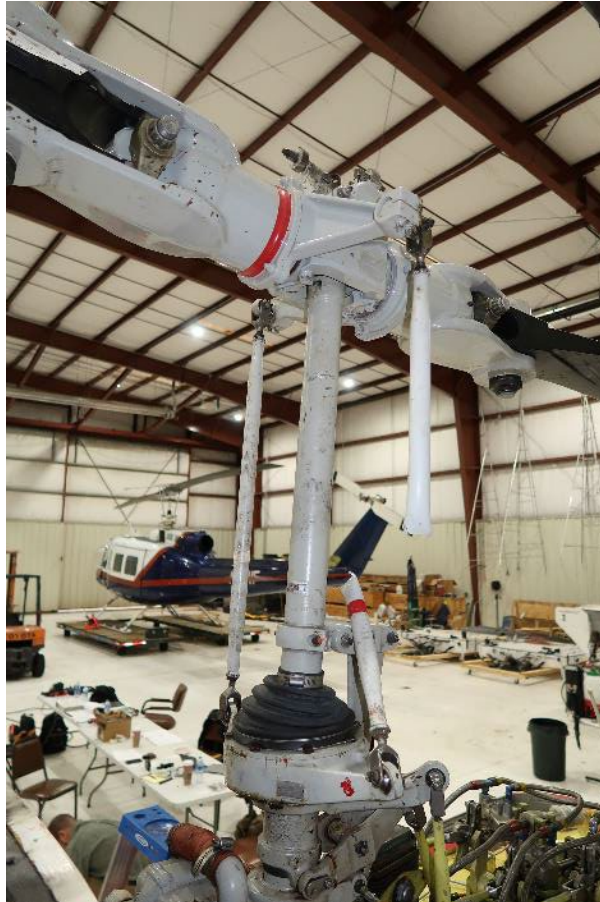
Figure 3. Main rotor head showing the fractured red pitch change link.
