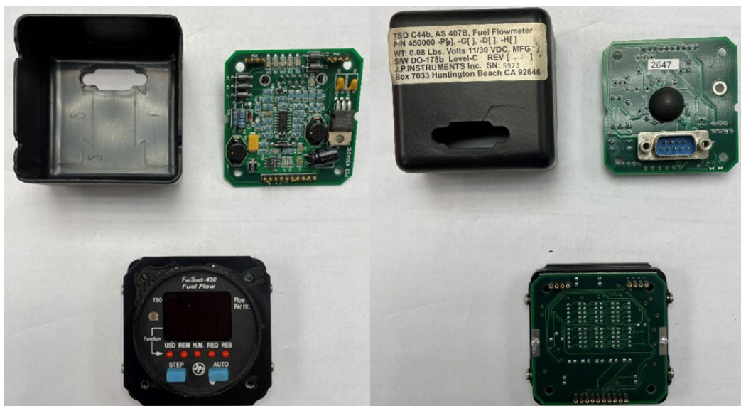
Figure 2. Front and back of the JPI FS-450 components as received.
