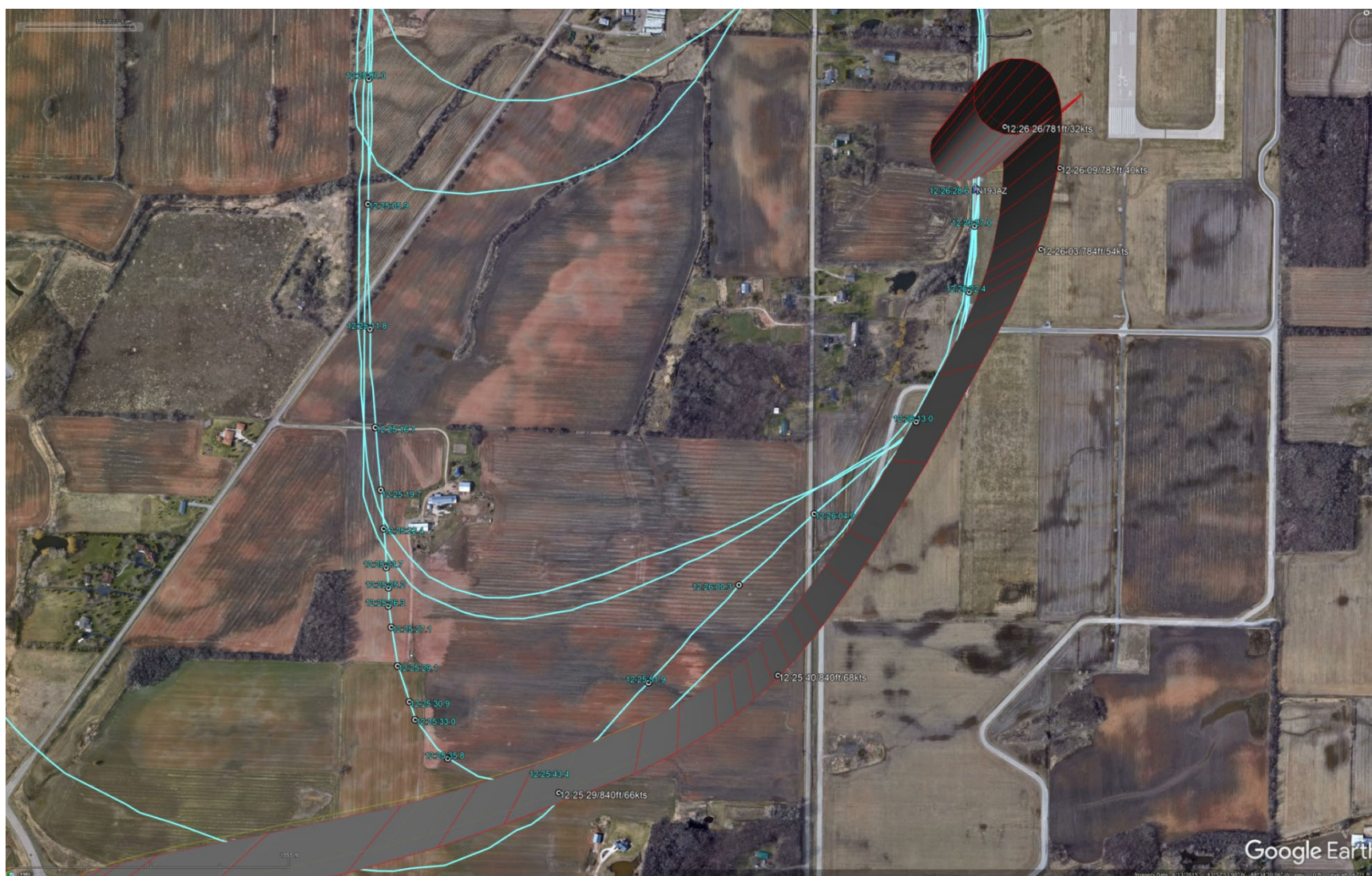
Figure 5. Google Earth overlay of the end of the accident flight that includes available GPS data from N193AZ shown in cyan.
