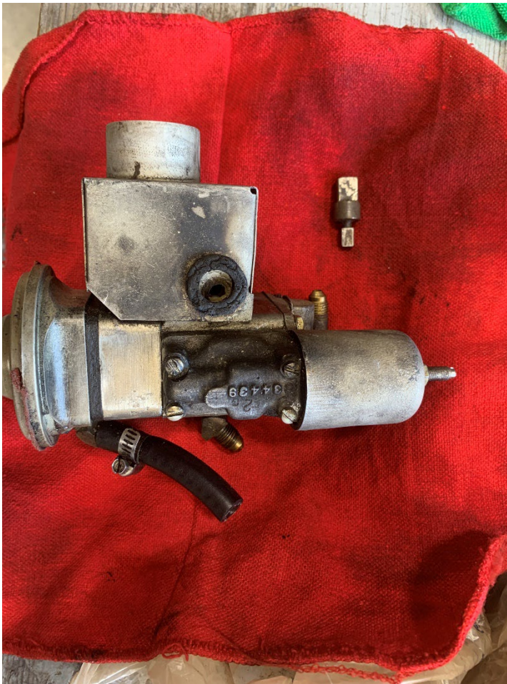
Figure 4 Fuel Pump (NTSB Photo)
