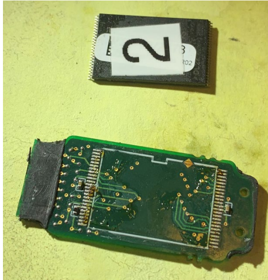
Figure 3. The Appareo Vision 1000 memory board after removal of one TSOP FLASH chip.
