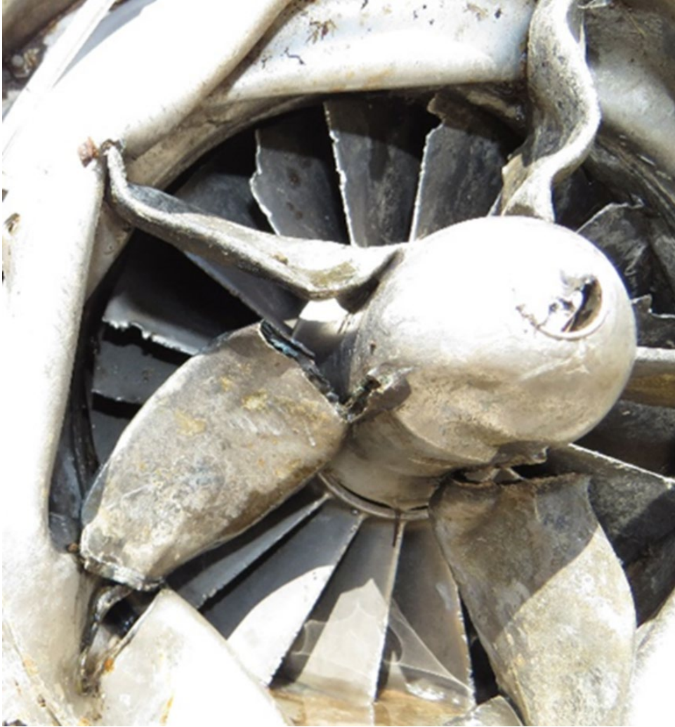
Figure 8. Inlet section of the engine exhibiting crushed inlet guide vanes.
