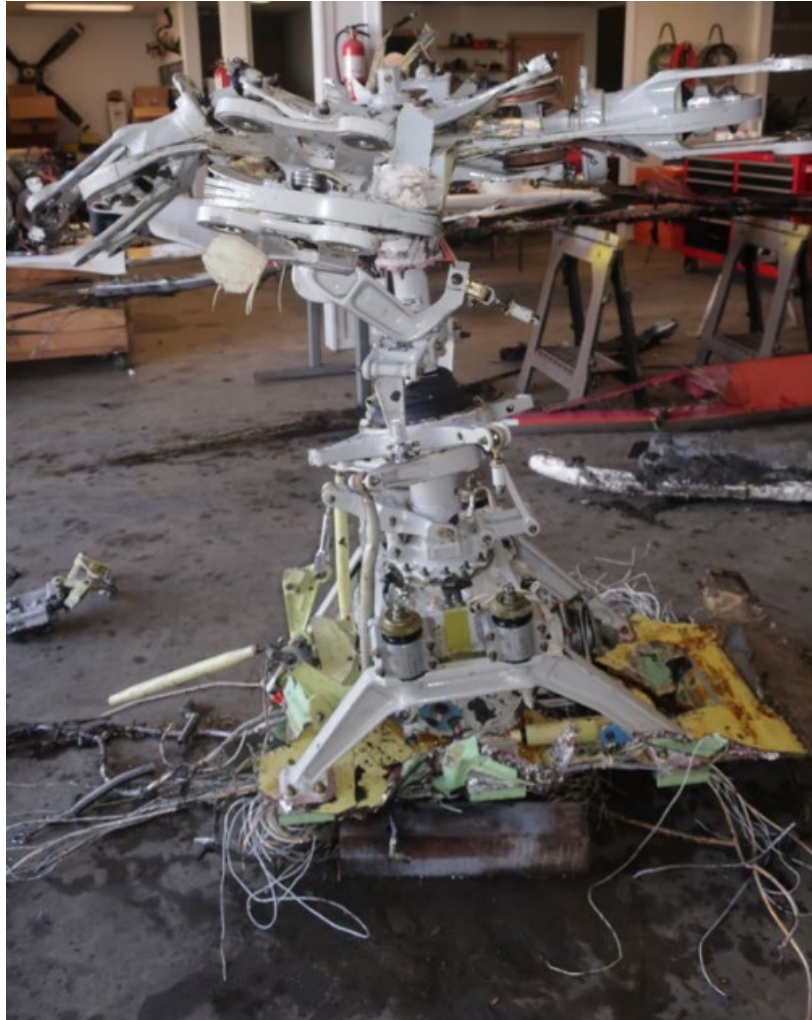
Figure 3. Transmission, transmission mount, mast, and main rotor head.
