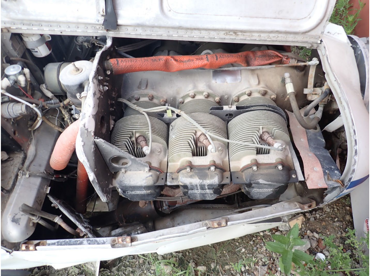
Figure 2: Engine condition as found. Note the corrosion on the exterior surface of the spark plugs.
