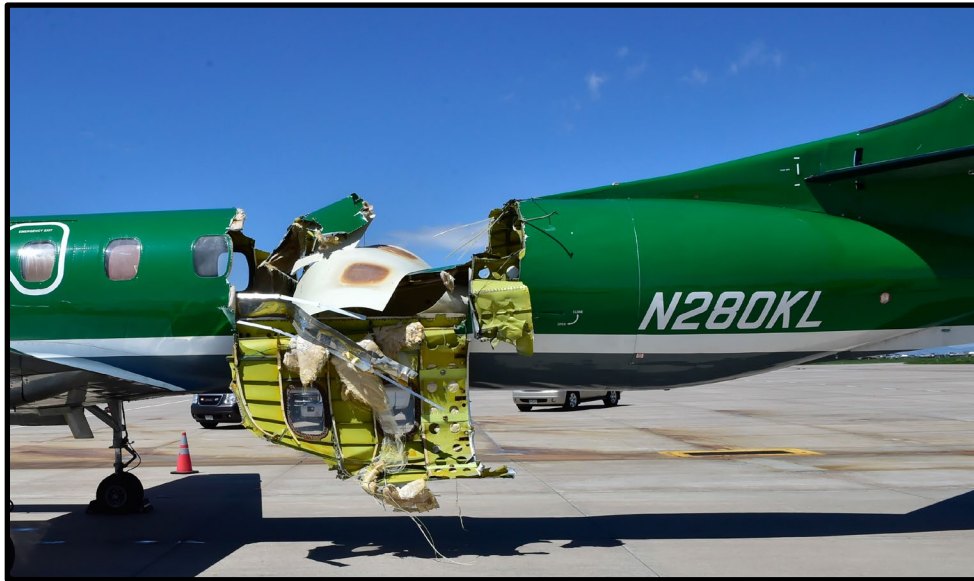
Figure 3-SA226-TC left fuselage damage.
