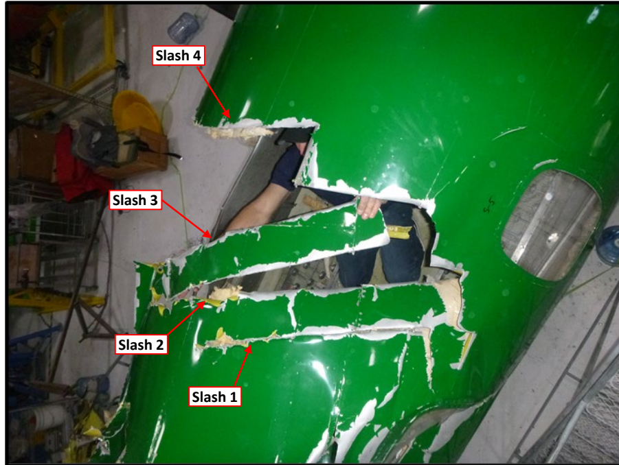
Figure 1-SA226-TC parallel slash marks in upper fuselage.
