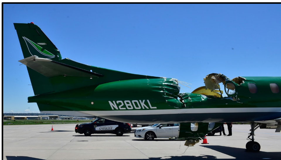
Figure 2-SA226-TC right fuselage damage.
