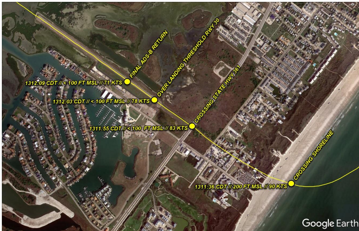
Figure 4: Radar ground track of N587CD's accident flight approach to KRAS runway 30 on April 24, 2021. 11
