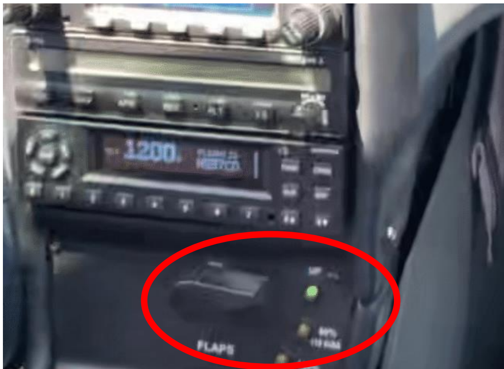
Photo 5: Enlargement of previous photo showing the flap selector switch consistent with the flaps up position, and the UP (0%) green light illuminated.
