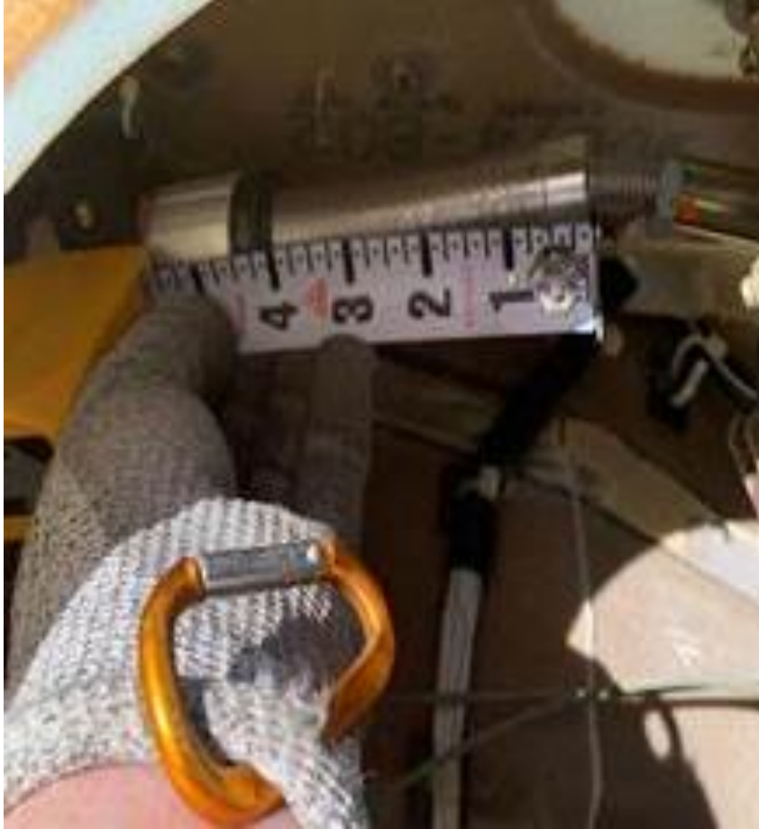
Photo 3: April 25, 2021 photo of N587CD flap actuator extended 4.5 inches, consistent with Flaps Up (0%). 34
