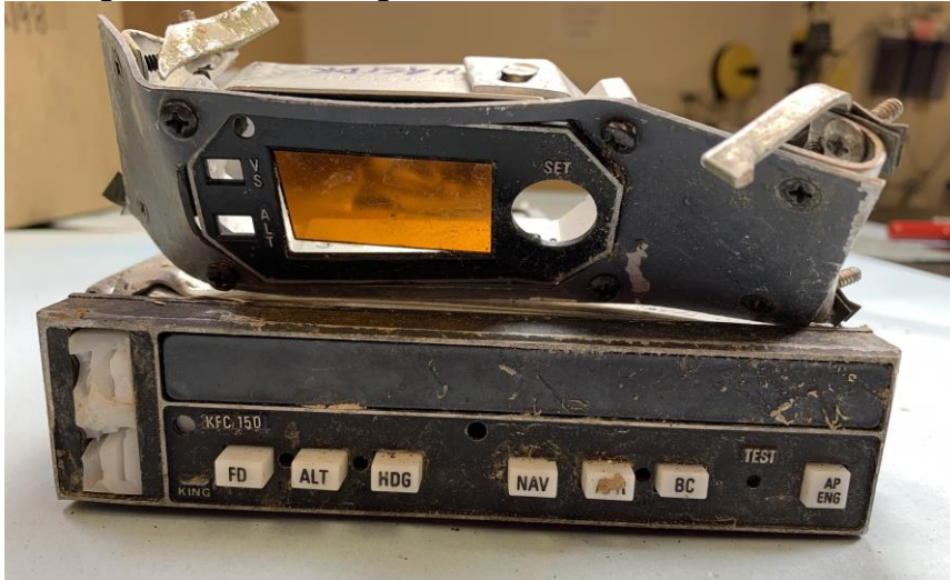
Figure 4. Exterior of the KFC-150, as received.
