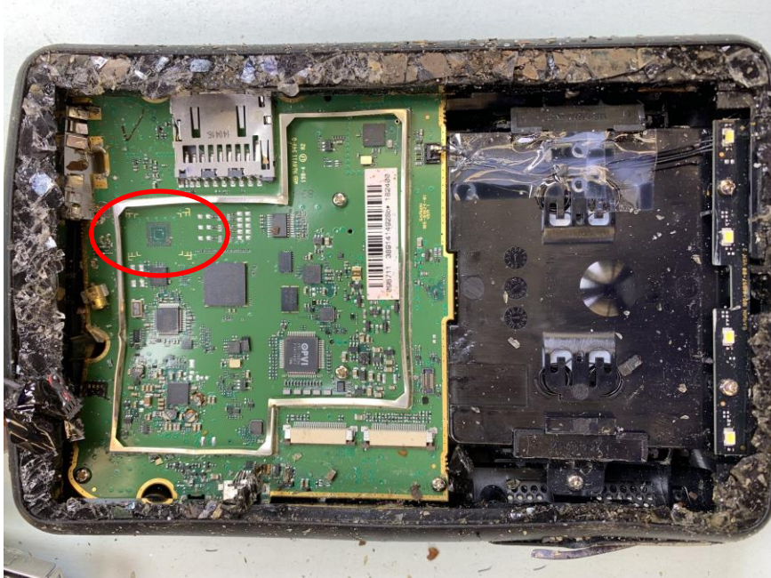
Figure 1. The internal components of the device, with the location of the memory chip mounting highlighted in red.
