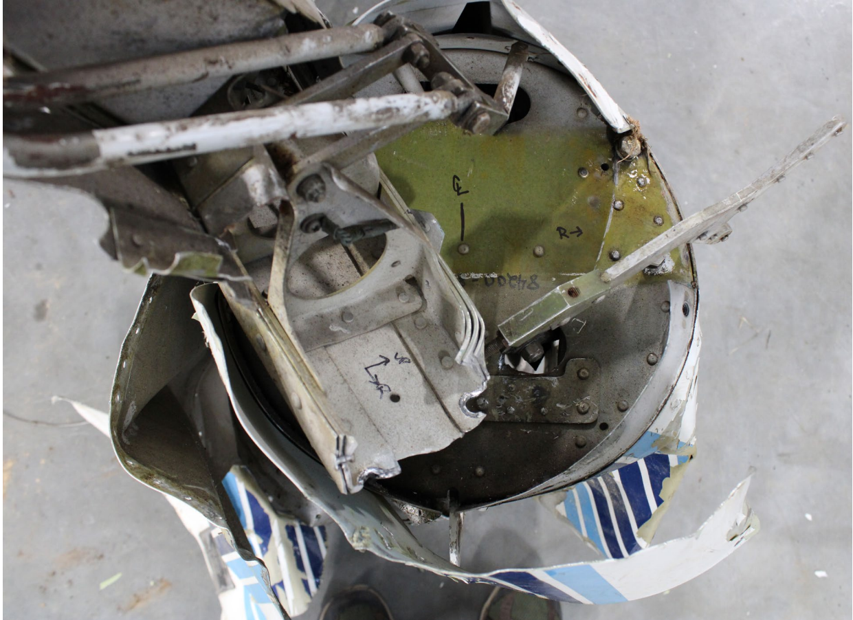
Figure 5 - Horizontal stabilizer attach point (looking forward)
