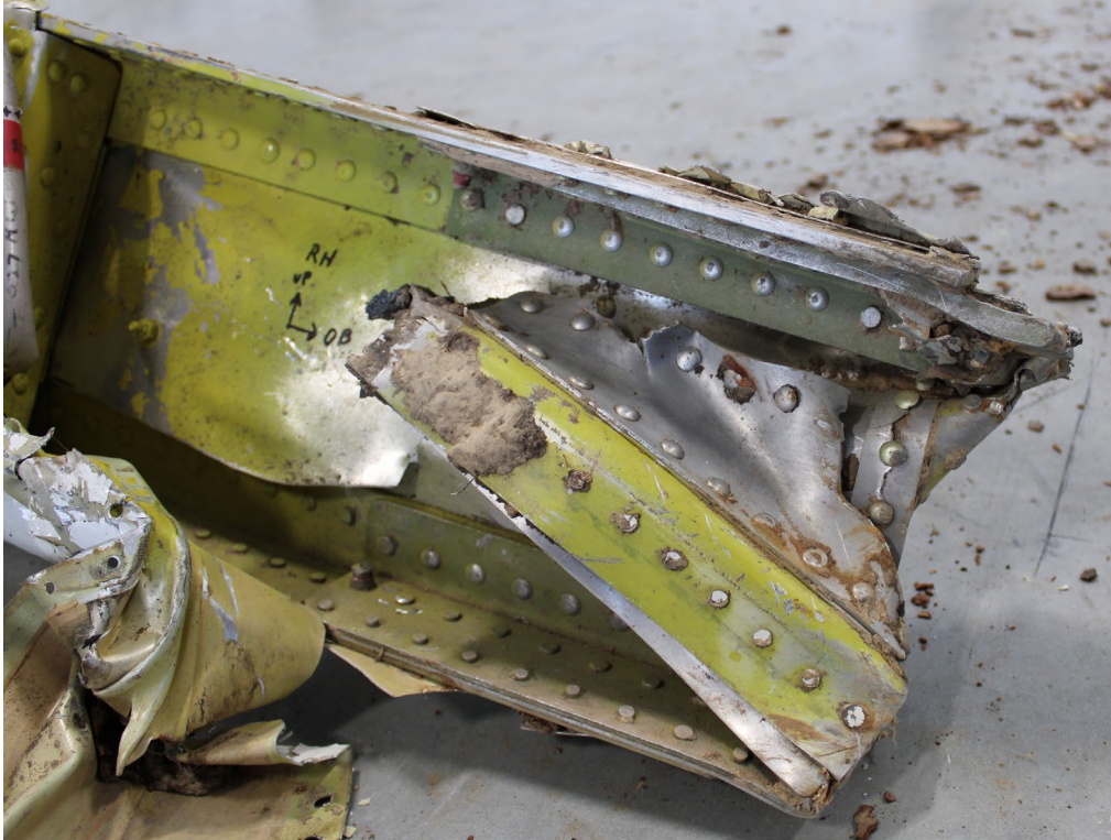
Figure 3 - Right wing forward spar separation location (looking forward)
