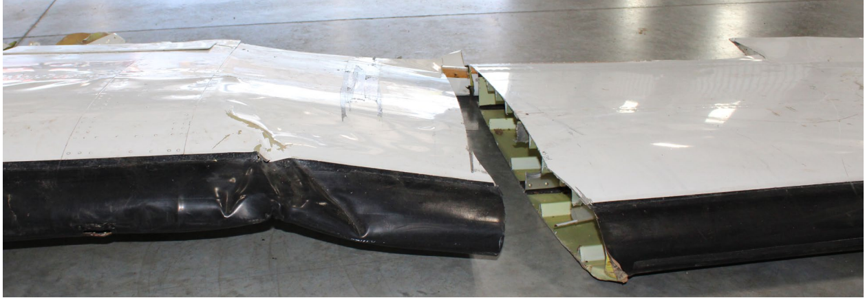
Figure 2 - Left wing downward deformation near WS 118 and cut near WS 134
