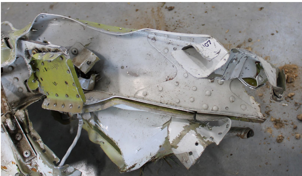
Figure 4 - Right wing aft spar separation location (looking forward)
